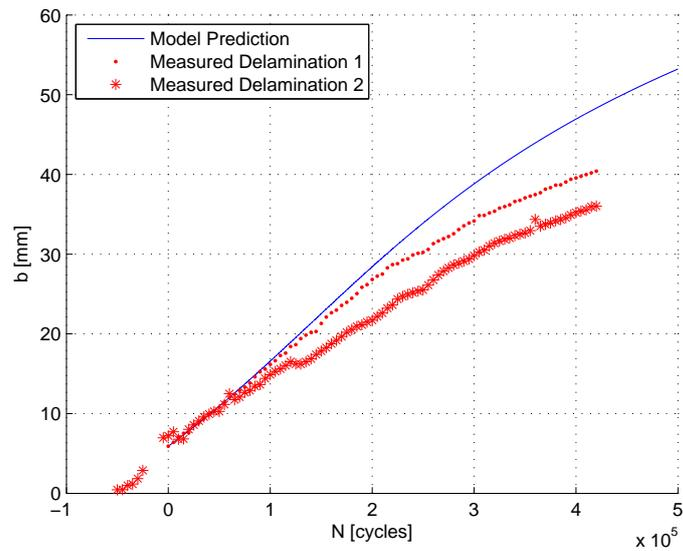
**Figure 7.4:** Delamination growth prediction for specimen A1 based on  $\Delta\sqrt{G_{II}}$ .
