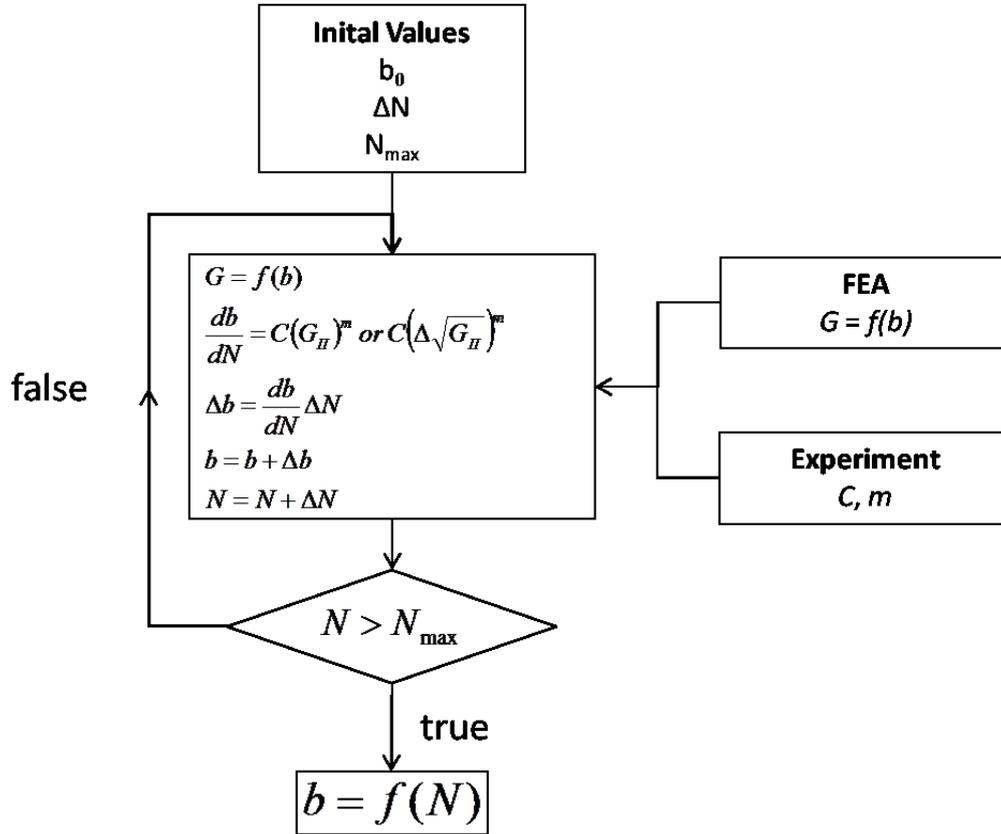
**Figure 7.1:** Flowchart depicting the numerical algorithm used to predict delamination length as a function of cycle count.
