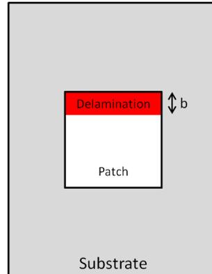
**Figure 5.19:** Delamination length definition used for the numerical analysis of the patch repair specimens.
