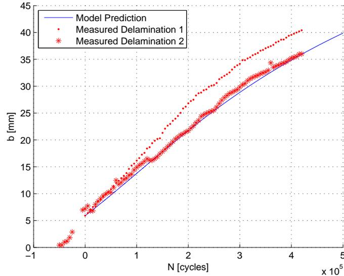
**Figure 7.2:** Delamination growth prediction for specimen A1 based on  $G_{tot,max}$ .
