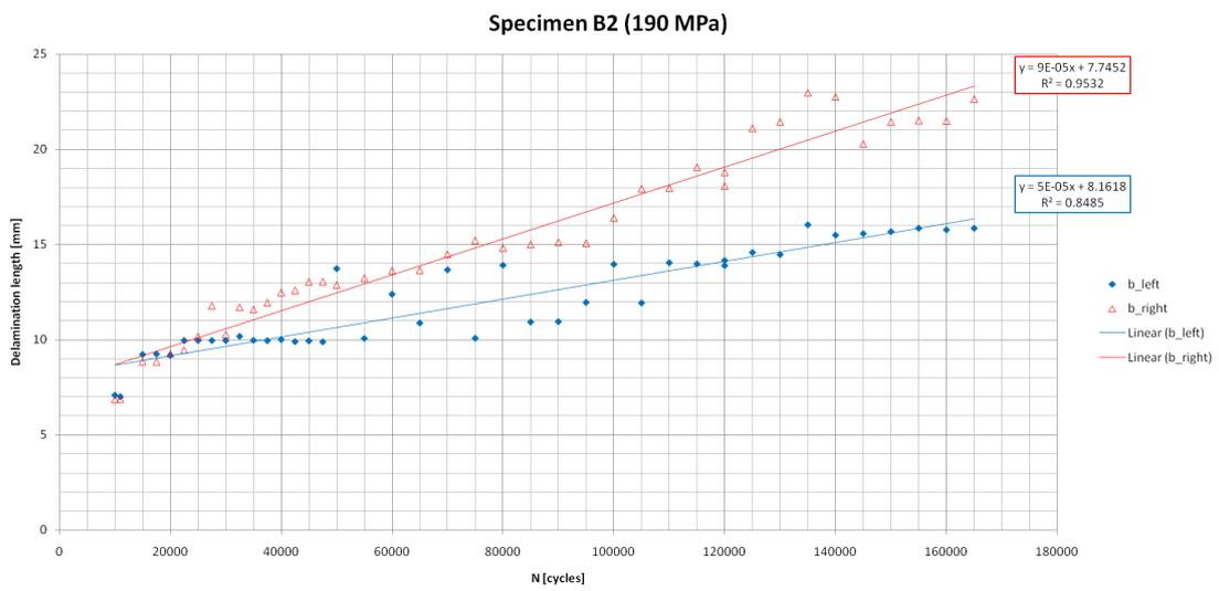
Figure A.5: Delamination lengths measured for specimen B2.
