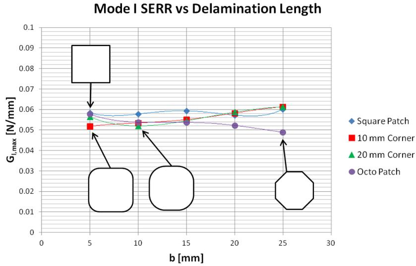
**Figure 5.24:** Mode I SERR vs delamination length for the patch repair specimens, including 4th order polynomial trendlines.
