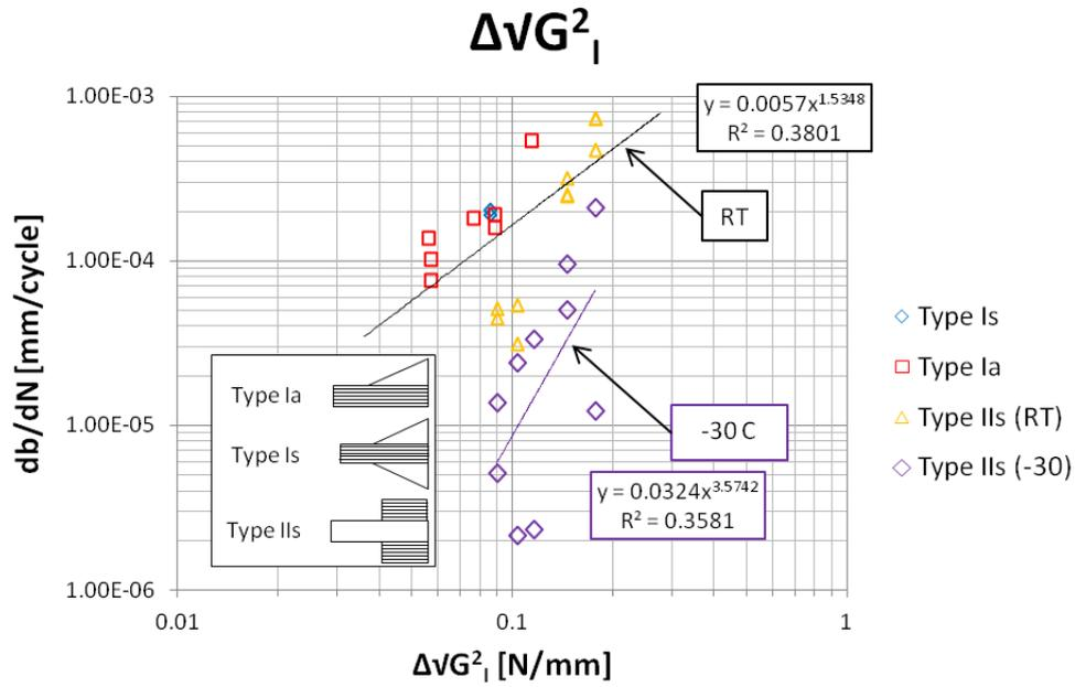
Figure 6.12: Delamination growth rate plotted as a function of mode I SERR range. Power-law curve fits are shown both for the specimens tested at room temperature and for the specimens tested at  $-30^\circ C$ .
