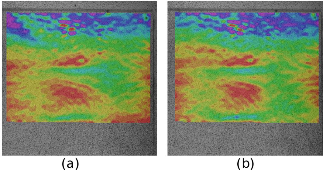
**Figure 6.18:** Comparison between two DIC measured strain fields after 55 kcycles. Image (a) was taken at the end of one test day. Image (b) was taken at the start of the next day. As no fatigue loading occurred in the meantime and the specimen was kept at room temperature in lab air, the two measured strain fields should be the same. However due to the noise in the DIC system they are not.
