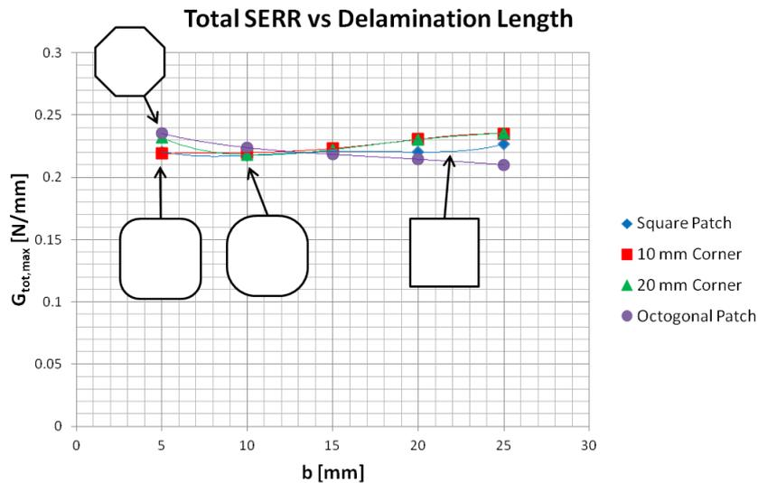
**Figure 5.23:** Total SERR vs delamination length for the patch repair specimens, including 4th order polynomial trendlines.
