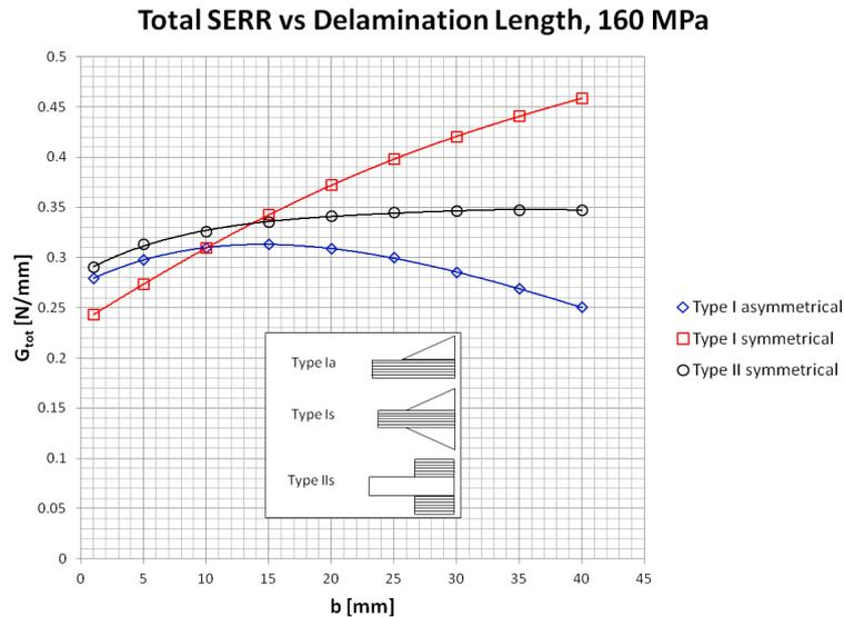
**Figure 5.2:** Total strain energy release rate as a function of delamination length for the three configurations tested, at an applied stress of 160 MPa. The lines are 4th order polynomial trendlines through the calculated points.
