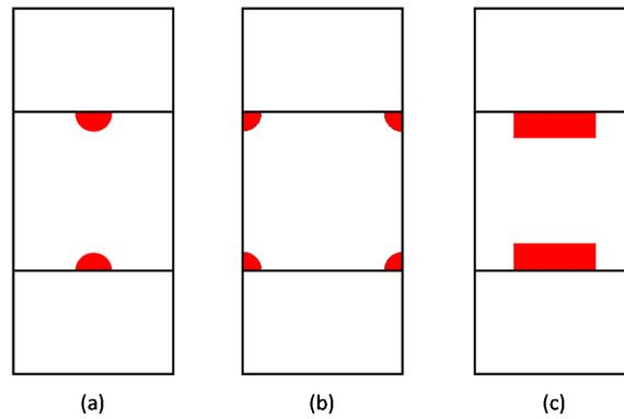
**Figure 5.16:** Delamination shapes analysed: (a) half penny-shaped delamination in the centre of the patch edge; (b) Quarter-circular delaminations from the patch corners and (c) rectangular crack in the centre of the width.
