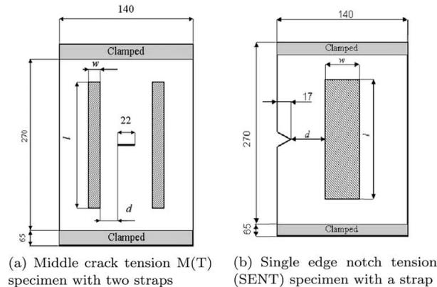
**Figure 2.2:** Configurations used for the validation of the Boscolo-Zhang model, figure from [27].
