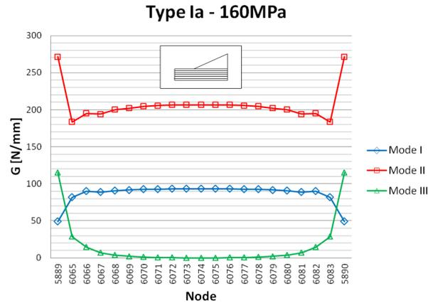
**Figure 5.8:** Distribution of the SERR components over the specimen width for a Type I asymmetric configuration with a 10 mm delamination.
