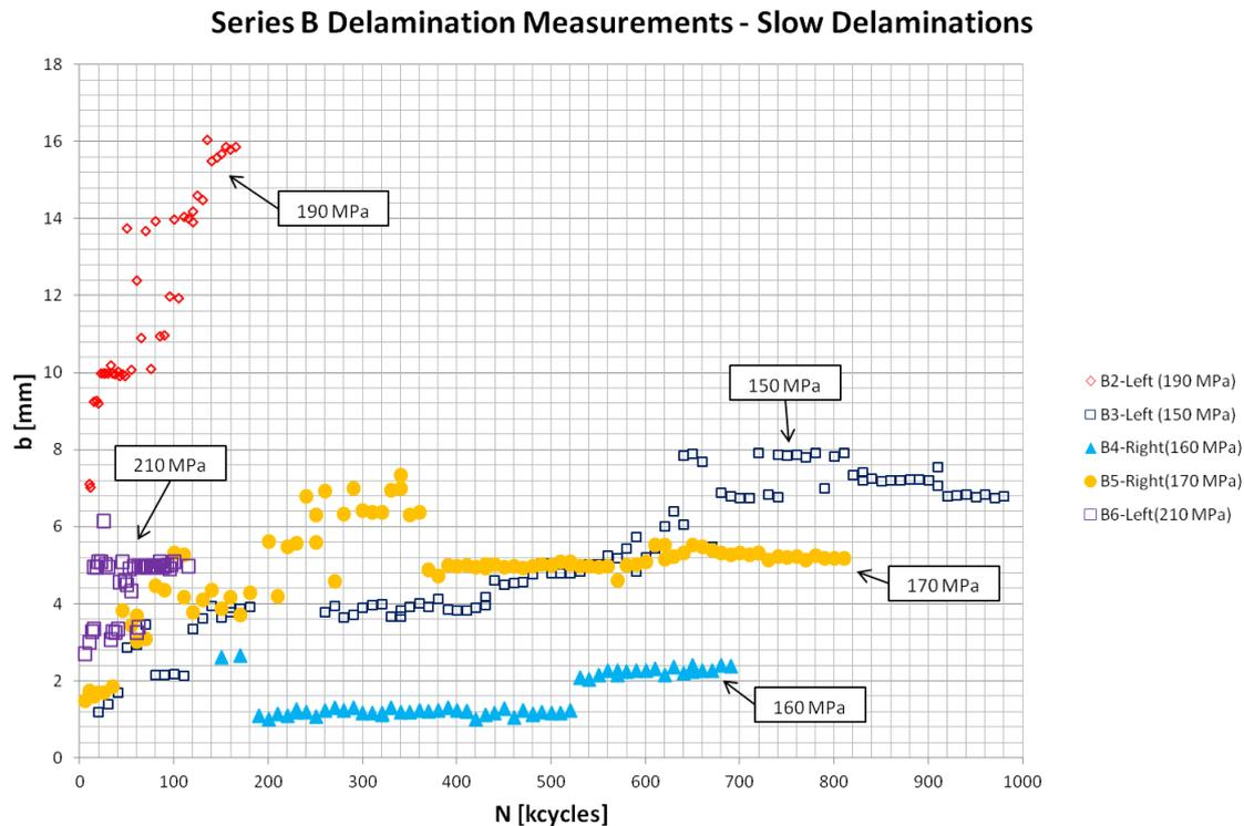
**Figure 6.7:** Measurement data for the slow delaminations of the series B specimens.
