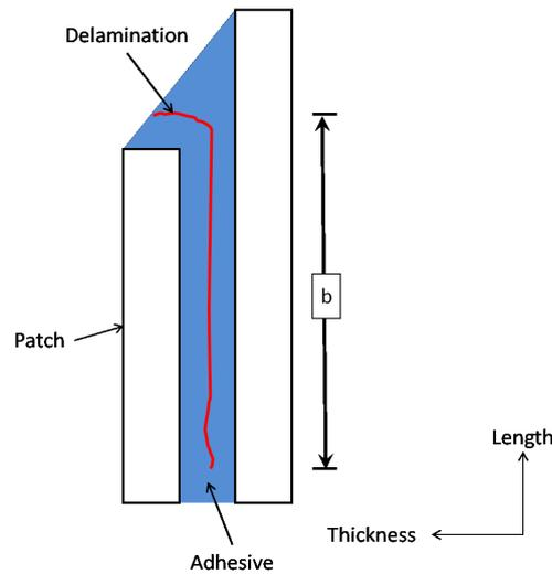
**Figure 6.3:** Definition of delamination length  $b$ . Delamination length was defined from the mouth of the delamination to the tip of the delamination. As the objective of the test was to measure delamination growth rate a fixed length offset will not affect the results of the test.
