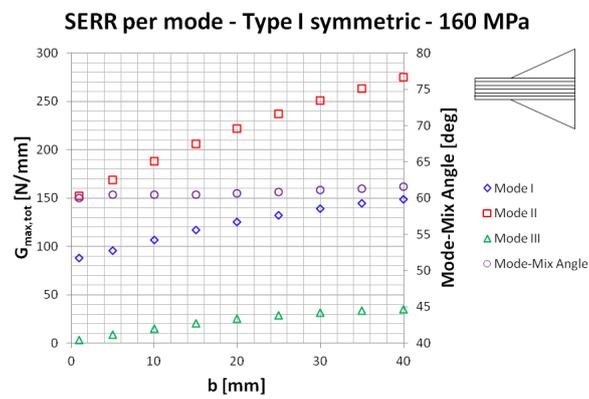
**Figure 5.5:** Distribution of the modal components of the SERR as a function of delamination length for a Type I symmetric specimen.
