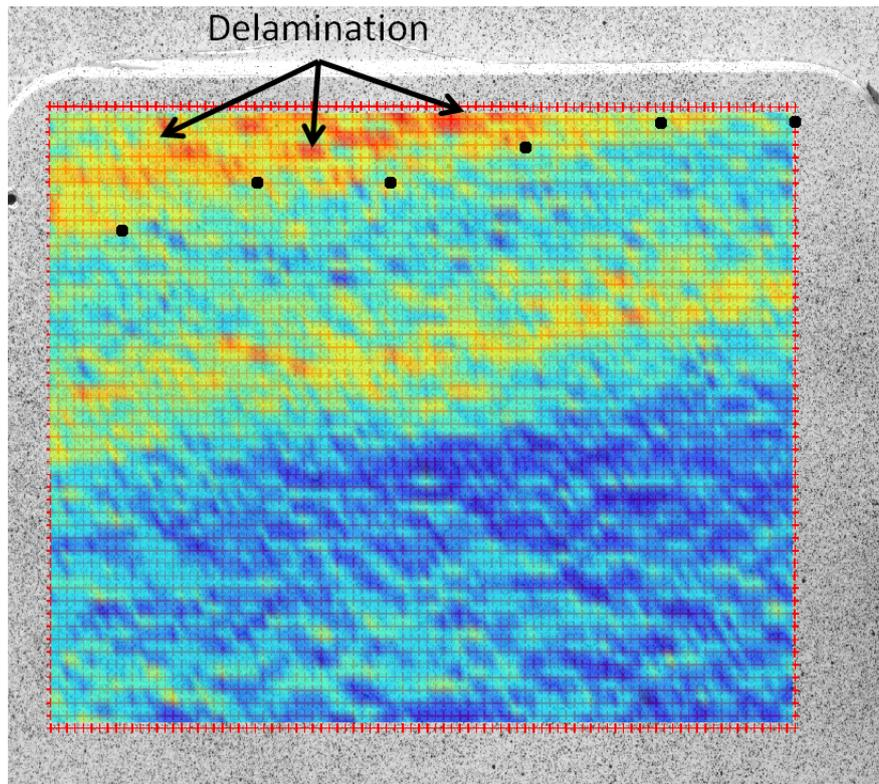
**Figure 6.19:** DIC image for specimen C2 at 20 kcycles and maximum fatigue load. The calculated strain field is superimposed, showing the delaminated area. The points used for the delamination measurements are marked by the black circles.
