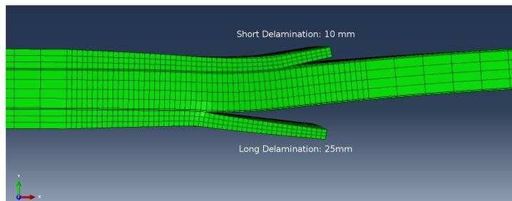
**Figure 5.15:** Secondary bending caused by asymmetric delamination growth. The bending causes closure of the shorter delamination. A scale factor of 50 has been applied to the magnitude of the deformations to enhance visibility.
