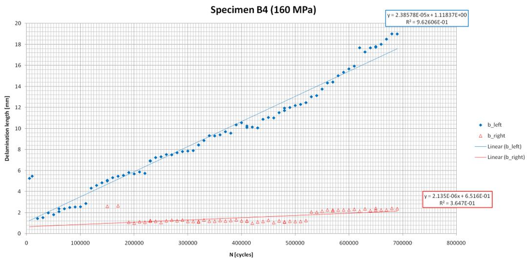
**Figure A.7:** Delamination lengths measured for specimen B4.
