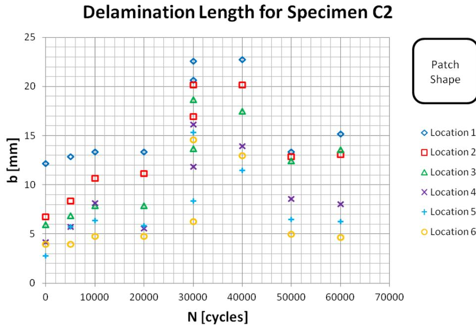
**Figure 6.20:** Delamination length measurements for specimen C2.
