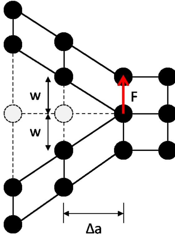
**Figure 2.1:** The virtual crack closure technique; only the nodes in the vicinity of the crack tip are shown. The SERR is found by considering the work done by force  $F$ , when closing the crack over the distance  $\Delta a$ , by displacement of the nodes behind the crack tip over the distance  $w$ . Note that the nodal displacements here are shown as being equal, but this is not necessary.
