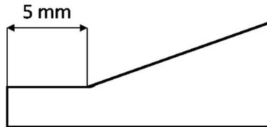
**Figure 3.2:** Detail of the tapering at the patch ends of series A specimens. Figure is not to scale.
