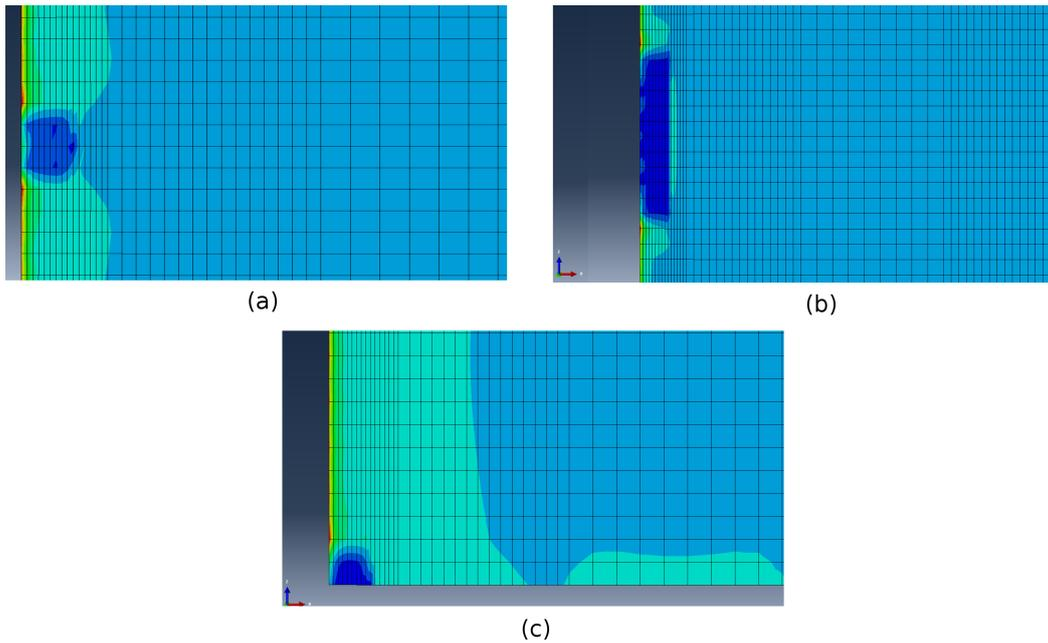
**Figure 5.17:** Results of FEA showing the von Mises stress distribution on the underside of the patch for various delamination shapes: (a) a half-penny shaped delamination in the centre of the patch width; (b) quarter-circular delaminations from the patch corners and (c) rectangular crack in the centre of the width. Areas of highest stress are in red, areas of lowest stress are coloured blue.
