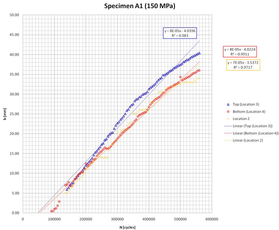
**Figure A.2:** Delamination lengths measured for specimen A1. Measurements done at location 2 were performed using the naked eye and a ruler and so are less accurate.
