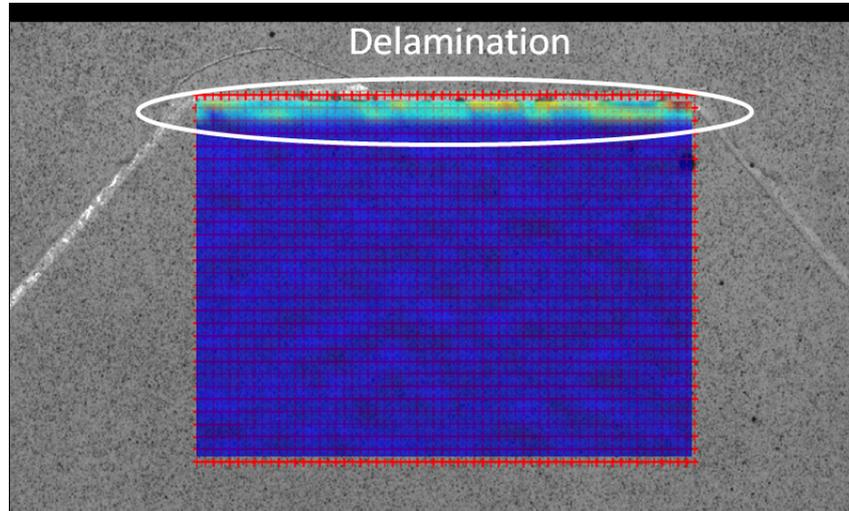
**Figure 6.22:** DIC image for specimen C4 at 170 kcycles and maximum fatigue load.
