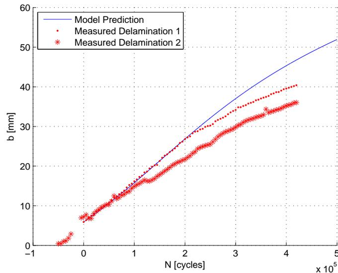
**Figure 7.3:** Delamination growth prediction for specimen A1 based on  $G_{II,max}$ .
