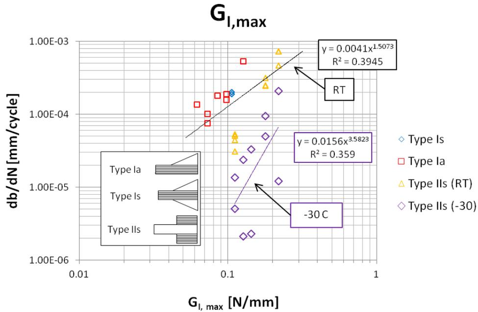
**Figure 6.9:** Delamination growth rate plotted as a function of maximum mode I SERR. Power-law curve fits are shown both for the specimens tested at room temperature and for the specimens tested at -30°C.
