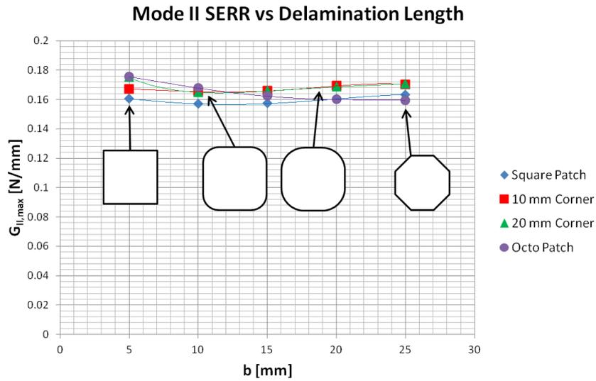
**Figure 5.25:** Mode II SERR vs delamination length for the patch repair specimens, including 4th order polynomial trendline.
