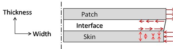
**Figure 5.7:** Stress distribution in the specimen cross-section, with the cut made at the delamination tip. The difference in Poisson ratio, combined with spring-back of the disbonded portion of the patch, result in a difference in the stress in width direction. This causes bending of the patch and skin and a non-constant peel stress distribution.
