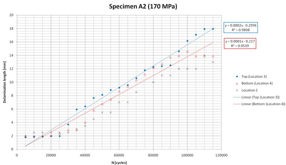
**Figure A.3:** Delamination lengths measured for specimen A2. Measurements done at location 2 were performed using the naked eye and a ruler and so are less accurate.
