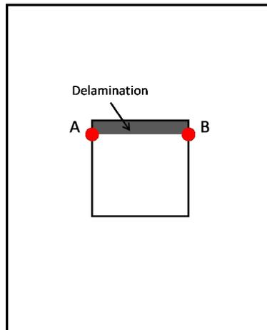
**Figure 5.20:** Location of the nodes on the delamination front at the patch edge
