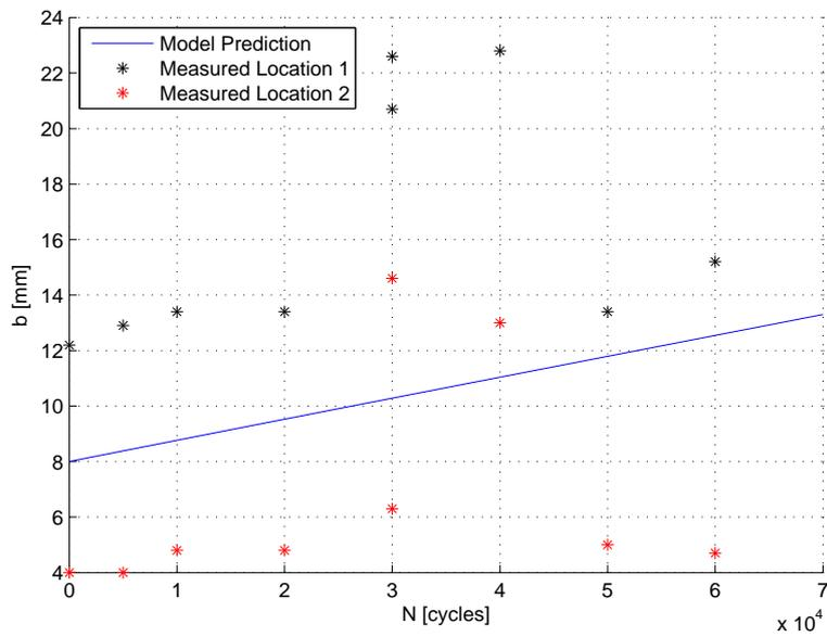
Figure 7.6: Delamination growth prediction for specimen C2 based on  $G_{II,max}$ .
