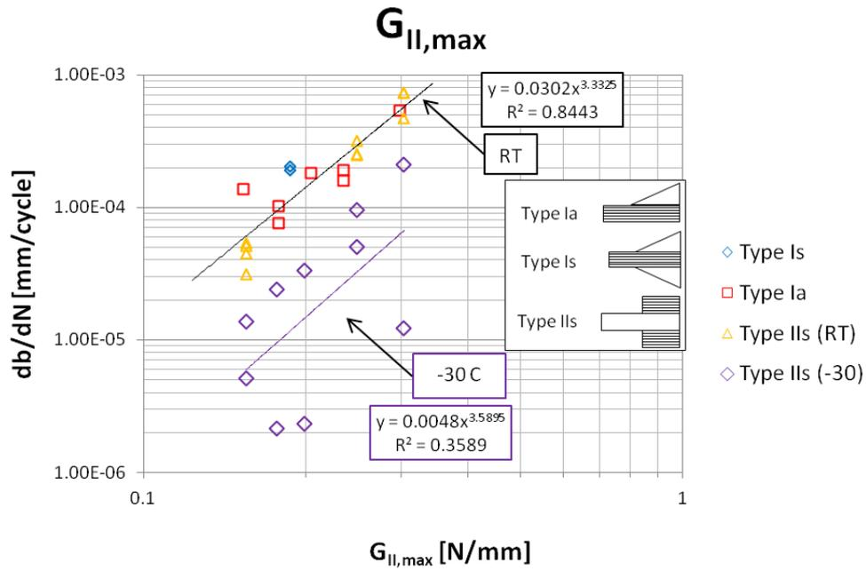
**Figure 6.10:** Delamination growth rate plotted as a function of maximum mode II SERR. Power-law curve fits are shown both for the specimens tested at room temperature and for the specimens tested at -30°C.
