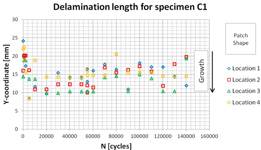
**Figure 6.17:** Delamination length measurements for specimen C1. The vertical axis shows the y-coordinate of the delamination front, measured from the bottom of the DIC image. A decrease of the y-coordinate implies delamination growth, as indicated.
