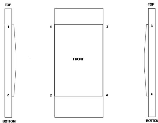
**Figure A.1:** Nomenclature used for series A specimens. Adapted from a figure by C. Rans (unpublished).
