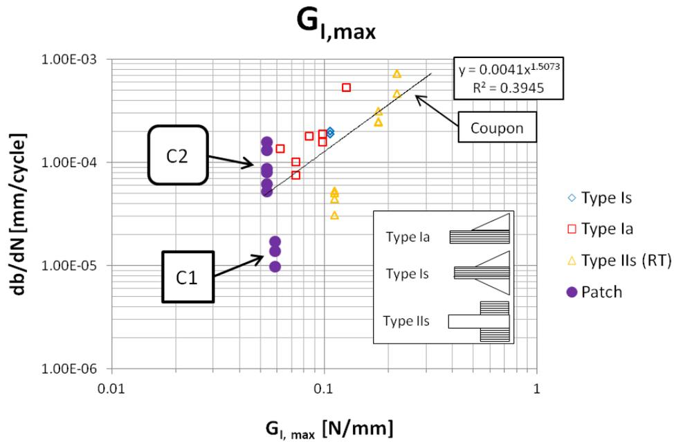
**Figure 6.24:** Delamination growth rate plotted as a function of mode I SERR. The power-law curve fit shown is based only on the material coupon data. Delamination growth rate of specimens C1 and C2 is shown for each measurement location separately.
