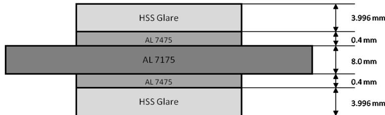
**Figure 3.5:** Schematic overview of the configuration of series B specimens. Figure is not to scale.
