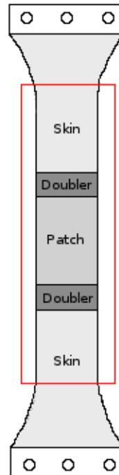
**Figure 4.1:** Schematic view of the Type I specimen. The red box indicates the area included in the FE model.
