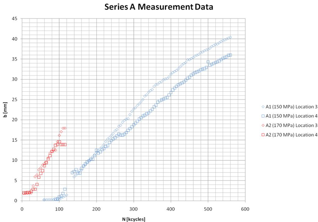
**Figure 6.2:** Measurement data for the Series A specimens.
