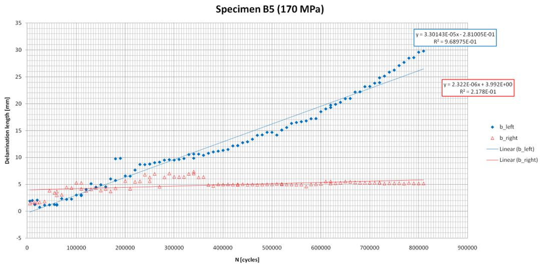
Figure A.8: Delamination lengths measured for specimen B5.
