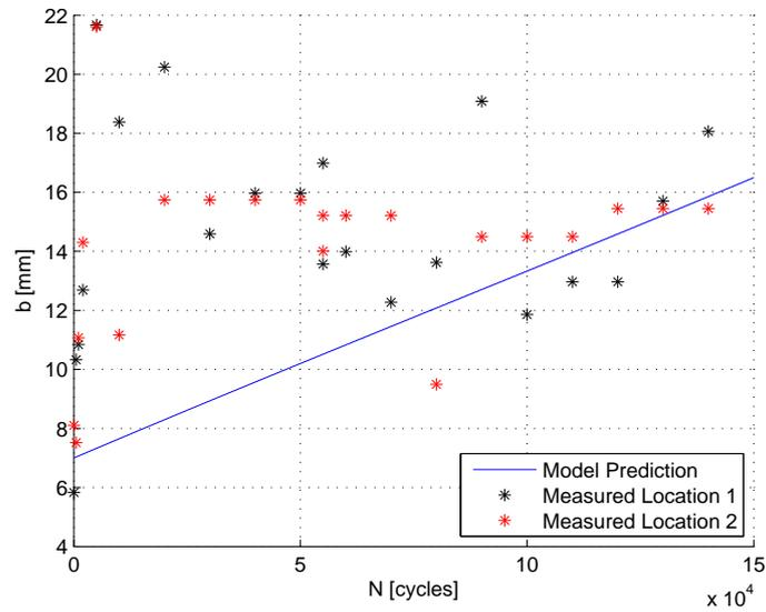
Figure 7.5: Delamination growth prediction for specimen C1 based on  $G_{II,max}$ .
