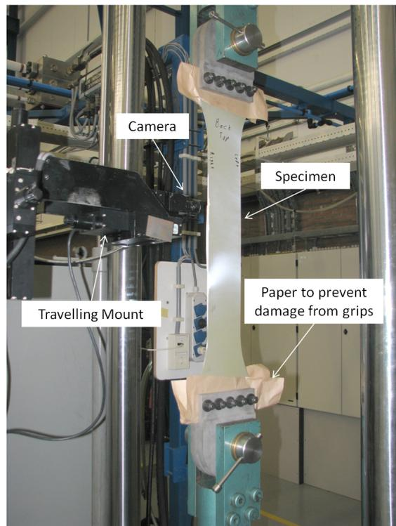
**Figure 3.3:** Test set-up, showing the specimen installed in the test machine and the travelling camera used for delamination length measurements.
