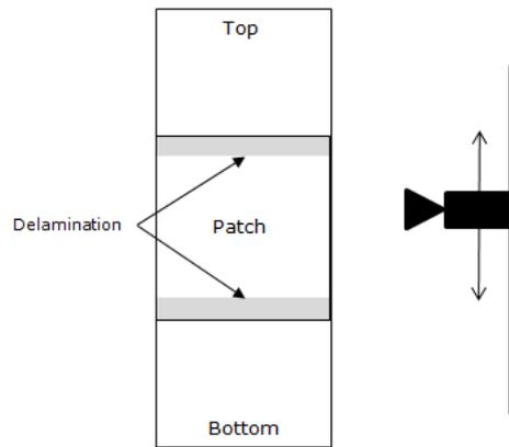
**Figure 3.4:** Schematic overview of the position of the camera used to monitor delamination growth.
