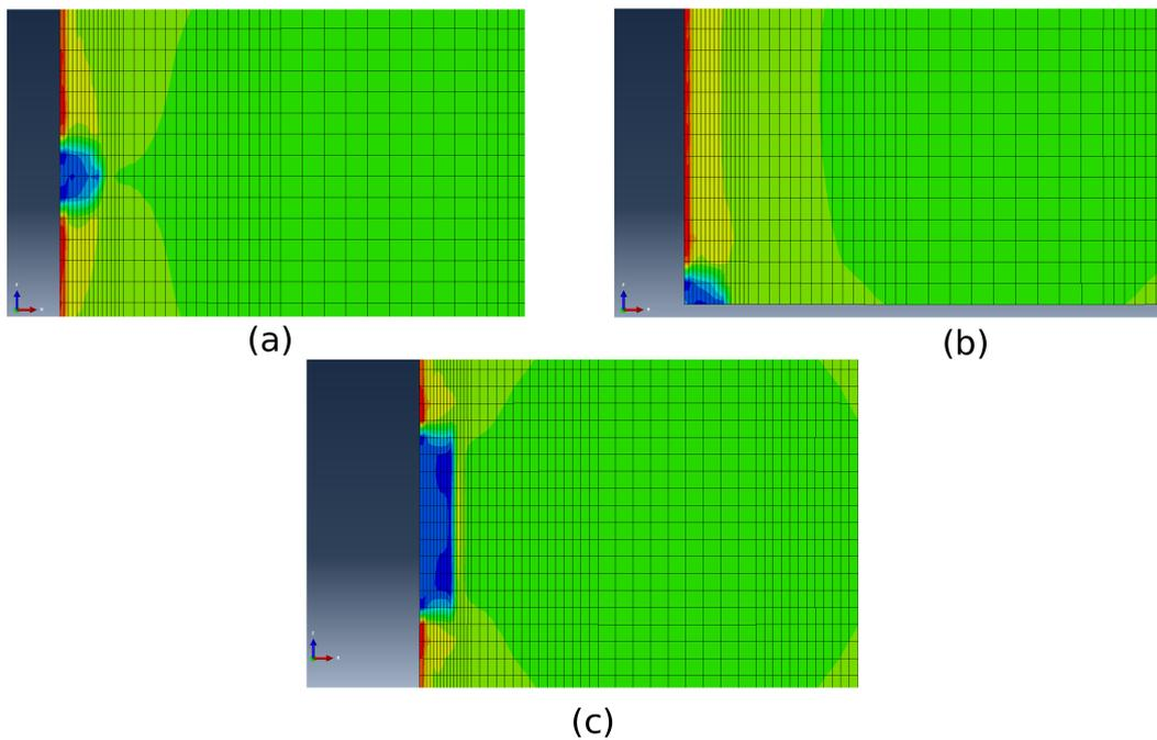
**Figure 5.18:** Results of FEA showing the distribution of normal stress in loading direction on the underside of the patch for various delamination shapes, as identified in figures 5.16 and 5.17. Areas of highest stress are in red, areas of lowest stress are coloured blue.
