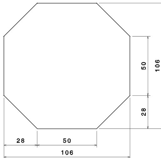
**Figure 3.8:** Dimensions (in mm) of the octagonal patch.
