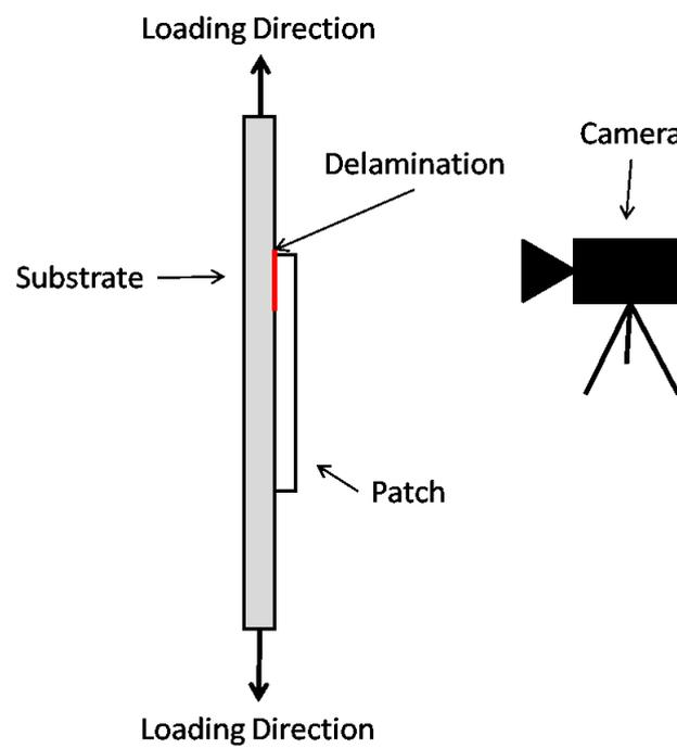
**Figure 3.9:** Schematic overview of the position of the DIC camera(s) used to monitor delamination growth for the patch repair specimens.
