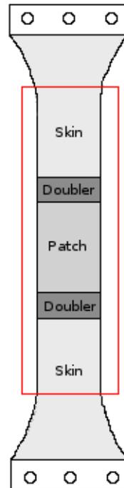
**Figure 4.1:** Schematic view of the Type I specimen. The red box indicates the area included in the FE model.
