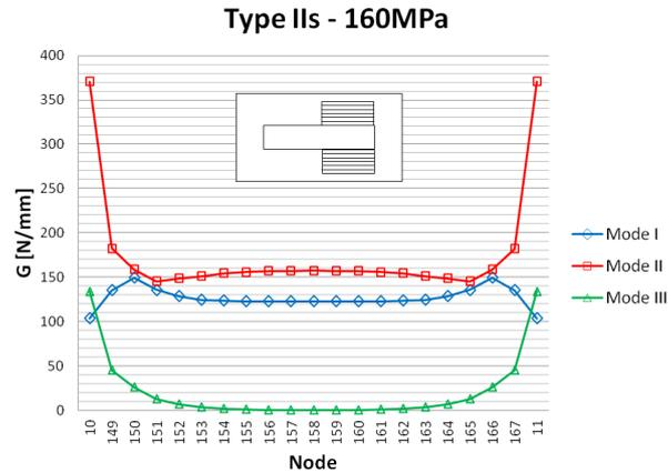
**Figure 5.10:** Distribution of the SERR components over the specimen width for a Type II symmetric configuration with a 10 mm delamination.
