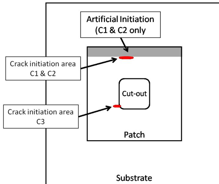
**Figure 6.15:** Schematic overview of the fatigue crack initiation locations. All fatigue cracks initiated in the substrate.
