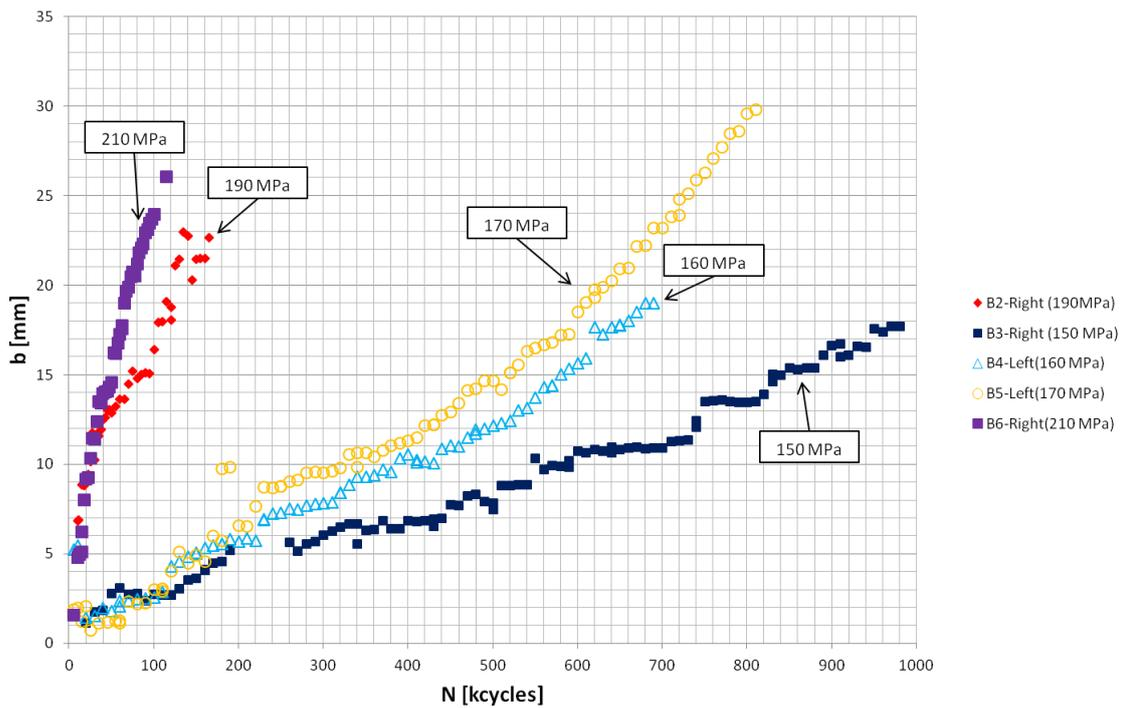
Figure 6.6: Measurement data for the fast delaminations of the series B specimens.
