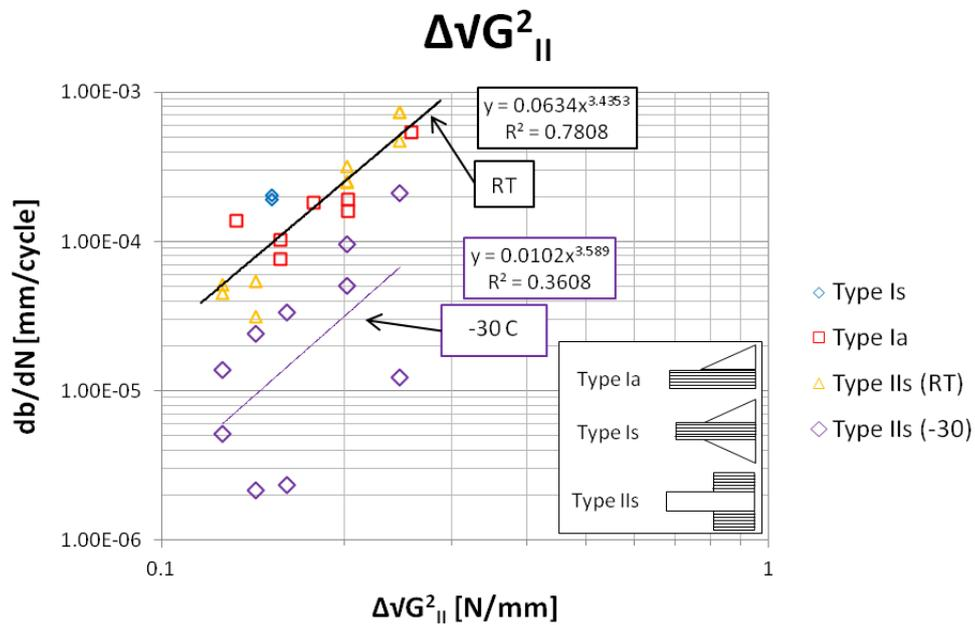
Figure 6.13: Delamination growth rate plotted as a function of mode II SERR range. Power-law curve fits are shown both for the specimens tested at room temperature and for the specimens tested at  $-30^\circ C$ .
