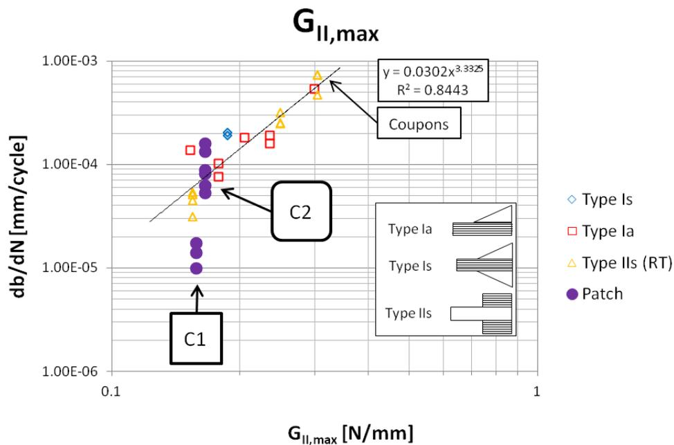
**Figure 6.25:** Delamination growth rate plotted as a function of mode II SERR. The power-law curve fit shown is based only on the material coupon data. Delamination growth rate of specimens C1 and C2 is shown for each measurement location separately.
