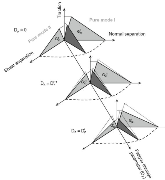
**Figure 2.4:** An example of a multi-mode bi-linear constitutive traction-displacement relation in a CZM. The traction depends on deformation in two directions (modes). The relation between traction and separation is described by two straight lines. The damage parameter  $D$  is used to reduce the stiffness, and thus the traction for a given displacement. Image from [32].
