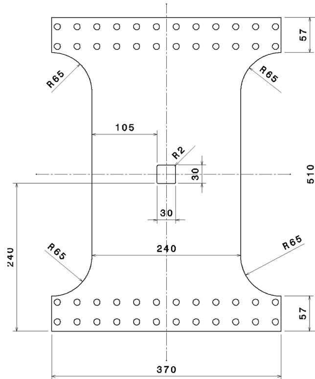
**Figure 3.7:** Base-plate used for the series C specimens. Top view, dimensions in mm.
