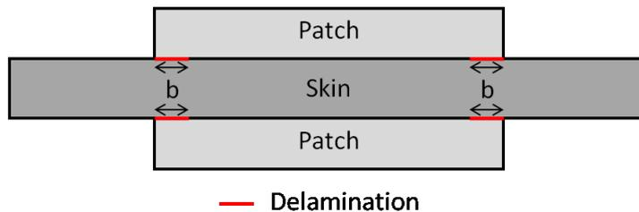
**Figure 5.1:** Definition of delamination length  $b$ .
