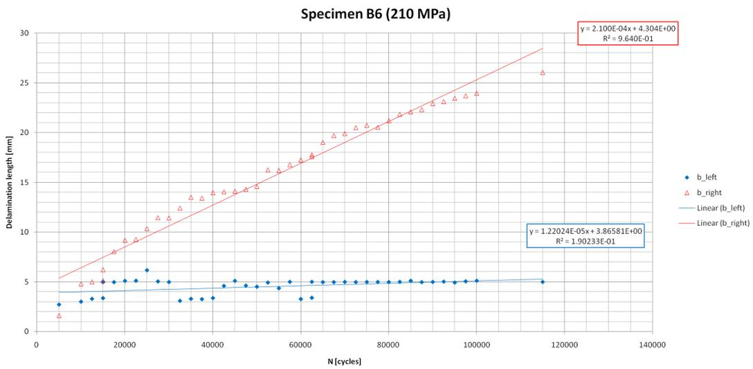
Figure A.9: Delamination lengths measured for specimen B6.
