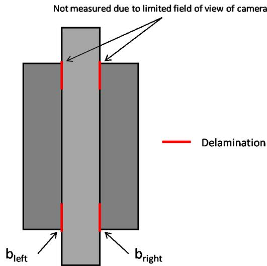
Figure 6.5: Nomenclature used for series B specimens.
