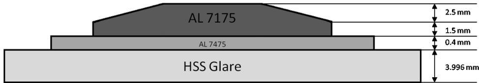
**Figure 3.1:** Schematic overview of the configuration of series A specimens. Figure is not to scale.
