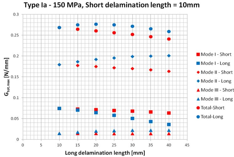
**Figure 5.13:** SERR for differential delamination growth in a Type I asymmetric specimen. The delamination nomenclature is illustrated by figure 5.12.
