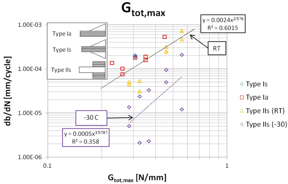
**Figure 6.8:** Delamination growth rate plotted as a function of maximum total SERR. Power-law curve fits are shown both for the specimens tested at room temperature and for the specimens tested at -30°C.
