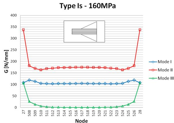
**Figure 5.9:** Distribution of the SERR components over the specimen width for a Type I symmetric configuration with a 10 mm delamination.
