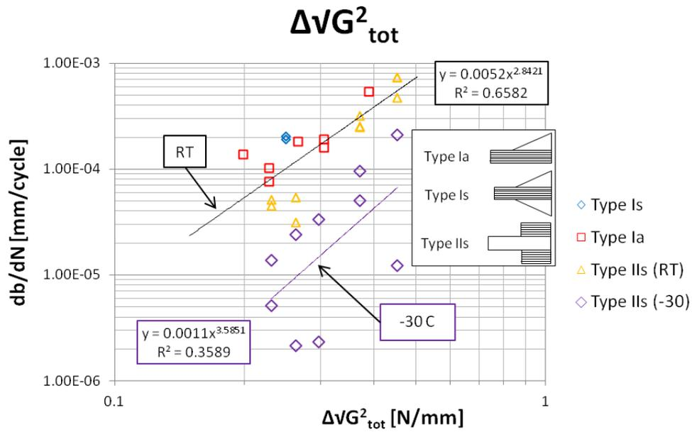
**Figure 6.11:** Delamination growth rate plotted as a function of total SERR range. Power-law curve fits are shown both for the specimens tested at room temperature and for the specimens tested at -30°C.
