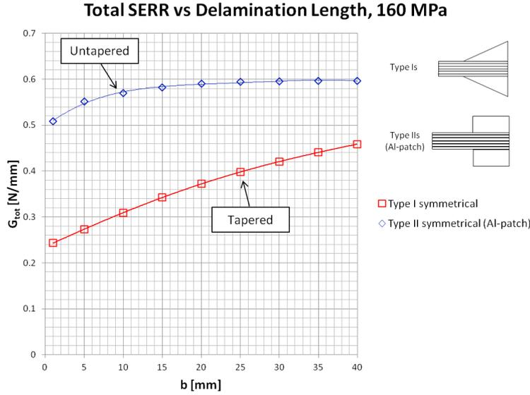
**Figure 5.3:** Comparison between  $G$  vs  $b$  behaviour for a Type I (tapered) symmetrical configuration and a Type II (untapered) symmetrical configuration if both used the same materials for the patch and the skin. This figure shows clearly the benefit of applying taper; a benefit that was hidden by the change in materials in the actual specimens.
