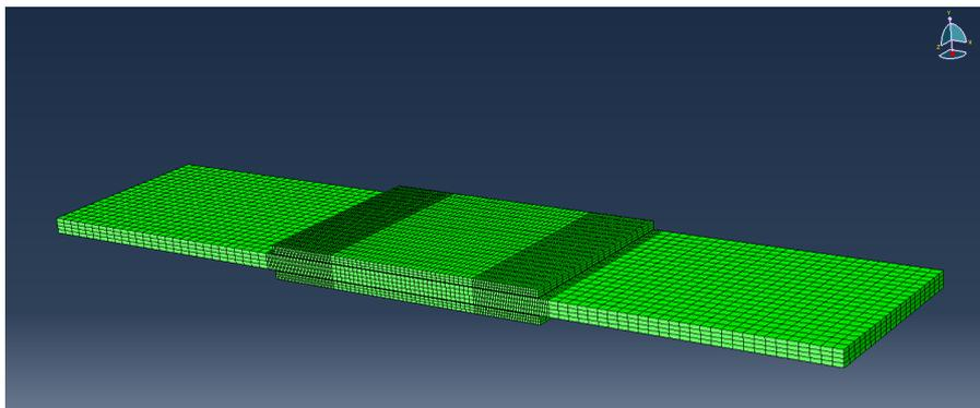
**Figure 4.2:** Mesh used for the FEA of the Type II symmetric specimens, with a delamination length of 30mm.
