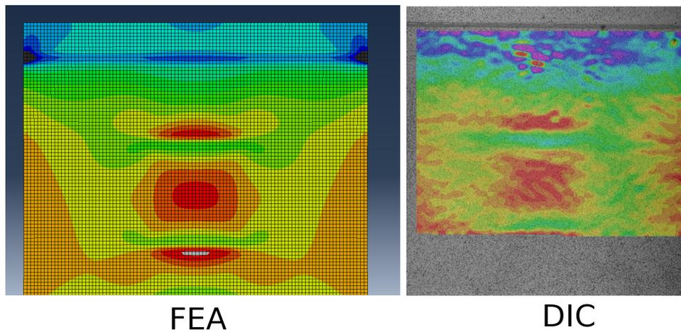
**Figure 6.16:** Comparison between the strain field predicted by FEA (left) and the strain field as measured by DIC (right). Black/blue/purple indicates areas of lowest strain, red/grey indicates areas of highest strain. The two high strain areas visible in the delaminated (low strain) area in the DIC image are thought to be measurement errors caused by damage of the CCD-chip in the camera used. The FEA image shows true strain, whereas the DIC image shows engineering strain.
