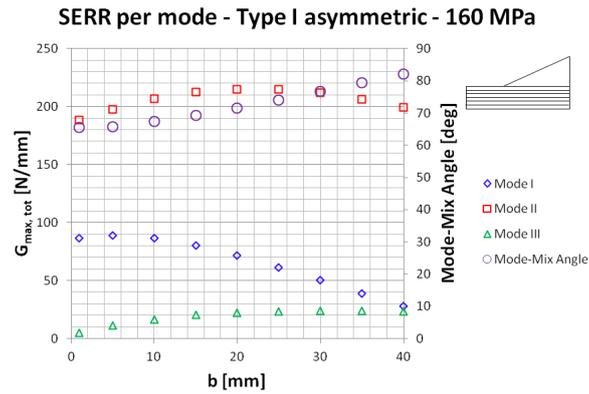
**Figure 5.4:** Distribution of the modal components of the SERR as a function of delamination length for a Type I asymmetric specimen.
