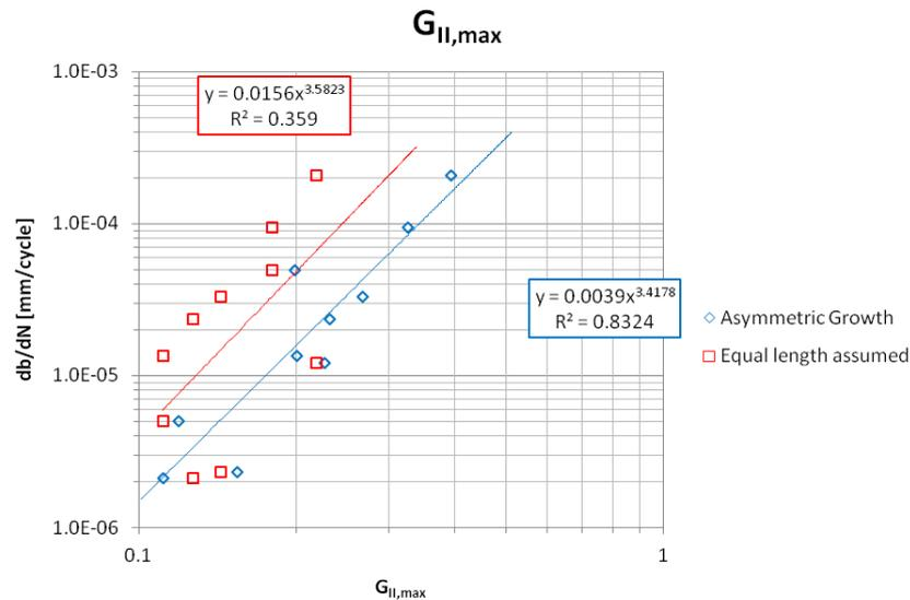
**Figure 6.14:** Comparison of the delamination growth rate as a function of maximum mode II SERR for the series B specimens, both with and without taking into account asymmetric growth.
