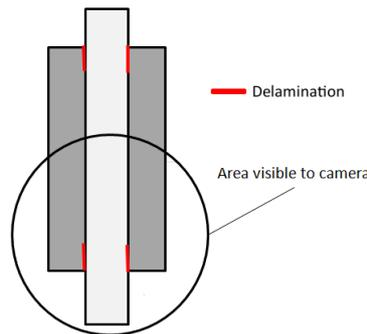
**Figure 3.6:** Estimate of the field of view of the camera during testing of series B.
