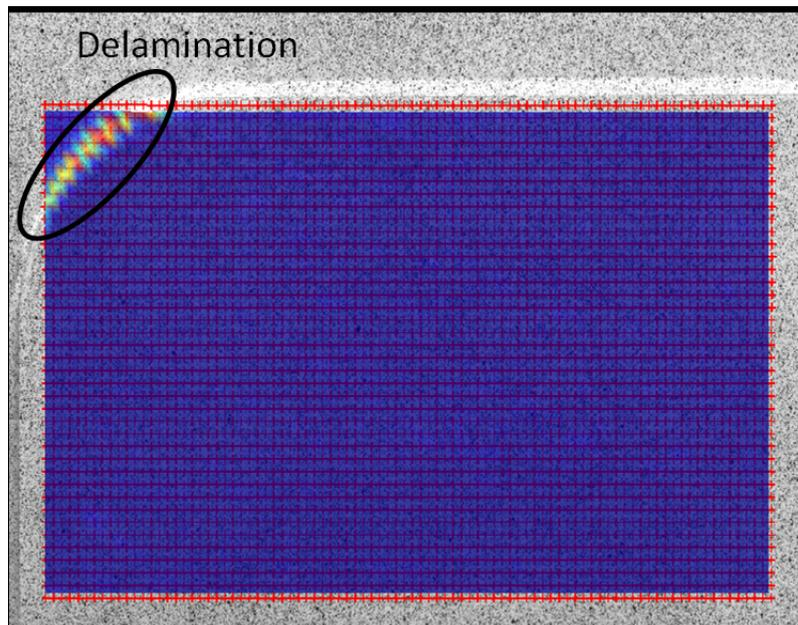
**Figure 6.21:** DIC image for specimen C3 at 170 kcycles and maximum fatigue load. The specimen failed due to fatigue cracking of the substrate shortly afterwards.
