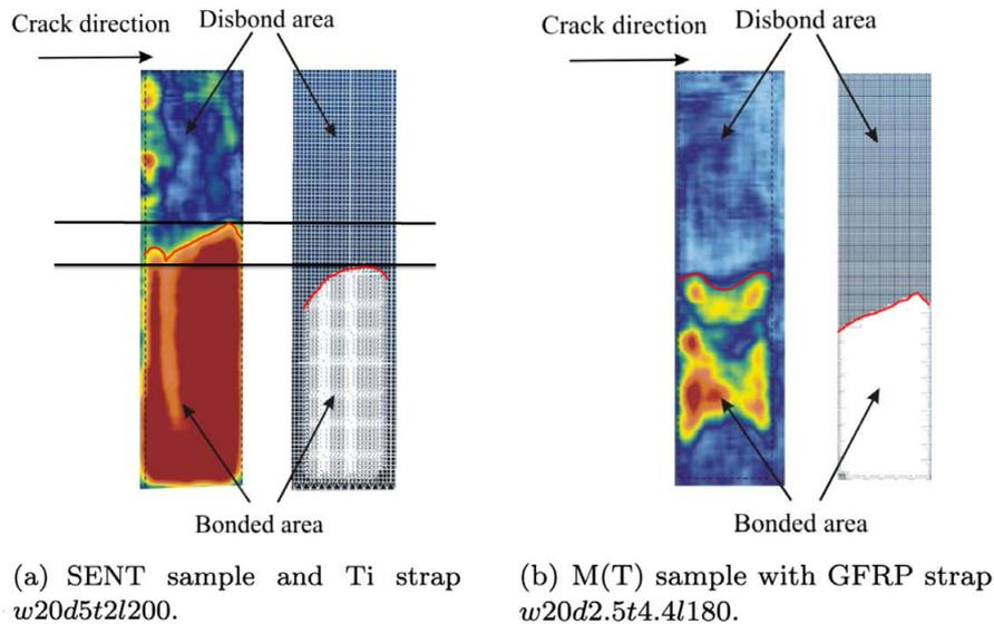
**Figure 2.3:** Delamination as predicted by the Boscolo-Zhang model compared with experimental results. Only half of the strap is shown, the top edge in the figure is the centre line of the strap. Figure from [27]. Horizontal lines showing extent of predicted and measured delamination as well as curves highlighting the delamination front added for emphasis.
