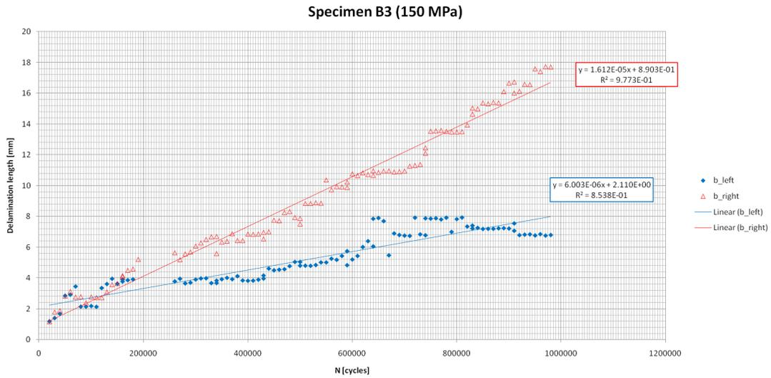
**Figure A.6:** Delamination lengths measured for specimen B3.
