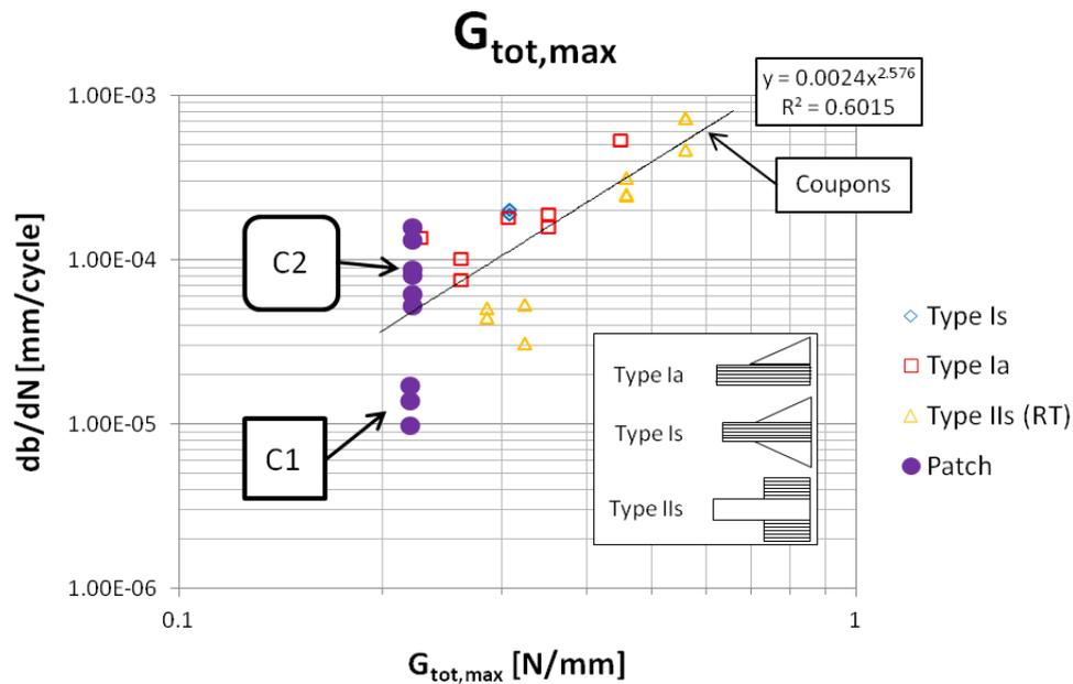
**Figure 6.23:** Delamination growth rate plotted as a function of total SERR. The power-law curve fit shown is based only on the material coupon data. Delamination growth rate of specimens C1 and C2 is shown for each measurement location separately.
