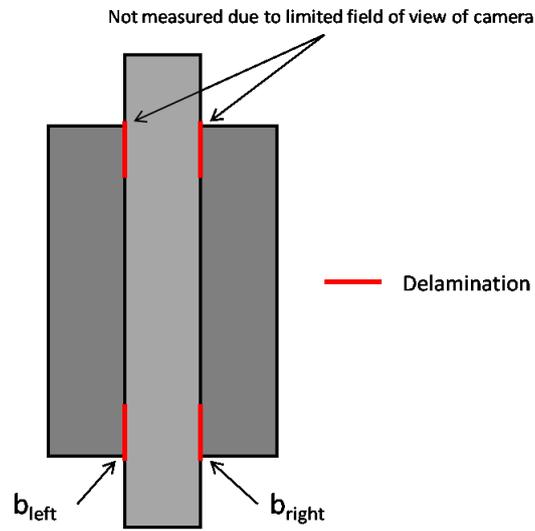
Figure A.4: Nomenclature used for series B specimens.
