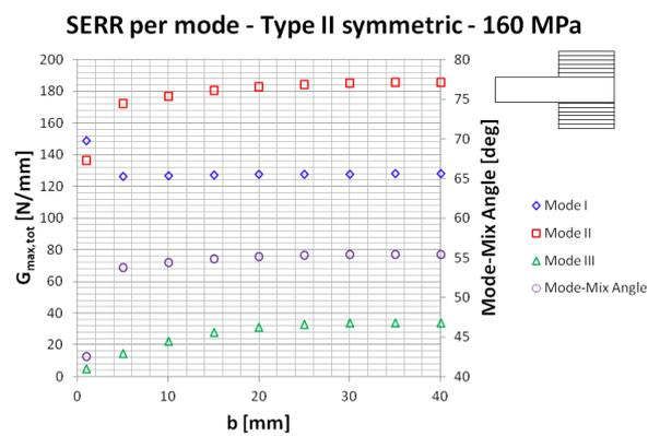
**Figure 5.6:** Distribution of the modal components of the SERR as a function of delamination length for a Type II symmetric specimen.
