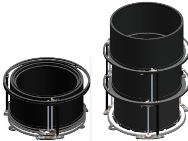
Fig. 7 Concept of the SSTL telescopic deployment barrel. 6
