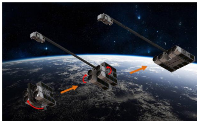
Fig. 15 View of the reconfiguration mechanism of AAReST, also showing the integrated tape spring hinge. 112
