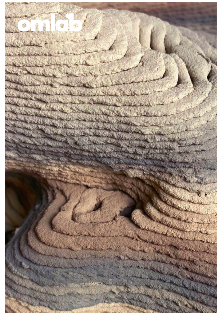
Figure 7. Images of pilot-scale Kaumera construction products. Top: Re-Plex (Sauerwein et al., 2023). Bottom : Buildmatterial 0.8 (MaterialDistrict. 3D Printing With Waste Material From Water Treatment, 2021)
