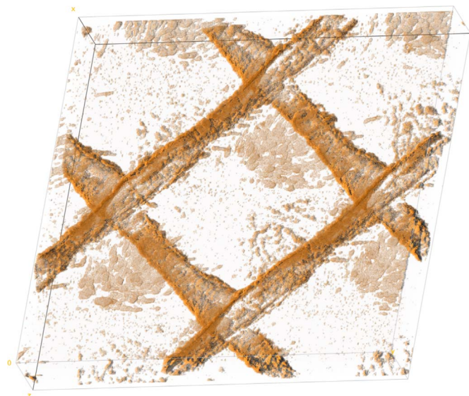
Fig. 4. Three-dimensional (3D) rendered OCT image with biomass (brown color), the spacer, membrane and cover glass were eliminated by using the scan at time zero as baseline. (For interpretation of the references to color in this figure legend, the reader is referred to the web version of this article.)
