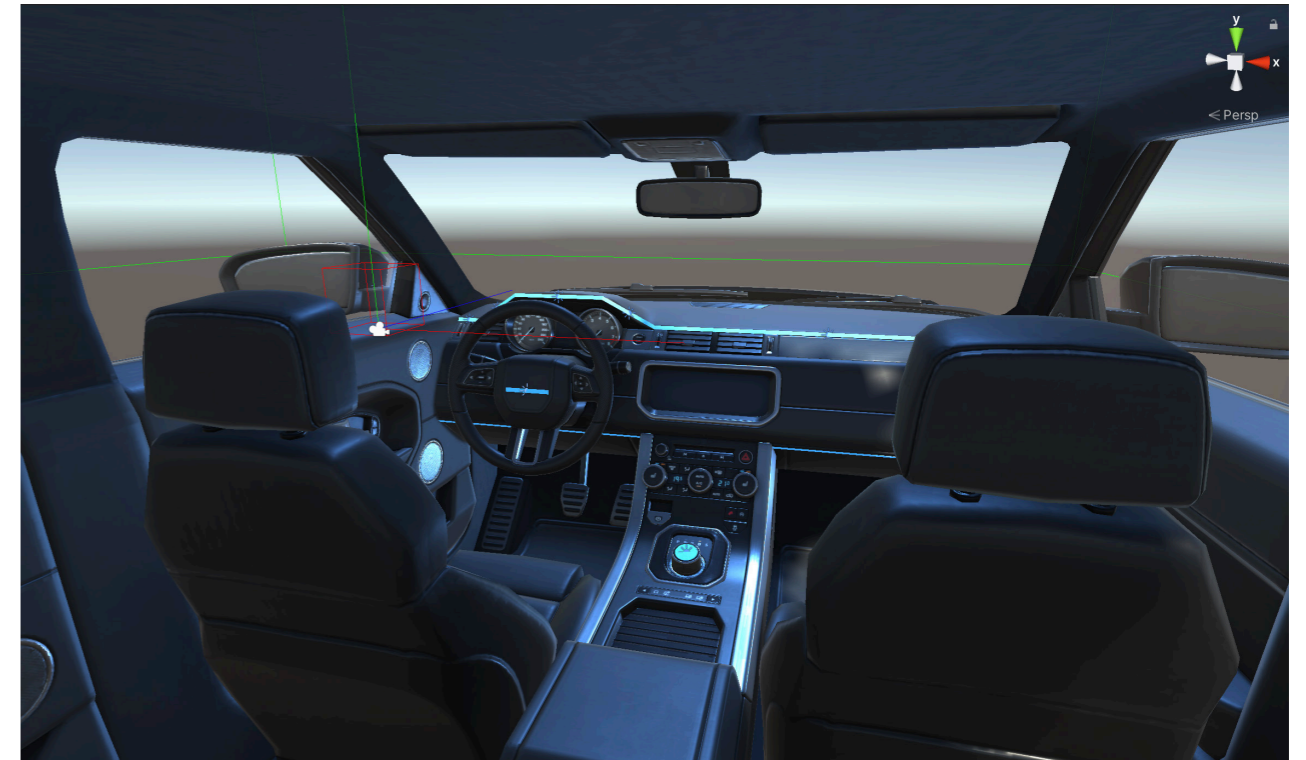
Figure 17: Virtual environment of MVP1. In the image, the version containing the dashboard and ambient lighting LED strips (in blue) is shown. The virtual prototypes are placed inside of a vehicle asset 1 .
