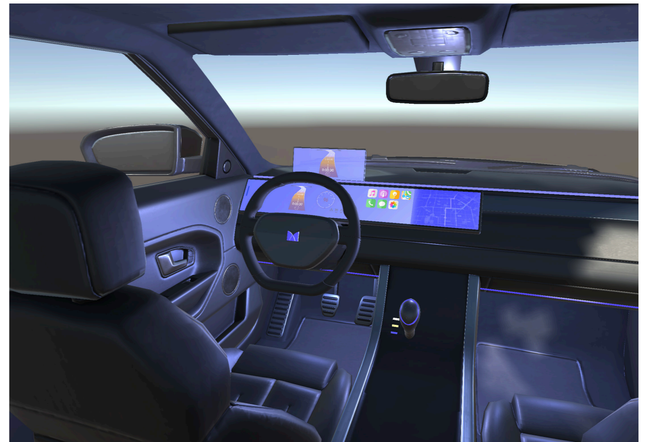
Figure 23: Modified vehicle asset. The large screen, head/up/display, LED lighting, wheel and shifter were changed or added to recreate the Mediator HMI design.
