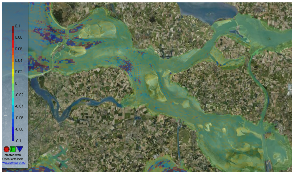
Figure 5.32: Sedimentation/erosion pattern of the present situation, red is sedimentation and blue is erosion in metres
