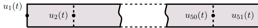
Figure 6-1: Model of a linear bar consisting of 50 elements of equal length. Note that 50 elements require a total of 51 nodes.
