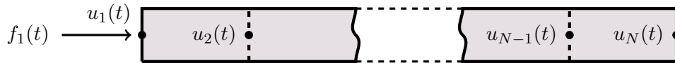
Figure 5-2: Model of a linear bar consisting of N elements of equal length.
