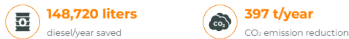
Figure 6.21: The reduction in emissions and fuel consumption of Island Discovery ship according to the battery provider, Corvus Energy [23]
