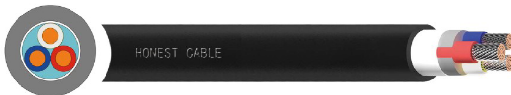
Figure 3.4: The cross-section of a marine cable used in this study. It consists of three wires per phase made up of annealed copper strands protected by XLPE insulation. The outermost insulation is also made of XLPE insulation as well [46].
