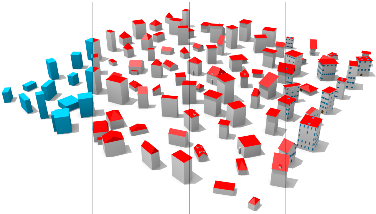
Figure 4: Composite rendering of a few exemplary datasets generated by RANDOM3DCITY: randomly generated buildings realised in CityGML in four LODs. The two representations on the left have their walls modelled as projections from roof edges as opposed to the third panel where the walls are modelled at their actual location and where roof overhangs are explicitly modelled, showing varying geometric references that are supported by the engine, besides multiple geometric and semantic LODs.
