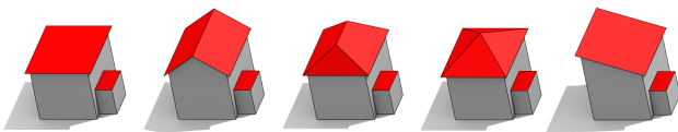
Figure 5: Different types of roofs (flat, gabled, hipped, pyramidal, and shed) fitted on the same building, with the automatically adjusted walls. This image shows the LOD2 (orthogonal view), and it also features an example of a building part.
