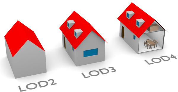
Figure 1: A building modelled in multiple LODs. The LOD labels are according to the categorisation of CityGML 2.0, and they denote both the granularity of the geometry and semantics. Besides small and illustrative models such as this one, building datasets containing multiple LODs are virtually non-existent.
