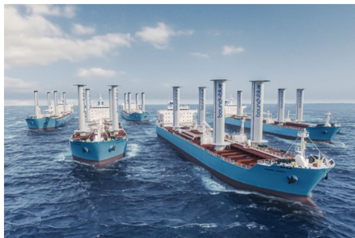
Figure 12: An illustration of Bound4Blue eSails on the Maersk tankers ( Camps, 2024 )
