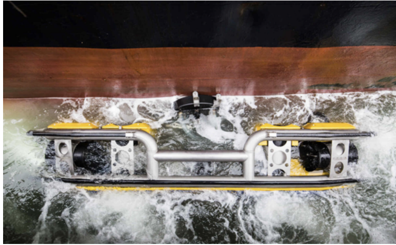
Figure 17: Hull cleaning by Damen (Offshore-Energy, 2024)
