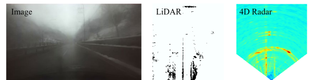
Figure 2.3: Comparison of a snapshot of a camera, LiDAR and Radar system [57].
