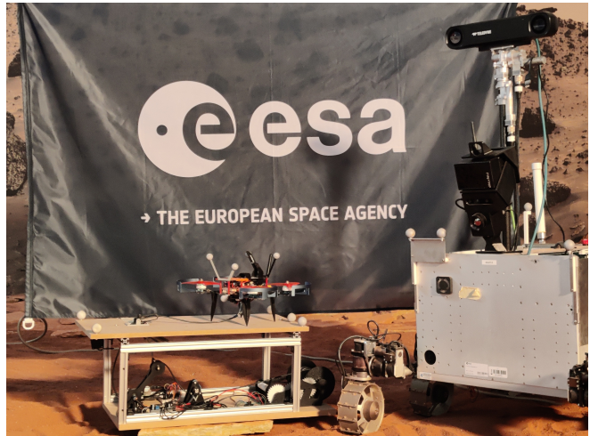
Fig. 1. The Tether Management System with the HolyBro QAV250 drone next to the MaRTA rover in the Mars yard of the PRL at ESA, ESTEC. The drone uses the TI Localization system to compute its position based on the physical properties of the tether: tether length and angles.
