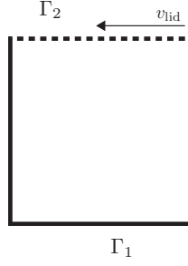
Figure 5.5: Illustration of the domain for the lid-driven cavity problem. The boundaries around the cavity are marked by \Gamma_1 except at the top lid where \Gamma_2 labels the boundary there.
