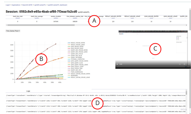
Figure 7: LogUI Session Dashboard. The Statistics Table (A) contains the values for the session for all metrics within the corresponding flight. The Graph View (B) shows visuals for this session. The Screen Recording (C) shows the screen recording of the session. The Logs (D) show all logs from this session. Clicking on a log makes the Screen Recording show the four seconds surrounding that event.
