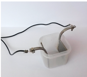
Figure 5.2: Setup for the impedance measurements
