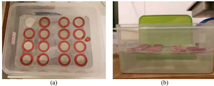
Figure 1: The setup for unidirectional sulfate penetration test
