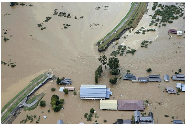
Figure 1. Breach of a dike in Japan in 2019. Image source: The Japan News
