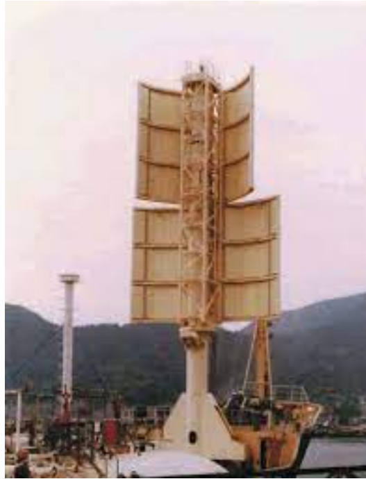
Figure 2.3: JAMDA (rigid) sail on a ship [12]
