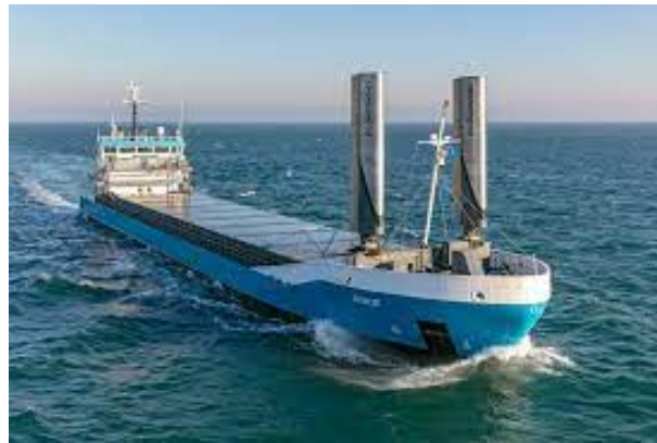
Figure 2.5: The VentiFoil from Enconowind [40]
