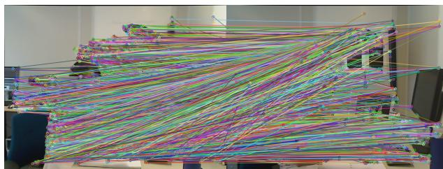
Figure 5.4: Matching result using the Brute-Force matcher
