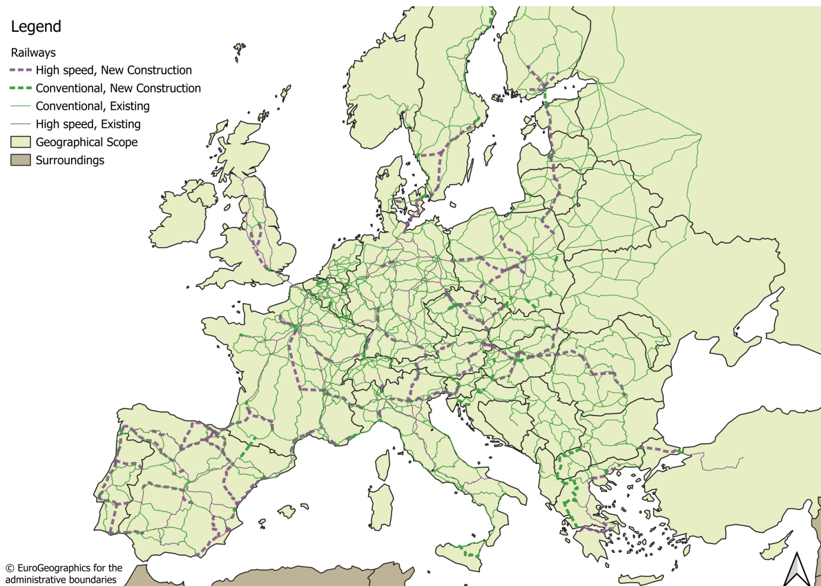
Figure 4.16: The visualisation of which TEN-T railways are planned to be constructed per 2050, and which are already existing. Based on the TEN-T policy (European Commission, 2021b) and created with QGIS (QGIS, 2023).
