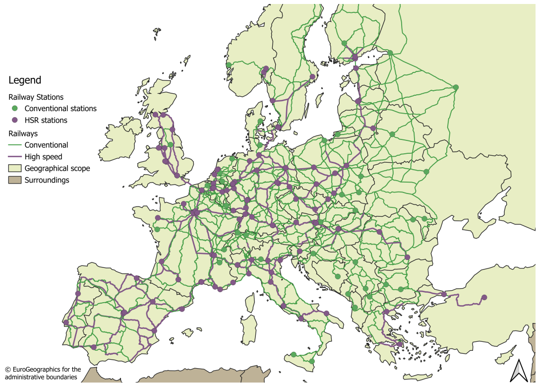
Figure 5.2: Identification of HSR-stations. National borders are adapted from Eurostat (2020a) data. Created with QGIS (2023).
