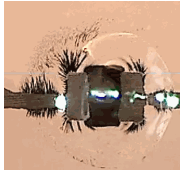
Figure 6.9: Short circuit during dielectrophoresis of NTC particles in a liquid epoxy matrix due to percolation of the NTC particles between the electrodes (Top view).
