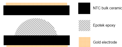
Figure 6.10: Schematic of the sintered NTC ceramic - epoxy stacks.
