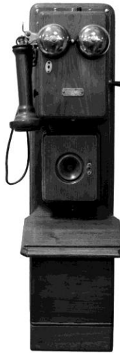
Figure 93: Three Box wall mount telephone made by Viaduct Manufacturing (1893).
