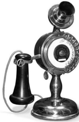
Figure 122: Strowger 11 digit Potbelly Dial Candlestick.
