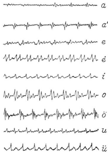
Figure 55: Undulating currents of the acoustic telegraph creating a letter.
