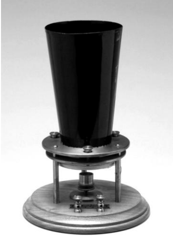
Figure 80: Model of the liquid transmitter (1876).
