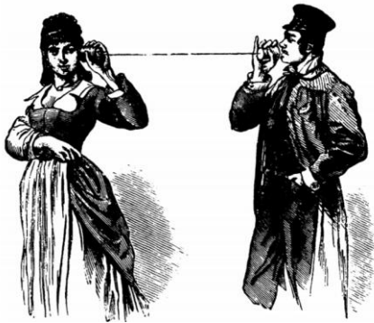
Figure 67: String Telephone or Lover's Telephone.
