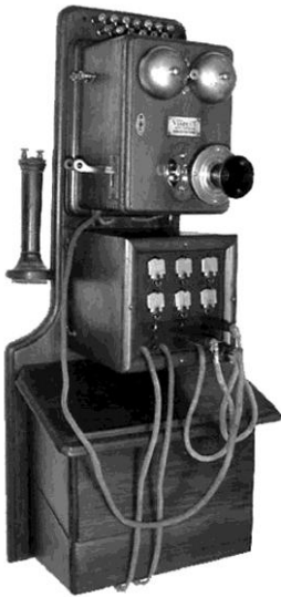
Figure 116: Wall switchboard made by Viaduct Manufacturing Co. (1890s ?)
