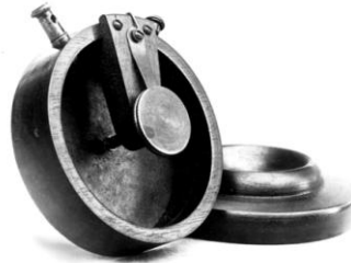
Figure 108: Berliner's microphone of his caveat filed on April 14, 1877.
