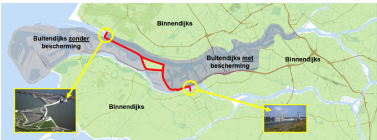
Figure 2.1: Left; Maeslant barrier, right; Hartel barrier and in red the dike protection of the Nieuwe Waterweg
