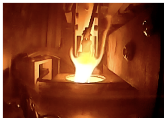
Figure 32: Visual reference (still) frame for gunpowder combustion. (Test ID: DL-1, repetition 4)
