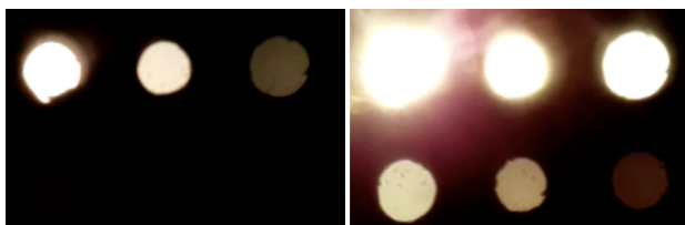
Figure 45: Comparison of recorded fiber camera frames (before color correction) at peak intensity for (left) Ratio A (repetition 1, fiber 2 selected for analysis) and (right) Ratio B (repetition 3, fiber 3 selected for analysis) illustrating the difference in combustion intensity.
