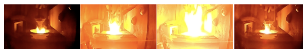
(e) Higher intensity orange flame, pixel intensity > 80 (additional test, orange torch composition mixed with leftover flash powder)
