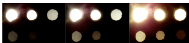
Figure 56: Comparison of recorded fiber camera frames (before color correction) at peak intensity for (left) V-90 (repetition 1, fiber 2 selected for analysis), (middle) V-100 (repetition 4, fiber 3 selected for analysis), and (right) V-110 (repetition 6, fiber 3 selected for analysis) illustrating the difference in combustion intensity when volume increased.
