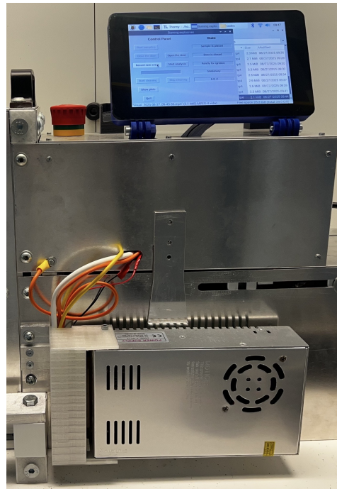
Figure 18: Implementation of the redesigned control unit with the RPi touchscreen display. Showing the assembled and operational setup corresponding to the CAD model in Figure 17.
