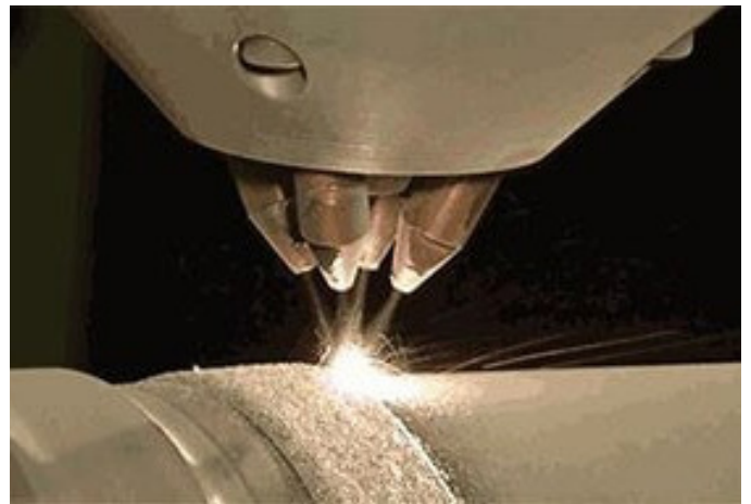
LENS technology being used to repair a metallic part Image Source: 3dprintingindustry.com
