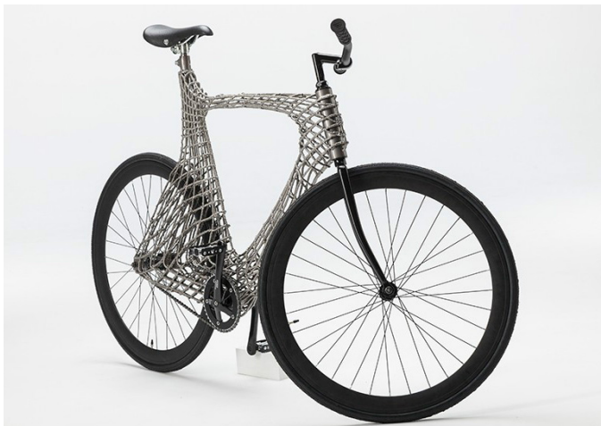
Stainless Steel Bicycle printed using WAAM at MX3D Image Source: Arch2o
