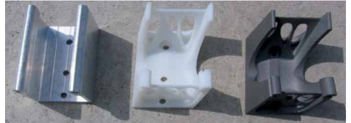
From left to right: Traditional T-Connector, polymer printed first design iteration, final design Source: Strauß (2013)
