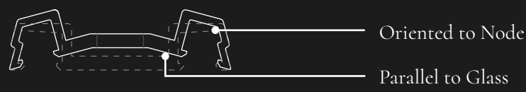
Figure 4.4.26: Section B: Concex Glazing
