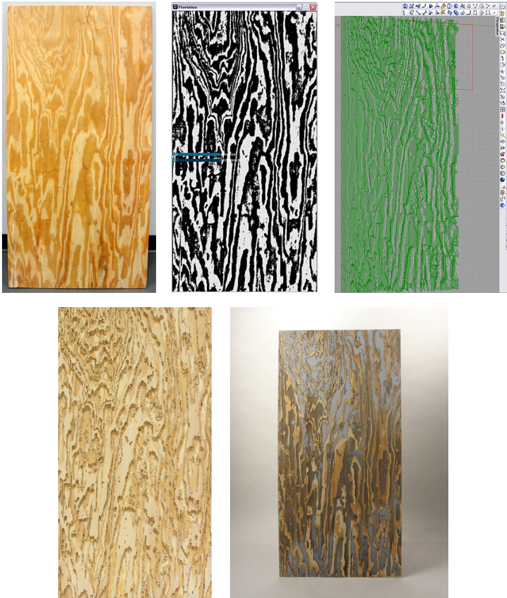
Figure 1 Digitized Grain prototype. T-B, L-R 1: original panel; 2: thresholding; 3: generated toolpath; 4: milled panel; 5: finished resin-plywood panel.
