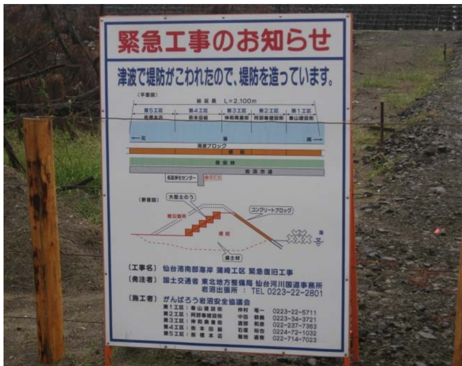
Figure 3.27: Plan for temporary retaining works, indicated in orange. The original cross section is indicated in grey.
