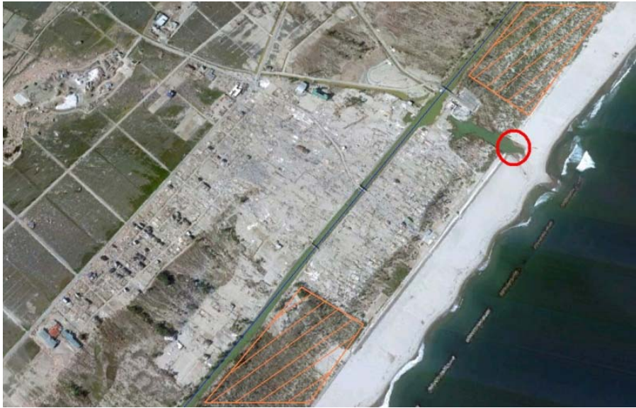
Figure 3.22: Arahama after the tsunami. The breakage on the sea dike is remarked with red, and the devastated forest zone is remarked with orange (Google earth caption, 2011)
