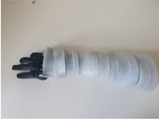
**Fig. 4.** The artificial arm is made of individual 3D-printed PLA segments covered with a silicone band combined on a steel rod.
