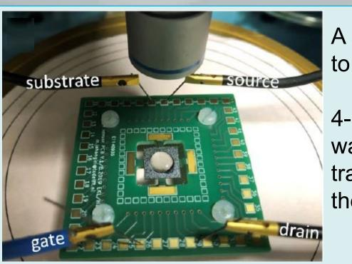
A single die wire-bonded to a custom PCB.
