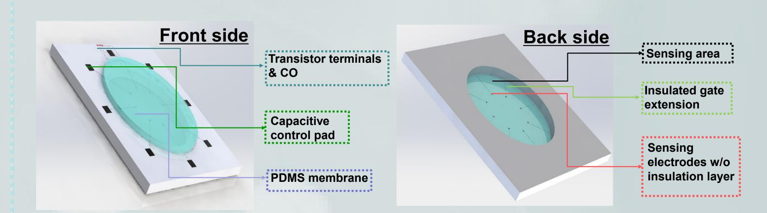
Front side: Electronic part, composed of 8 transistors.
