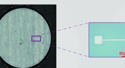
Back side of the chip after etching silicon and releasing the suspended PDMS membrane with insulated gate extensions.
