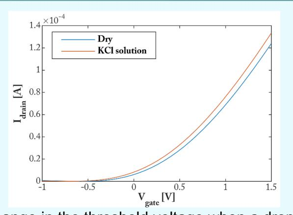
Change in the threshold voltage when a droplet of KCl solution is put on the sensing region.
