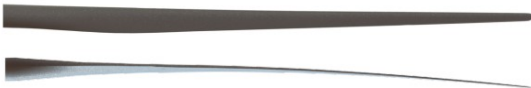
Figure B.3: View from the Suction Side (Top) and Trailing Edge (Bottom) of the Offshore Wind Turbine Blade [16]
