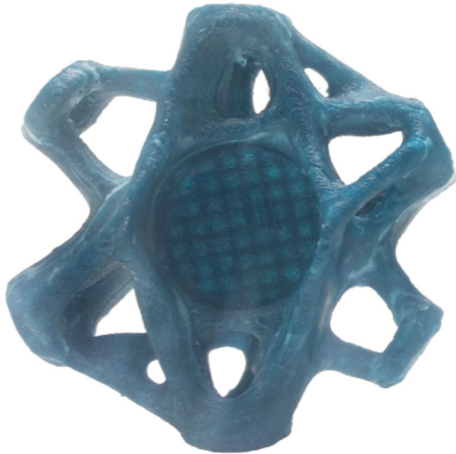
Fig. 22 FDM printed wax element
