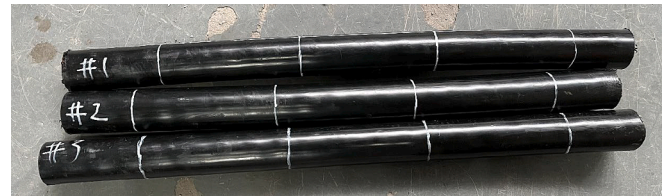
Fig. 16. Cable specimens for bending test.
