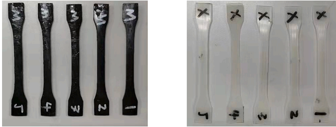
Fig. 11. Dumbbell shape of MDPE (left) & XLPE (right).
