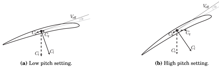
Figure 1.6: A comparison of relevant blade forces and flow velocity components acting on a propeller blade section with either a low- or a high-pitch setting during energy-harvesting conditions [13] .
