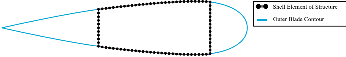
Figure 2.11: A notional diagram of the shell-element representation of a blade section with spar caps.
