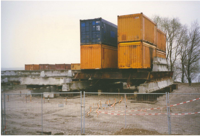
Figure 4 Test site for the Pile-tunnel interaction test
