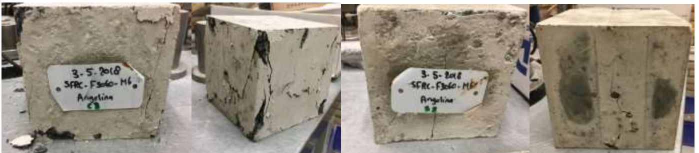
Figure 52: Failed pattern of SFRC-F3060-M specimens after compression en splitting tensile test.
