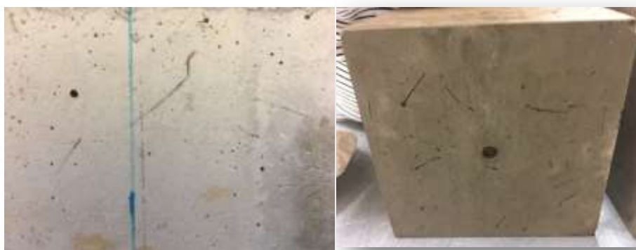
Figure 59: Examples of SFRC-F3060-M6 where short as long fibres were visible at the outer surface of the specimens.
