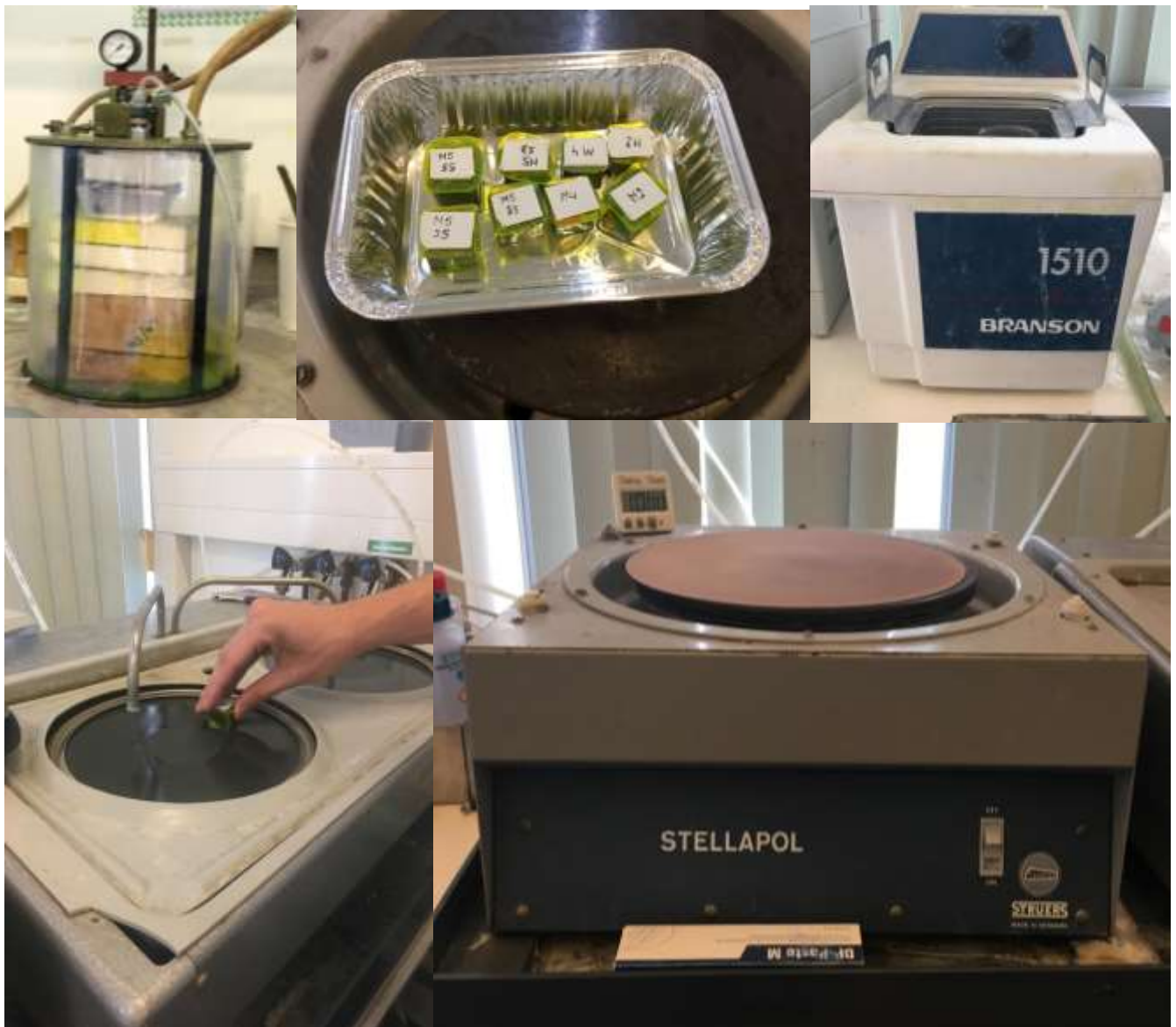
Figure 60: The apparatus used to prepare the polishes sections of reference SFRC-M2, SFRC-F-M4 and SFRC-LM-M5.
