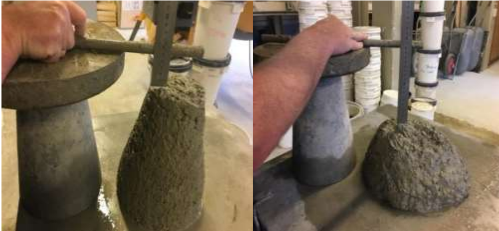
Figure 40: Slump tests of SFRC-LM-M5; trial mixture (left) and larger volume (right)).
