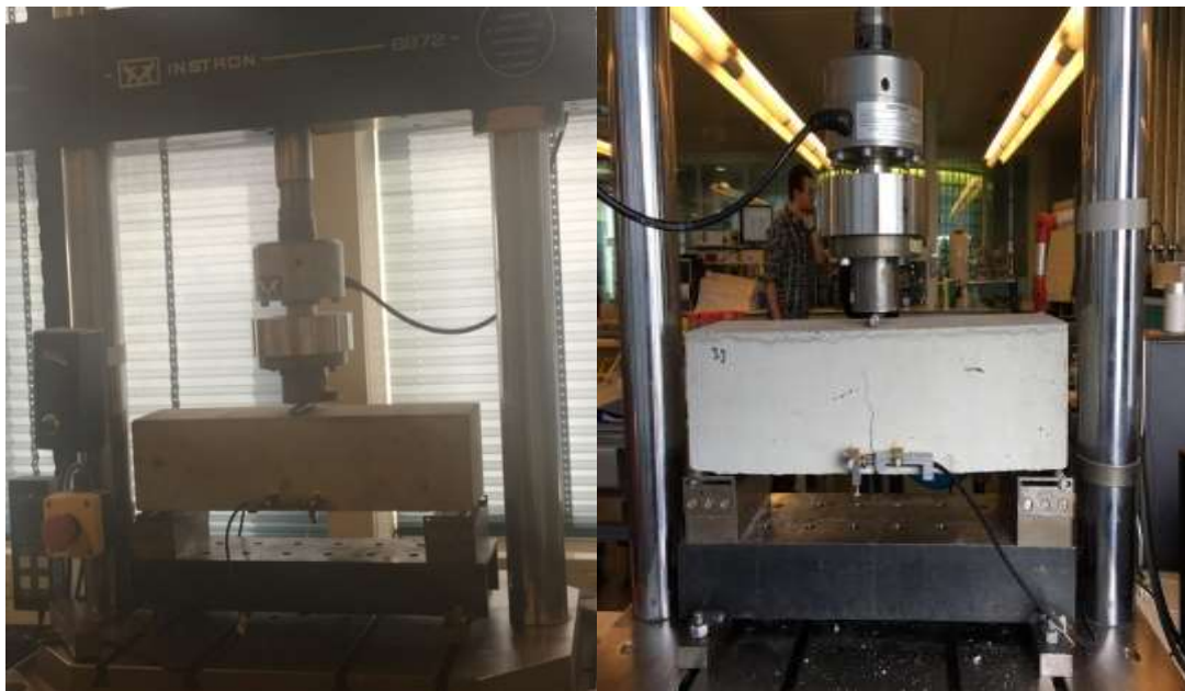
Figure 22: Left: Plain concrete and Right: SFRC prism during 3-point bending test
