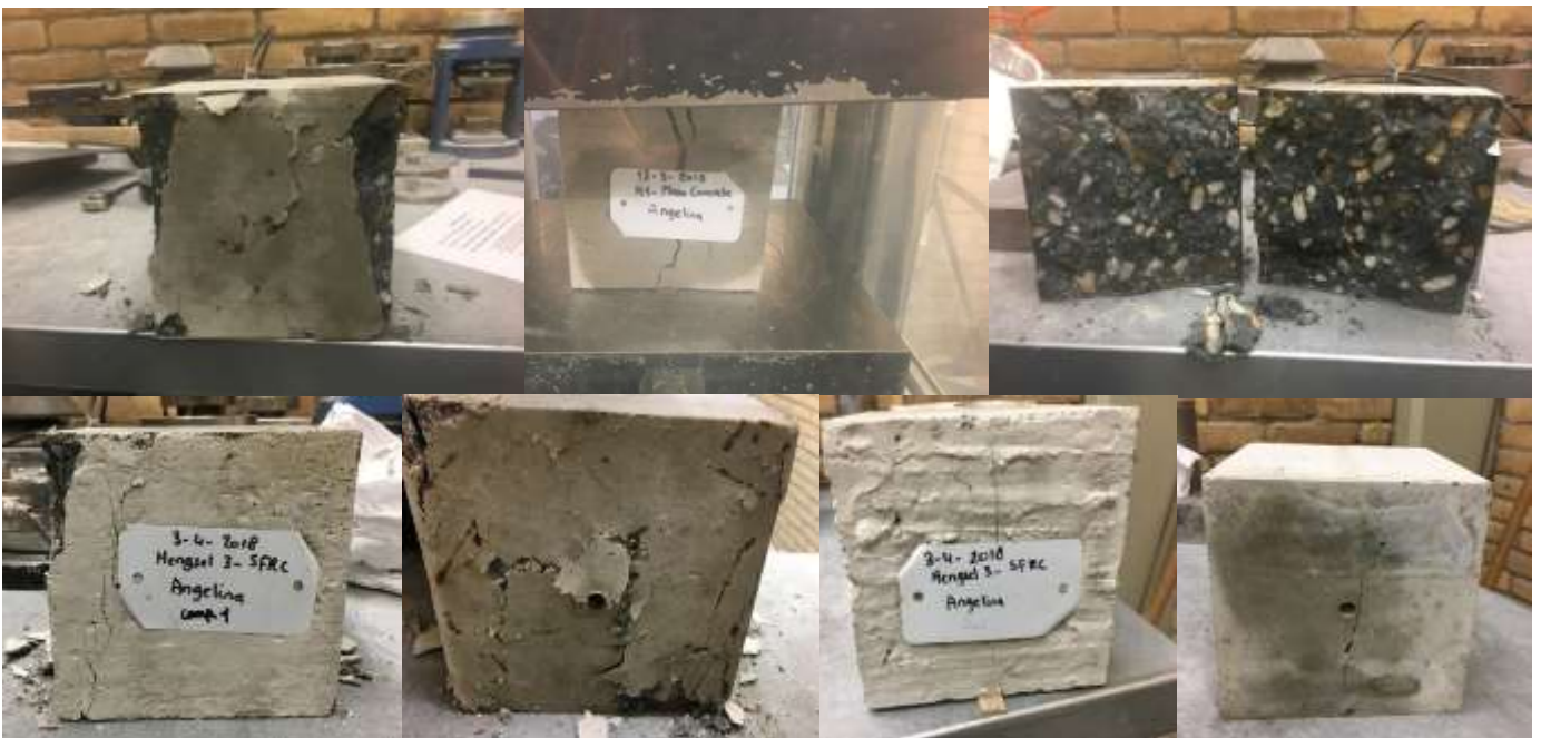
Figure 23: Top Plain concrete-M1 specimens: 1) after the compression test 2&3) after the splitting tensile strength. Below: SFRC-M2 specimens: 1&2) after the compression test 3&4) after the splitting tensile strength.
