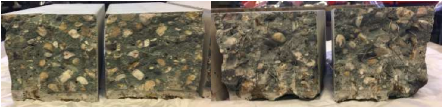
Figure 49: Left: the cross-section of the failed specimen of SFRC-LM-M5, Right: the cross-section of the strong specimen SFRC-LM-M5.
