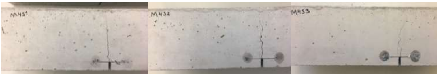
Figure 46: The crack pattern of SFRC-F-M4 specimen after the 3-point bending test.
