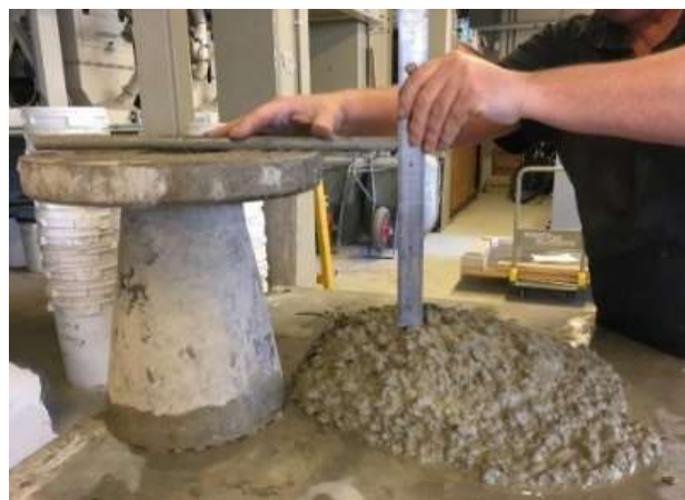
Figure 31: The slump test of SFRC-SP-M3 in phase 3.
