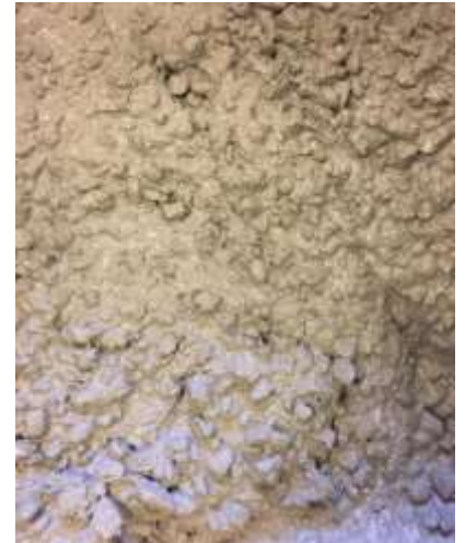
Figure 56: SFRC-F3060-M6 in the wheelbarrow before filling the molds.
