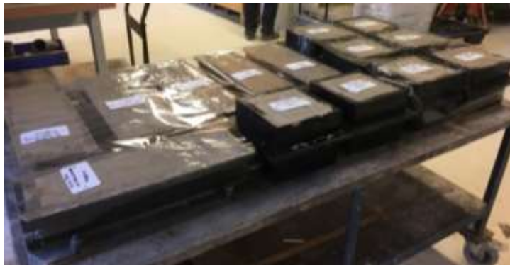
Figure 21: The cubes and prisms molds used to cast the concrete mixtures.
