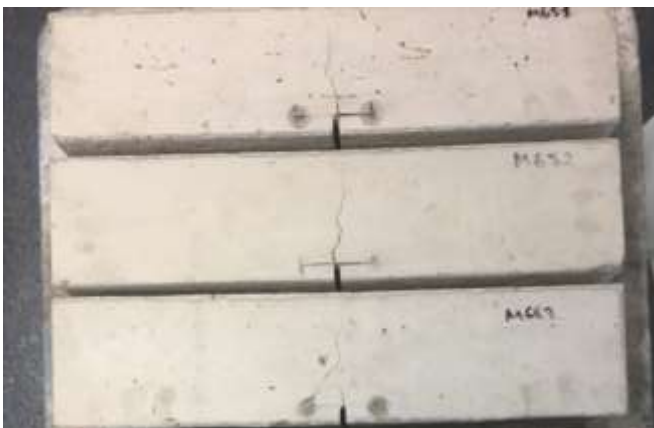
Figure 53: The crack pattern of SFRC-F3060-M6 prisms after the 3-point bending test.
