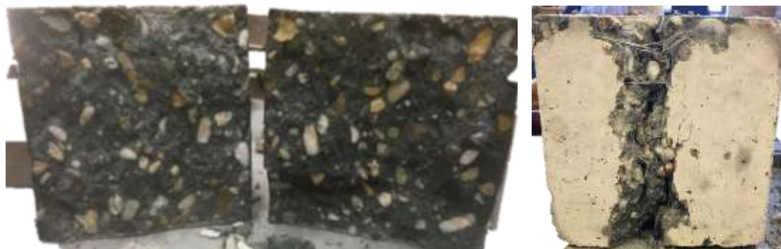
Figure 28: Comparison of cross-section specimens of plain concrete M1 (left) and reference SFRC-M2 (right)
