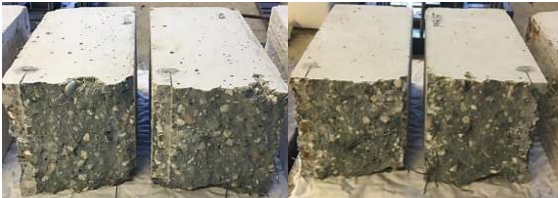
Figure 48: Left: The cross-section of specimen 4, Right: cross-section of specimen 5 of SFRC-F-M4.
