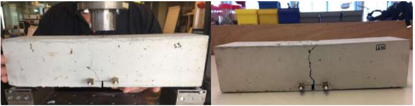
Figure 29: a) Left: partly cracked specimen of SFRC-M2 b) Right: completely cracked specimen (s4).
