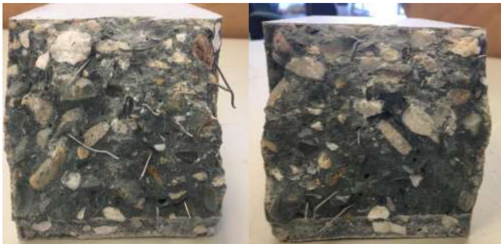
Figure 30: Specimen 4 of mixture SFRC-M2 after breaking it by hammer.
