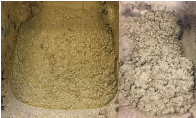
Figure 45: SFRC-F-M4 (left) and trial mixture of SFRC-LM-M5 (right) in fresh state.
