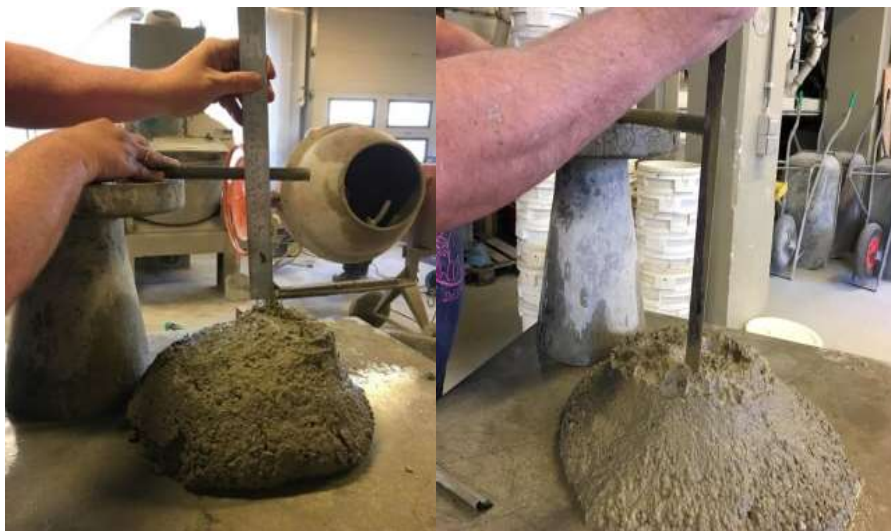
Figure 39: Slump tests of SFRC-M4; trial mixture (left) and larger volume (right).
