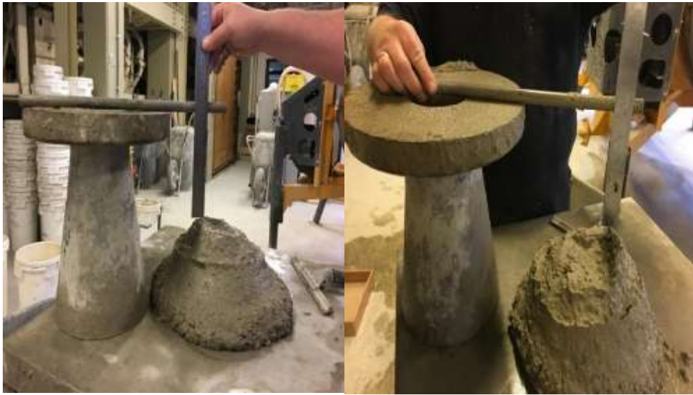
Figure 20: The measured slump of plain concrete-M1 (left) & SFRC-M2 (right).
