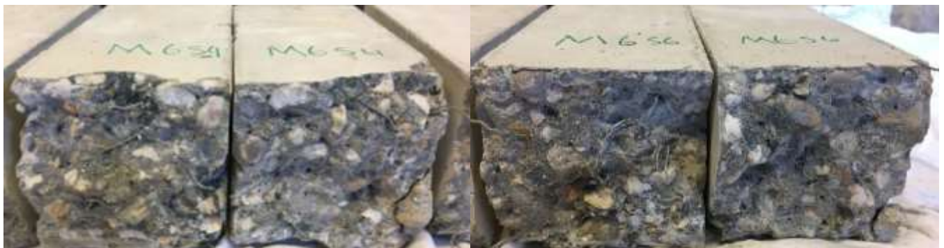
Figure 57: Comparison between the cross-section of specimen 4 and specimen 6.
