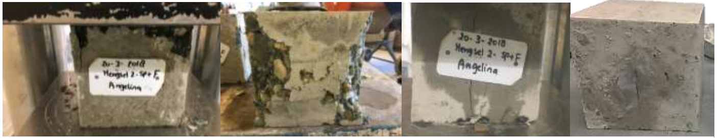
Figure 32: SFRC-SP-M3 specimens: 1&2) after the compression test 3&4) after the splitting tensile strength.
