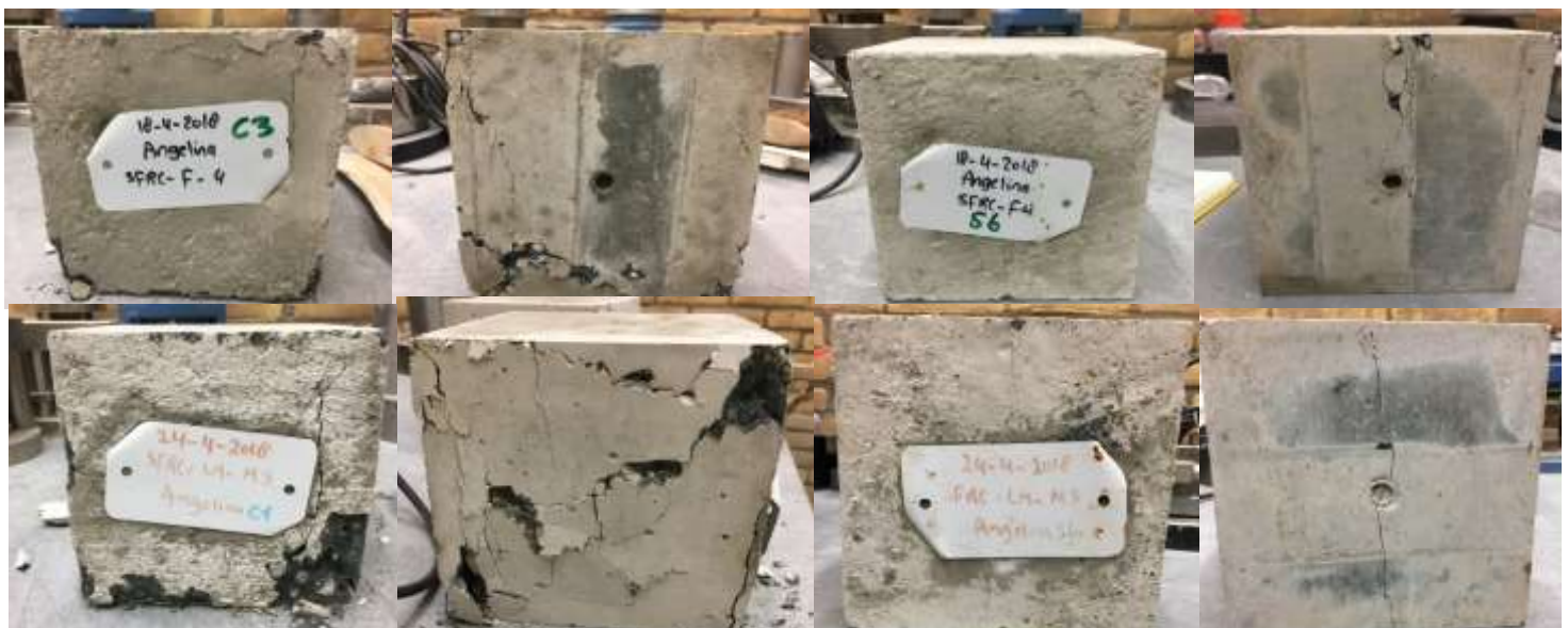
Figure 41: Top: SFRC-F-M4 specimens: 1&2) after the compression test 3&4) after the splitting tensile strength. Below: SFRC-LM-M5 specimens: 1&2) after the compression test 3&4) after the splitting tensile strength.
