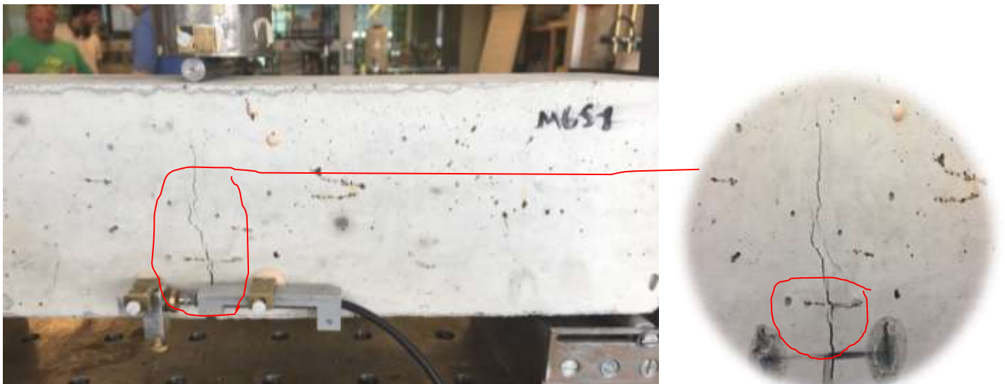
Figure 58: Crack pattern of SFRC-F3060-M6 specimen during 3-point bending test, where the first crack initiates above the notch that was hindered by fibres, hence another crack appeared above and went through the fibre.
