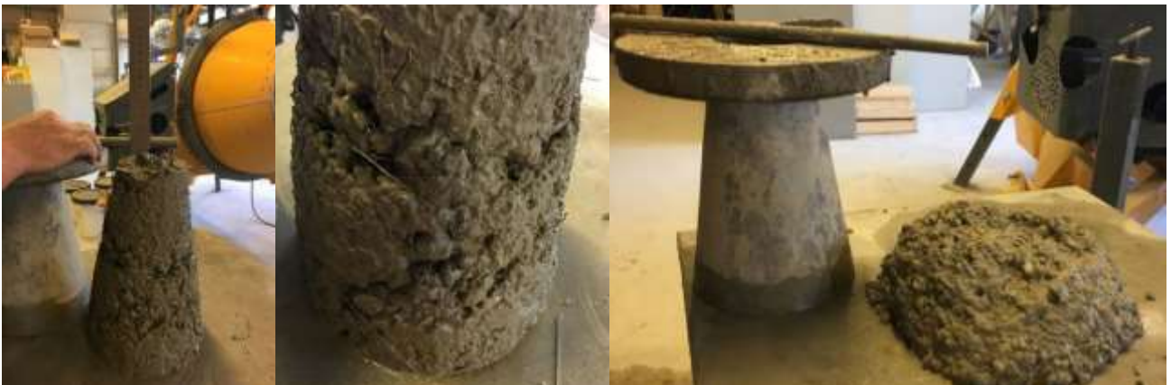
Figure 51: Left: Slump test of SFRC-LM-M6 trial mixture and a close-up on the gaps in the slump, Right: the slump of the larger volume after adding SP.
