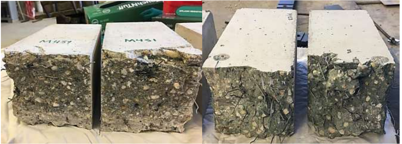
Figure 47: Left: the cross-section of specimen 1, Right: cross-section of specimen 3 of SFRC-F-M4.
