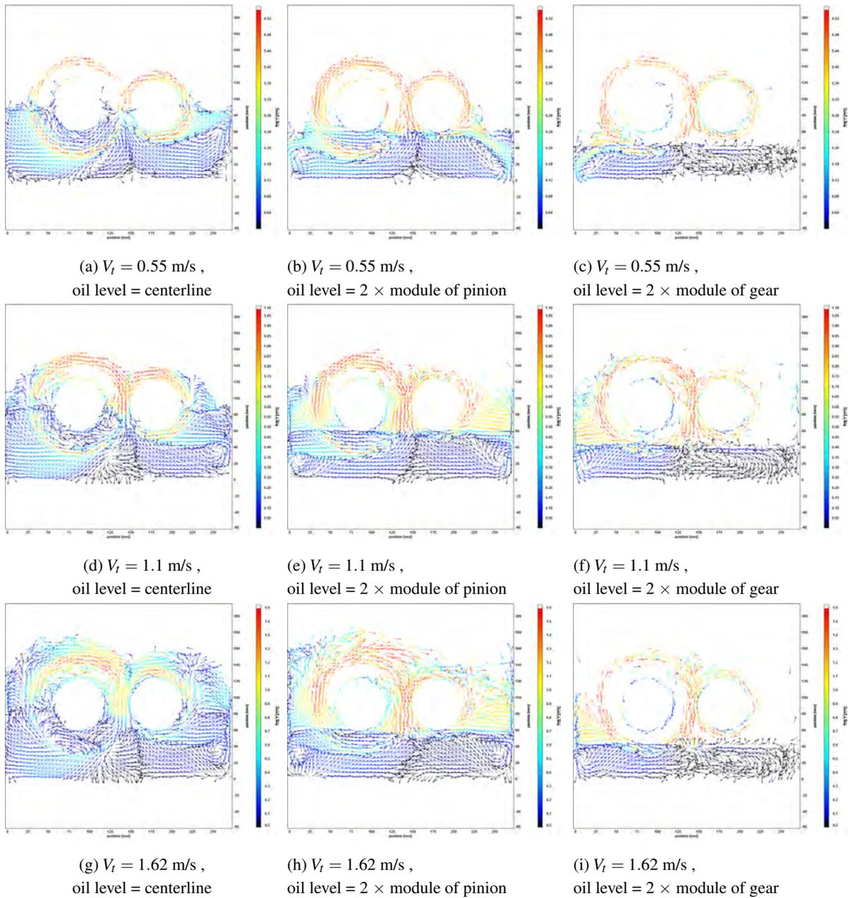
**Figure 8:** Overall mean velocity vector fields. Oil temperature at 20°C
