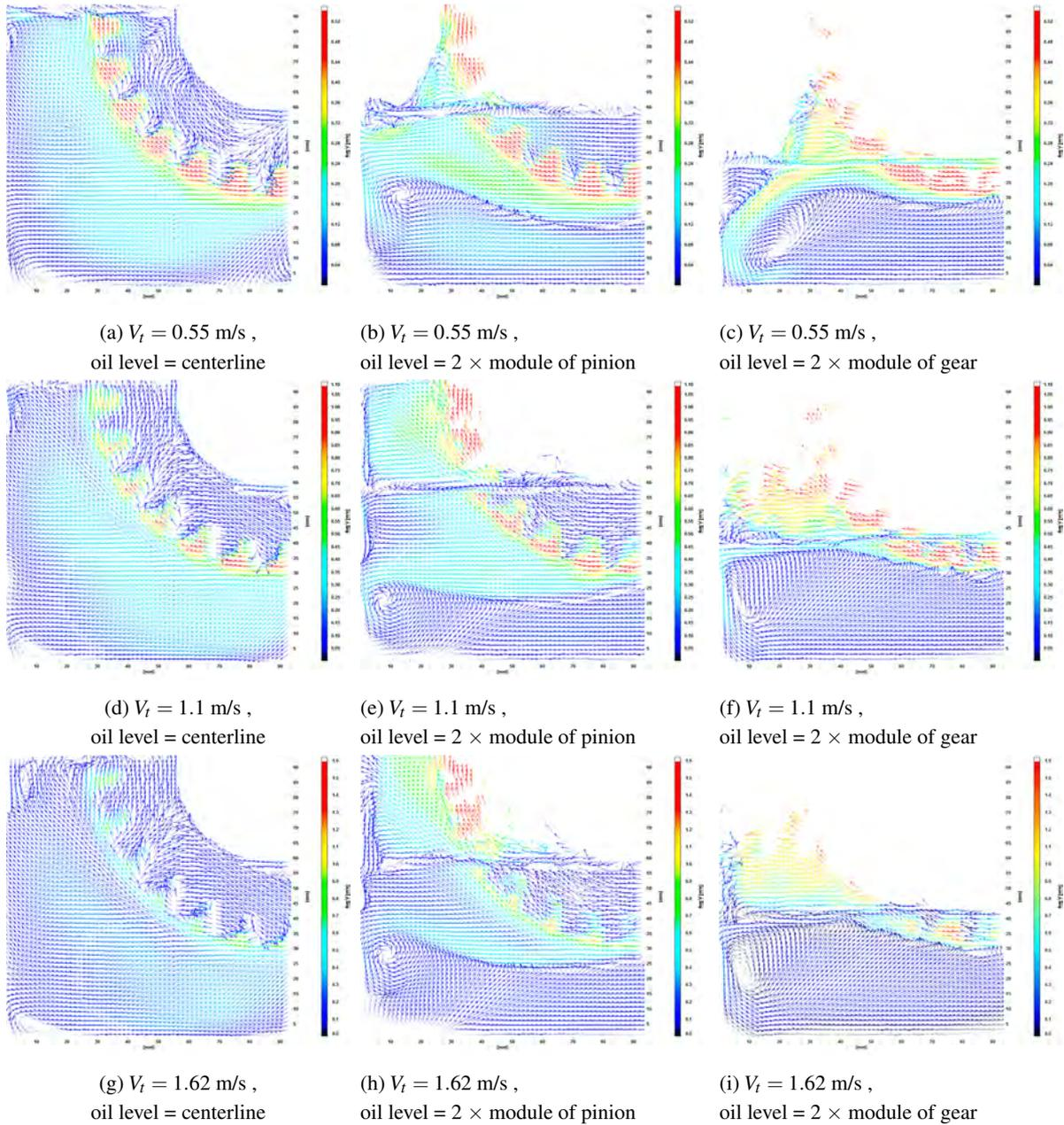
**Figure 9:** Mean velocity vector field close to the gear. Oil temperature at  $20^\circ\text{C}$
