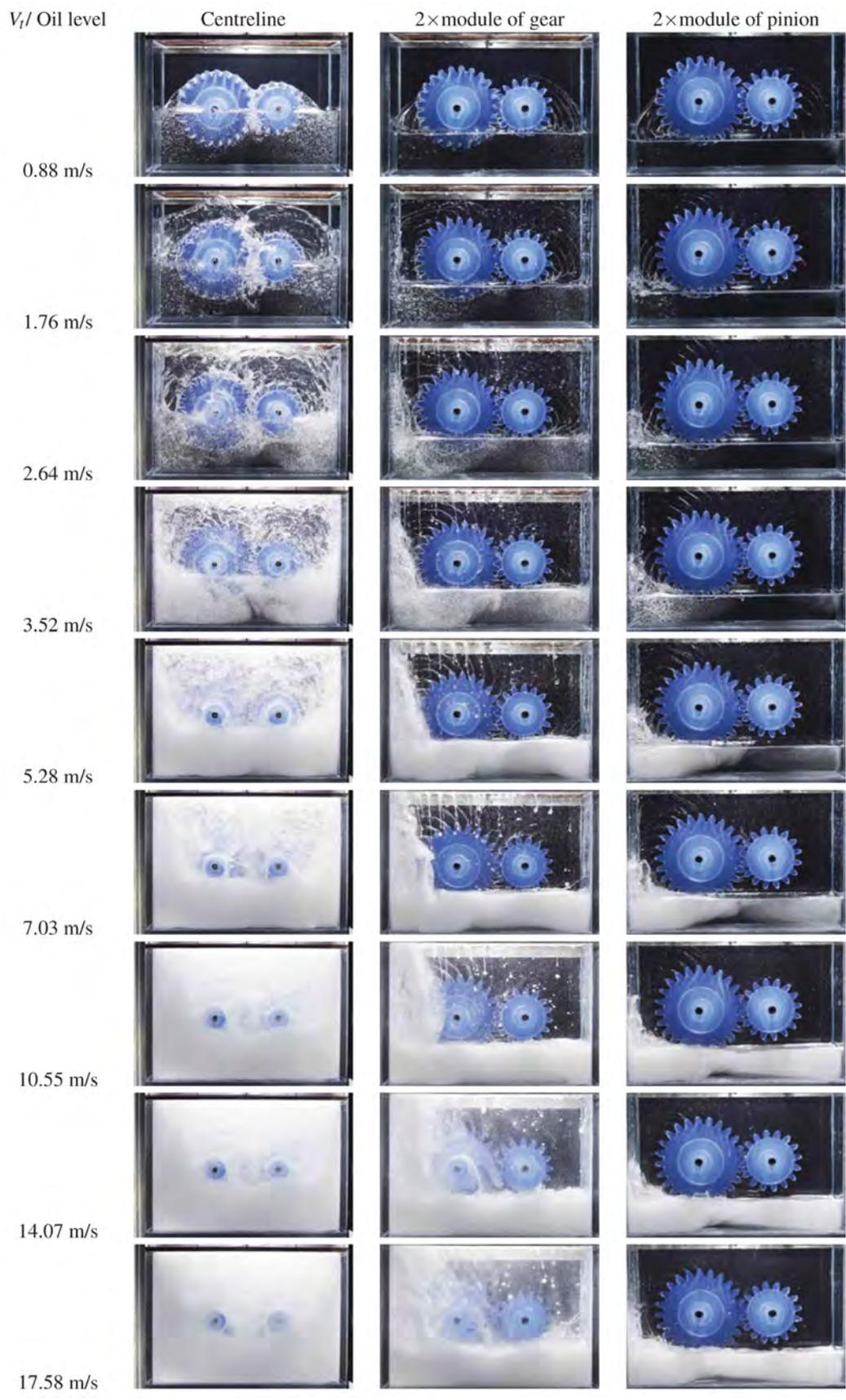
**Figure 4:** Collection of instantaneous image of oil flow inside a gearbox at room temperature
