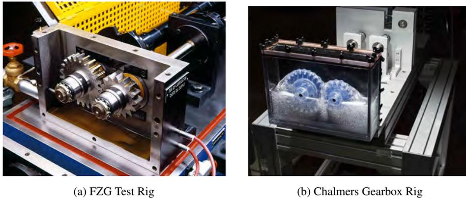
**Figure 1:** Comparison between the FZG gear test rig and the Chalmers gearbox rig
