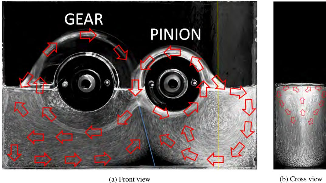
**Figure 3:** Flow Visualization of test oil at 20°C,  $V_t = 0.35$  m/s. Blue line emphasizes two separate regions created by the rotation of the gear and the pinion. Yellow line indicates the cross sectional region. Red arrows indicate the flow direction.
