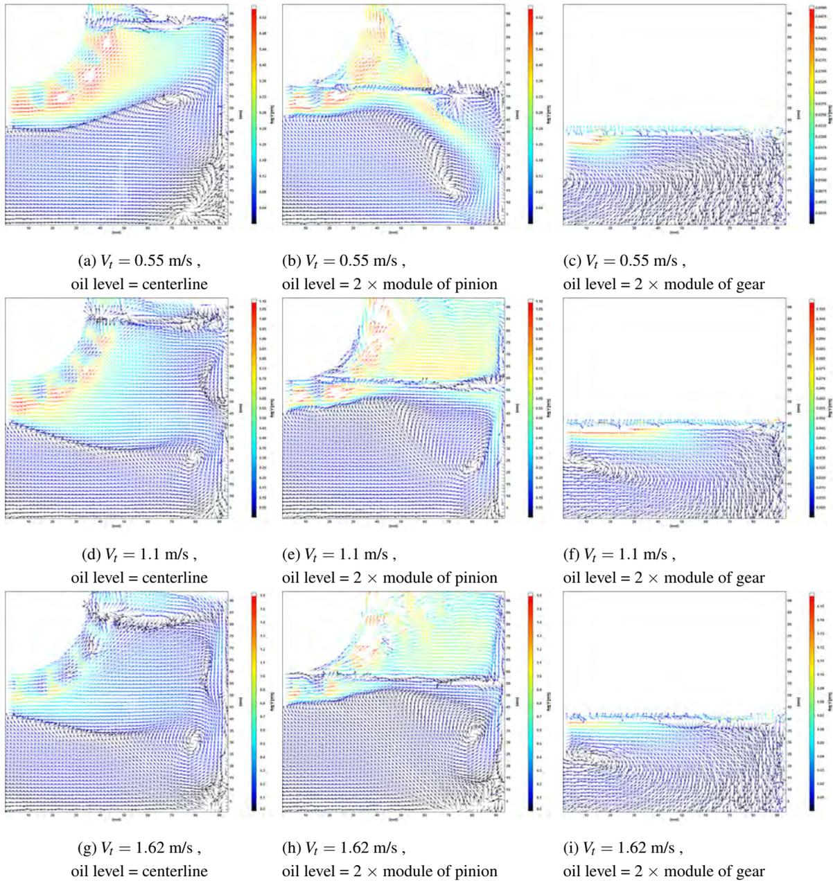
**Figure 10:** Mean velocity vector field close to the pinion. Oil temperature at  $20^\circ\text{C}$ . Note that for oil level  $2 \times$  module of gear, the pinion do not touch the oil bath.
