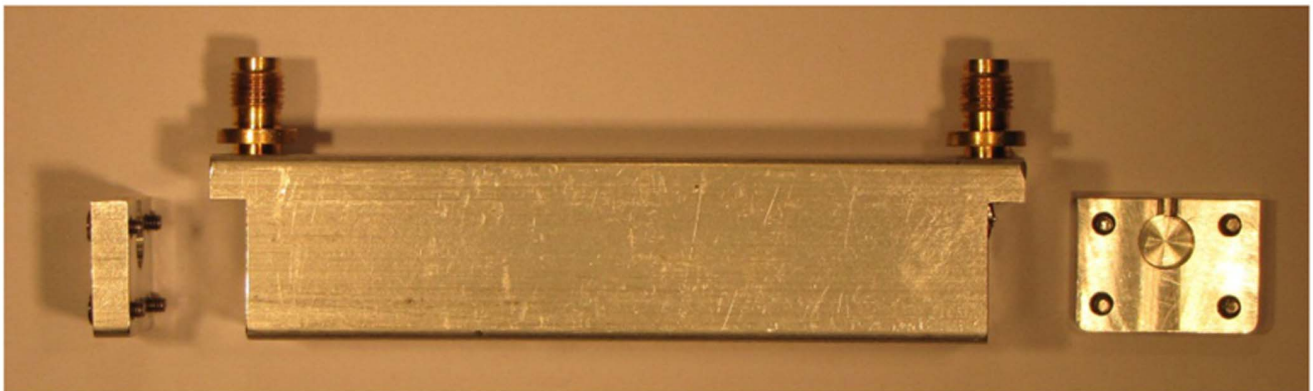
Figure 5. Picture of a monolithic aluminum cell. With its perpendicular SMA connectors this 82 mm inner length construct is the longest possible cell allowing TEM || B operation in our wide-gap magnet. doi:10.1371/journal.pone.0059874.g005
