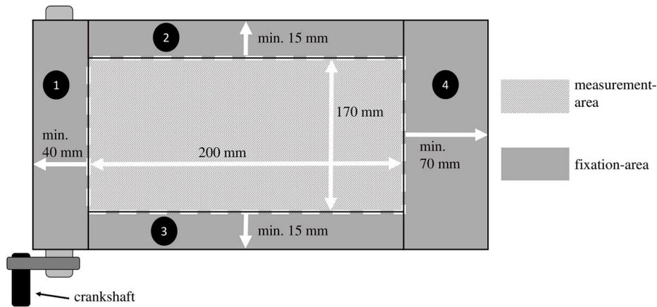
Fig. 4. Geometrical guidelines for the cover sample.
