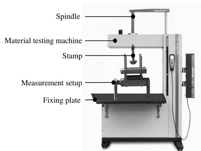
Fig. 1. Elements of the measurement tool.
