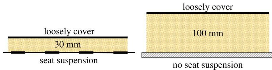
Fig. 6. Two different seat layouts (No. 5 and No. 10) are shown with nearly the same pressure distribution and maximum pressure but with a 1.5-fold higher elongation for the seat-layout with 100 mm foam. The left seat layout (No. 10) has a loosely cover, a 30 mm high and 12 kPa hard foam and contains a seat suspension. The right seat layout (No. 5) has a loosely cover, 100 mm high and 4 kPa soft foam without a seat suspension.
