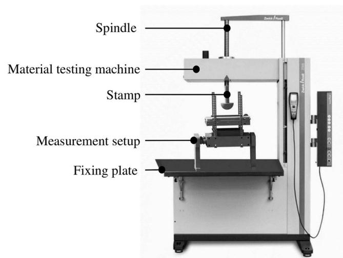
Fig. 1. Elements of the measurement tool.
