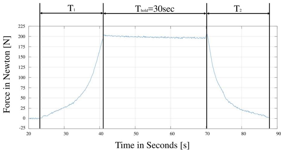
Fig. 5. Prescribed force curve for the measurement cycles (without pre-cycles).
