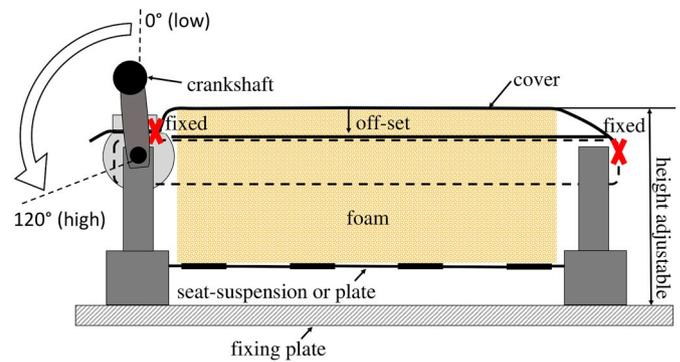
Fig. 2. Schematic measurement setup, including the cover fixation, the foam, the seat suspension or plate as well as the cover height adjustment for various foams.
