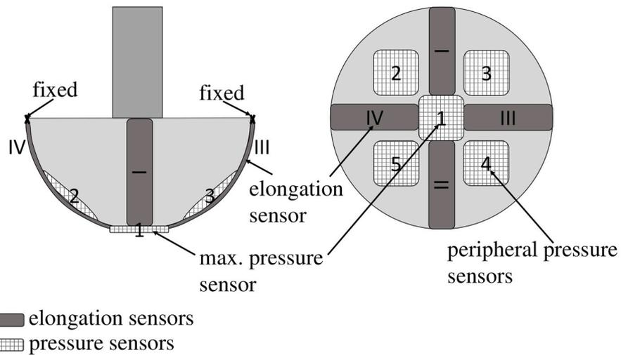
Fig. 3. Overview of the pressure and elongation sensors location.
