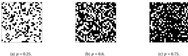
Figure 2.3: Bernoulli percolation with occupation probability p on a 30 \times 30 lattice. The black squares are occupied sites, the white squares are unoccupied sites. Underneath each figure, the used value of p is specified.
