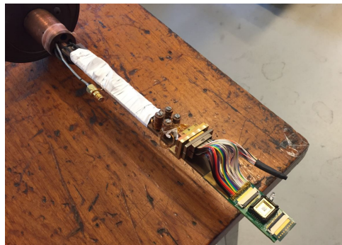
Figure 3.10: PCB board mounted on the end of the dipstick for tests at 4 K
