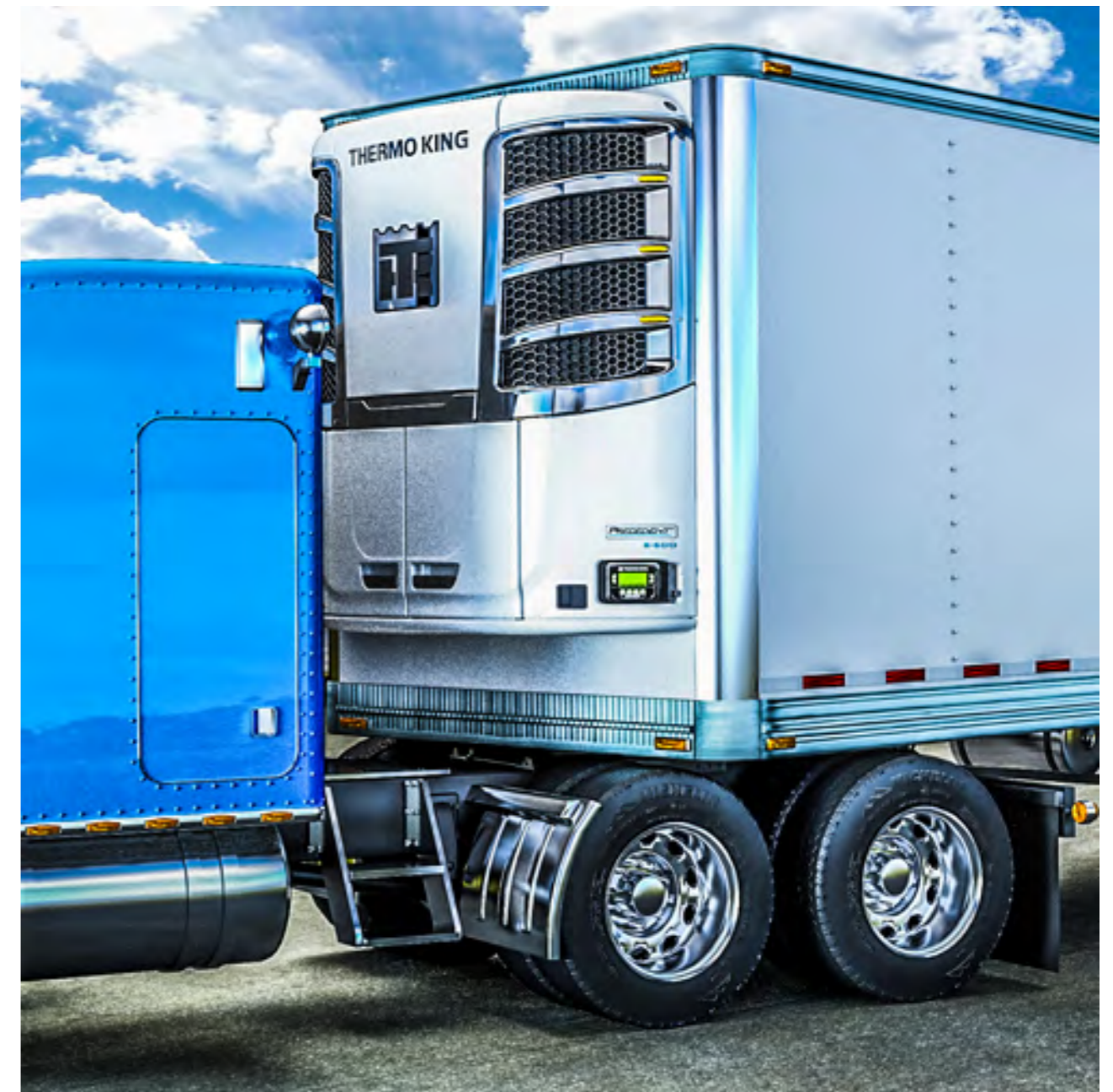
Fig.16: Cooling unit on trailer
