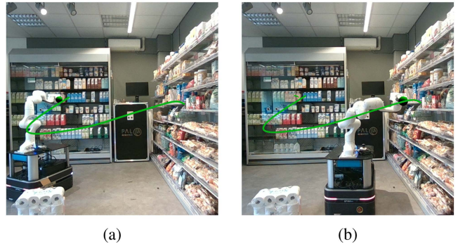
Fig. 1. DF for path (green) following with a nonholonomic mobile manipulator. DF control all actuators simultaneously to follow the end-effector path while keeping a given orientation and avoiding collision with the environment.
