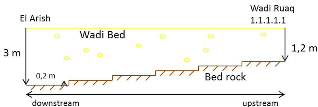
Figure 4.6 Simplification of the wadi bed thickness in the El Arish watershed (own illustration, 2017)
