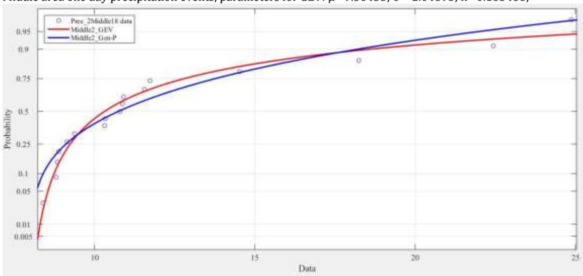
Middle area two days precipitation events, parameters for GEV:  $\mu = 10.3326$ ;  $\sigma = 1.51493$ ;  $k = 0.652081$ ;
