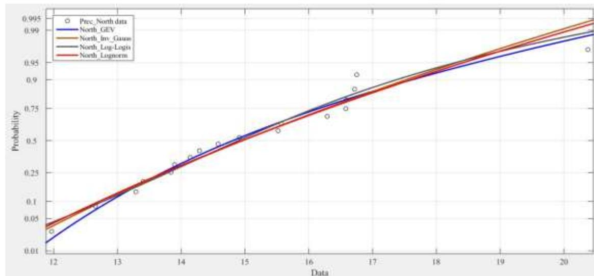
North area one day precipitation events, parameters for GEV:  $\mu= 17.9345$ ;  $\sigma= 2.00568$ ;  $k= 0.05$ ;
