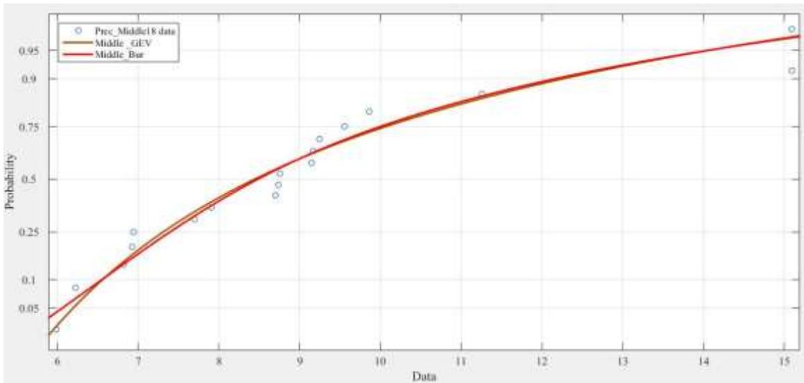
Middle area one day precipitation events, parameters for GEV:  $\mu= 9.86455$ ;  $\sigma = 2.04895$ ;  $k= 0.165488$ ;
