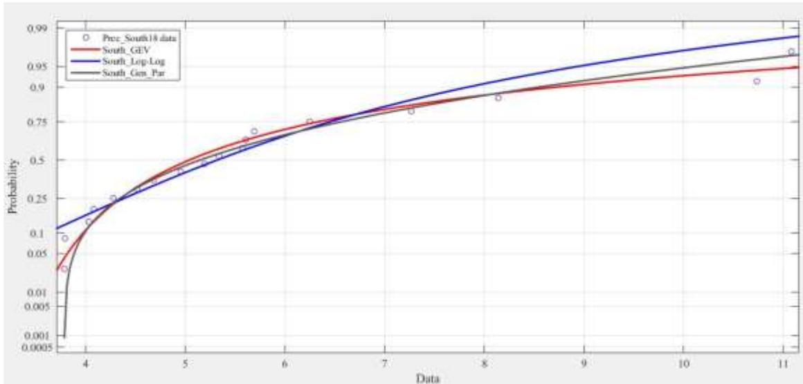
South area one day precipitation events, parameters for GEV:  $\mu = 5.85416$ ;  $\sigma = 1.23711$ ;  $k = 0.497289$ ;
