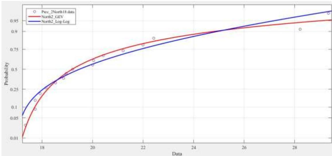
North area two days precipitation events, parameters for GEV:  $\mu= 19.8955$ ;  $\sigma= 1.47462$ ;  $k= 0.556684$ ;
