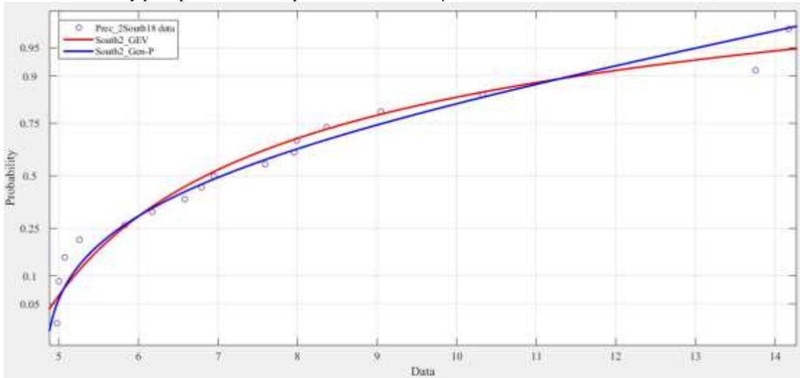
South area two days precipitation events, parameters for GEV:  $\mu = 6.68105$ ;  $\sigma = 1.68481$ ;  $k = 0.477008$ ;
