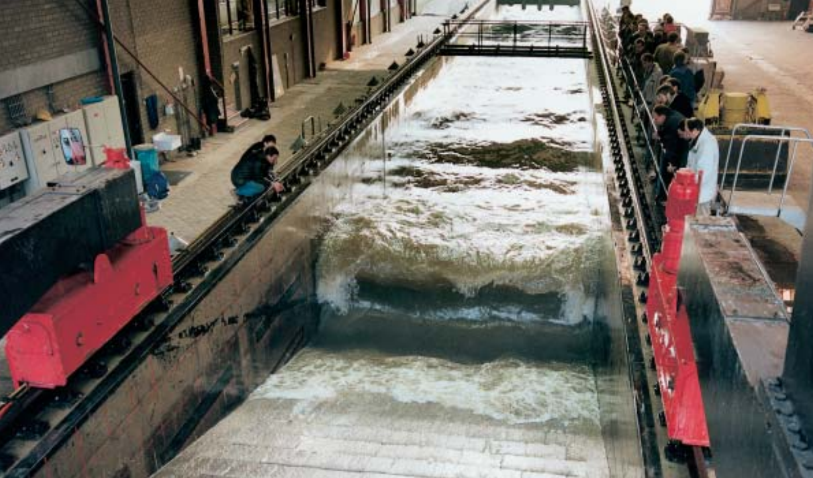
Figure 6. Fundamental research project on the stability of placed block revetments at prototype scale in the large wave flume (Delta flume) of WL Delft Hydraulics (1992).
