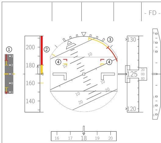
Figure 4.4: Wireframe view of the Airbus A320 PFD with additional load factor indicator ① and flight envelope limits for airspeed ②, bank angle ③ and angle of attack ④
