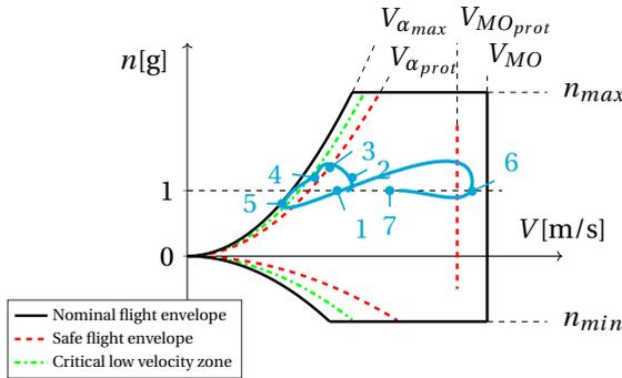
Figure 2.16: Trajectory through the flight envelope during windshear recovery with frames indicated in Fig. 2.15
