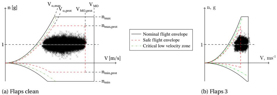
Figure 4.1: Typical flight envelopes with velocity ( $V$ ) versus load factor ( $n$ ); [97] augmented with load factor data for 10,066 A320 flights; [98] the actual envelopes depend on the aircraft's configuration and loading
