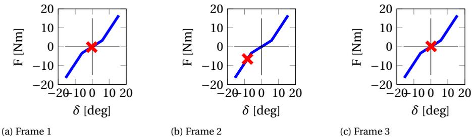
Figure 7.16: Haptic profiles for frames indicated in Fig. 7.15, cross indicates the current state
