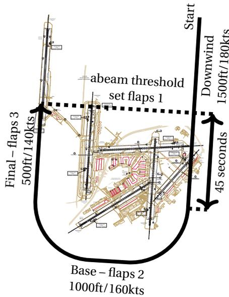
Figure 6.9: Traffic pattern flown to runway 36L at Schiphol (Schiphol layout from AIP [84])
