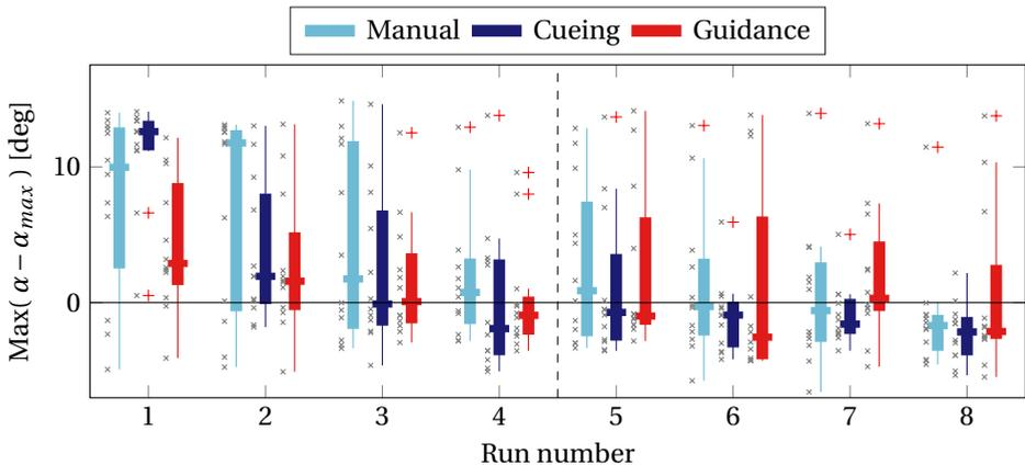
Figure 7.21: Highest angle of attack obtained during the windshear, relative to the maximum angle of attack (positive values result in a stall warning)
