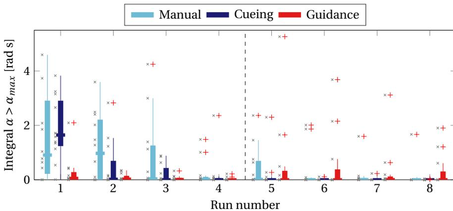
Figure 7.22: Integral above angle of attack limit during windshear (Manual Participant 7, 8.45rad s, not shown)
