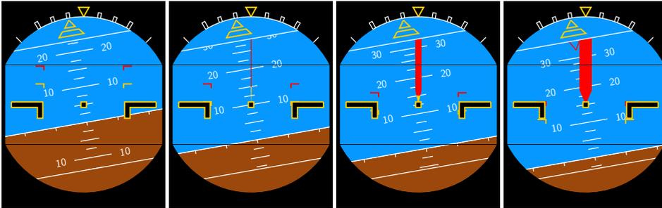
Figure 4.6: AoA indicators relative to the fixed aircraft symbol progressively reaching the AoA limit
