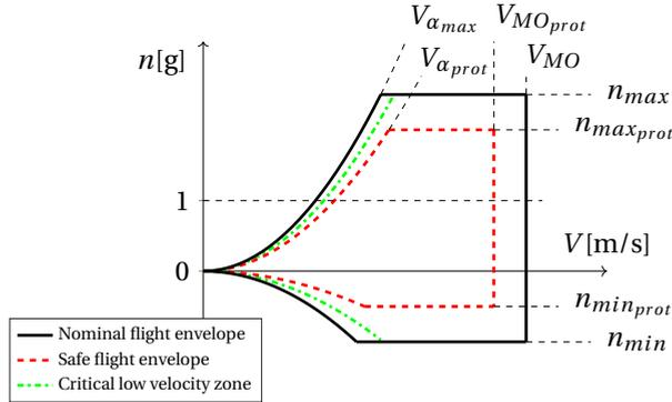
Figure 3.2: Flight envelope, load factor ( $n$ ) versus velocity ( $V$ )
