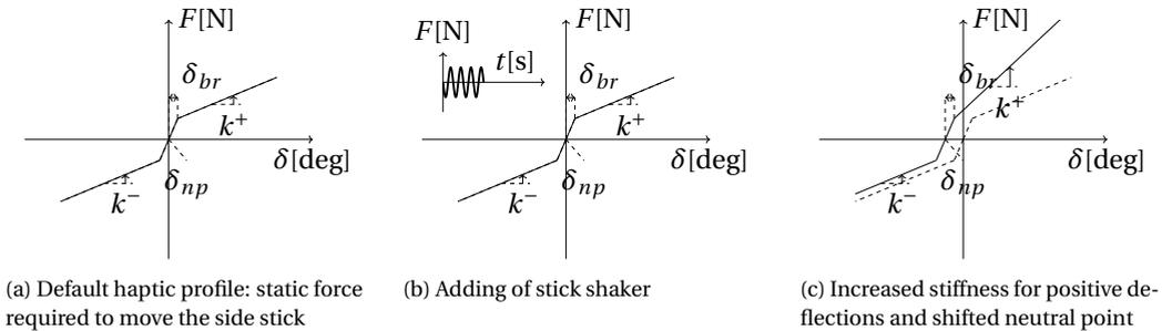
Figure 1.5: Haptic Profile: static force required to move the side stick
