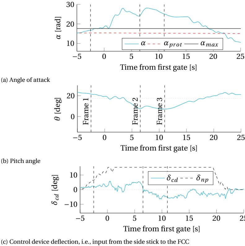
Figure 7.17: Time traces of the design flaw which occurred during Run 1 of Guidance Participant 5
