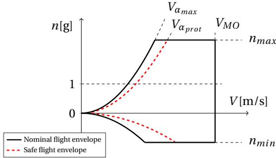
Figure 2.6: Flight envelope with A320 longitudinal Flight Envelope Protection limits indicated
