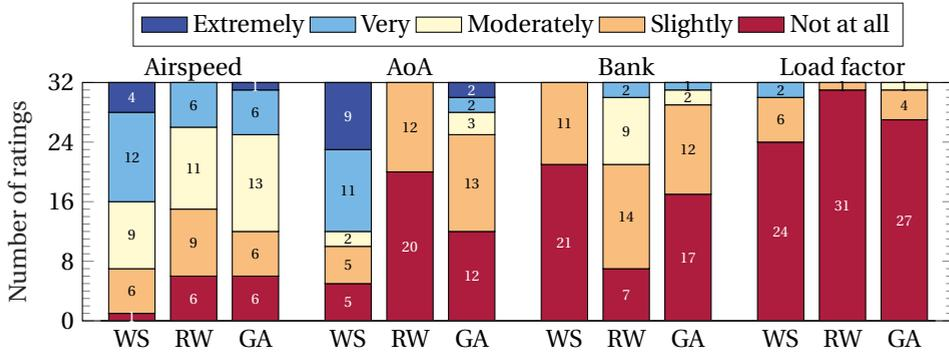
Figure 4.27: Subjective usefulness ratings of display elements in helping to stay inside the flight envelope limits
