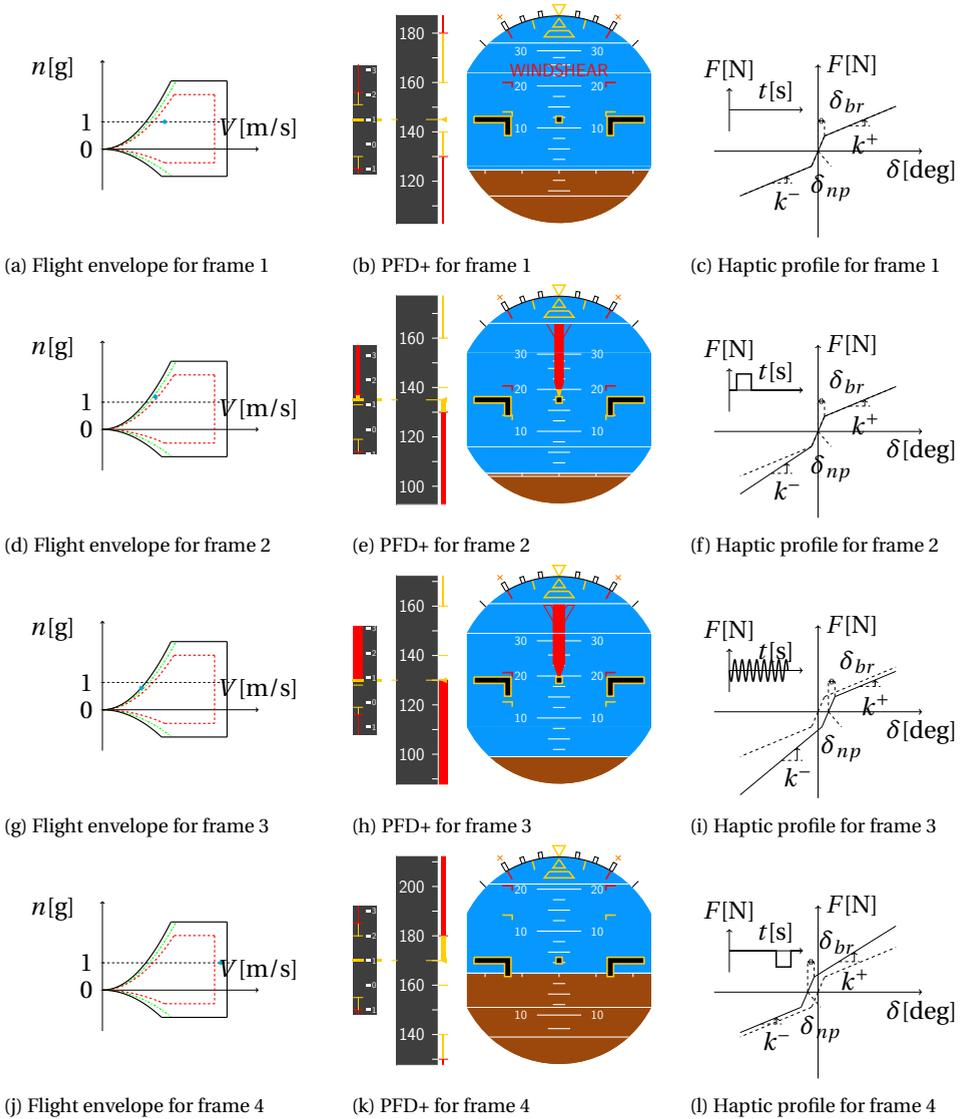
Figure 4.7: Typical windshear recovery procedure. The left column shows the flight envelope, the center column shows an excerpt of the PFD and the right column shows the associated haptic pitch profile
