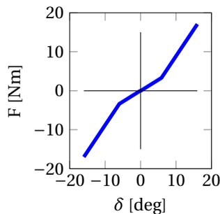
Figure 7.2: Default haptic profile in the cueing design, i.e., force required on the side stick for a given deflection
