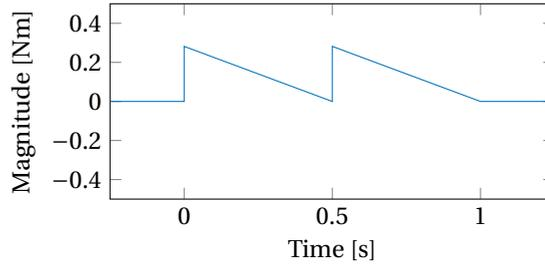
Figure 6.2: Sawtooth-shaped forcing function used
