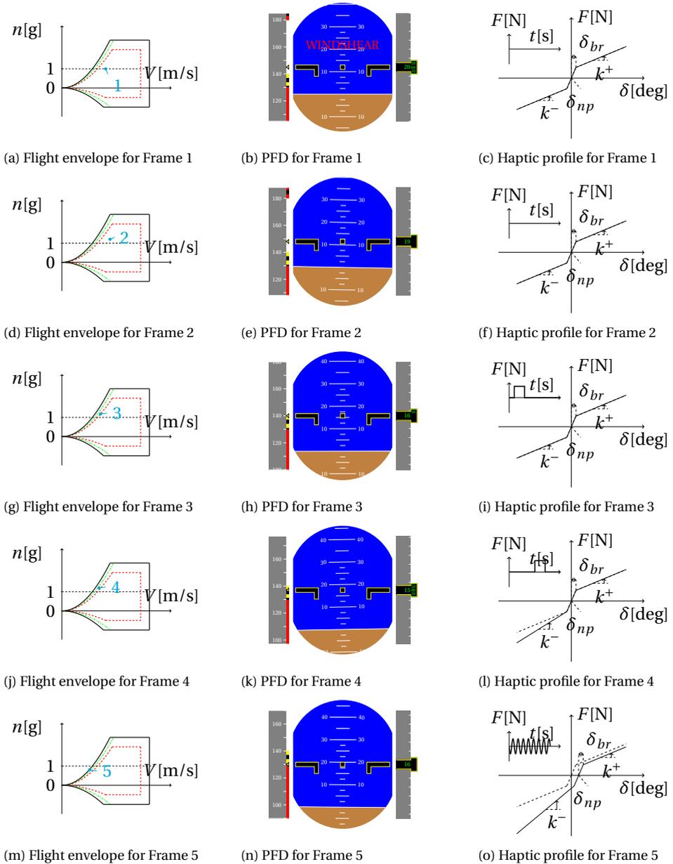
Figure 2.17: Flight envelopes, PFDs, and haptic profiles for the windshear recovery according to the frames from Fig. 2.15
