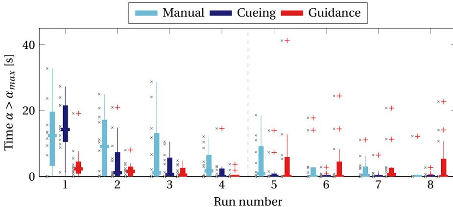
Figure 7.20: Time with angle of attack above limit during windshear (Manual Participant 7, 61.7s, not shown)
