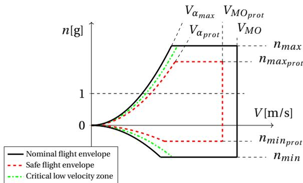
Figure 1.1: Flight Envelope: allowable load factor versus velocity
