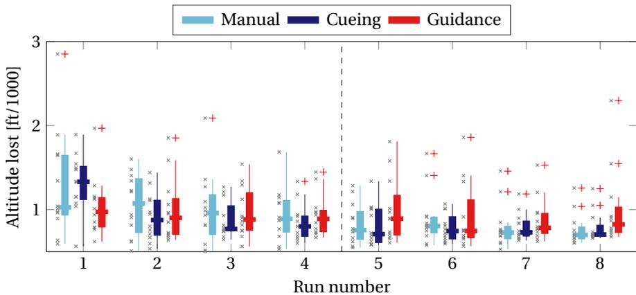
Figure 7.19: Altitude lost during windshear recovery
