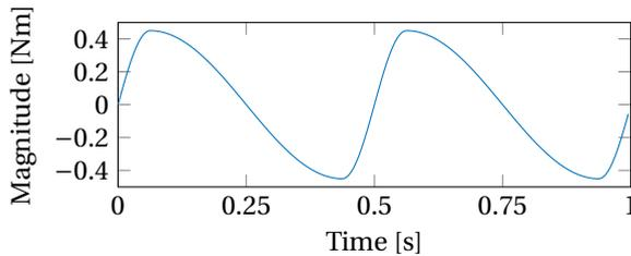
(a) Asymmetric-in-*time* and symmetric-in-*amplitude* vibration [109]
