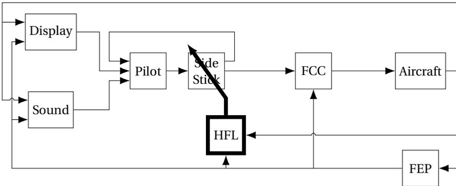
Figure 1.2: Pilot-aircraft control loop, combined with the haptic feedback as presented in this thesis in thick
