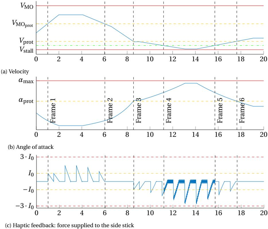
Figure 6.3: Illustrative example of haptic feedback triggering on changing states
