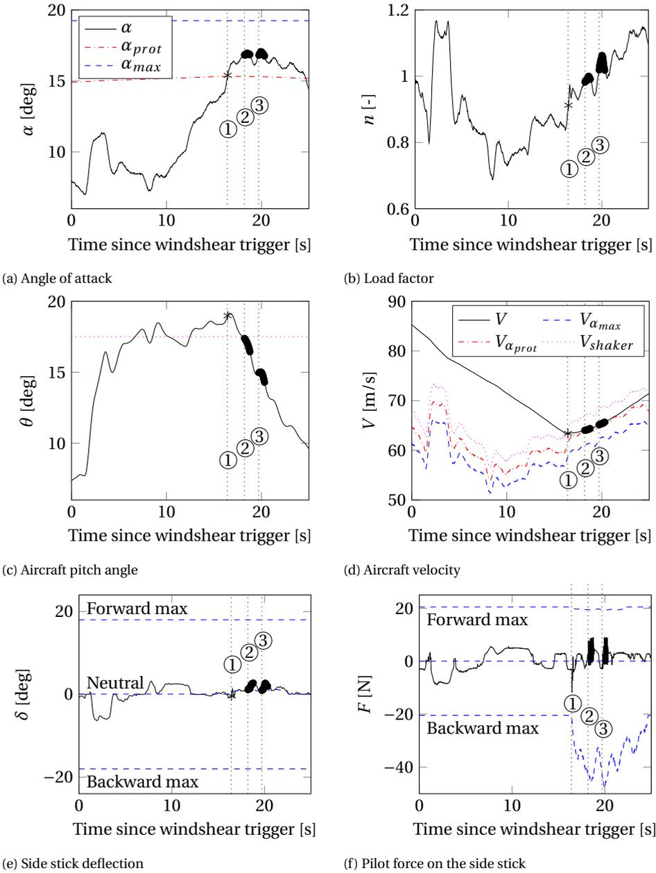
Figure 3.9: Time traces for Participant 3 in condition WSALHF, thrust was set to full after 6.4s
