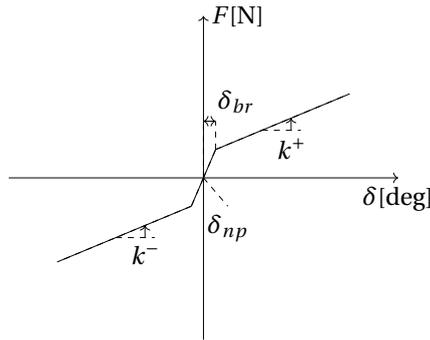
Figure 2.7: Nominal control device profile: required force exerted ( $F$ ) versus stick deflection ( $\delta$ )
