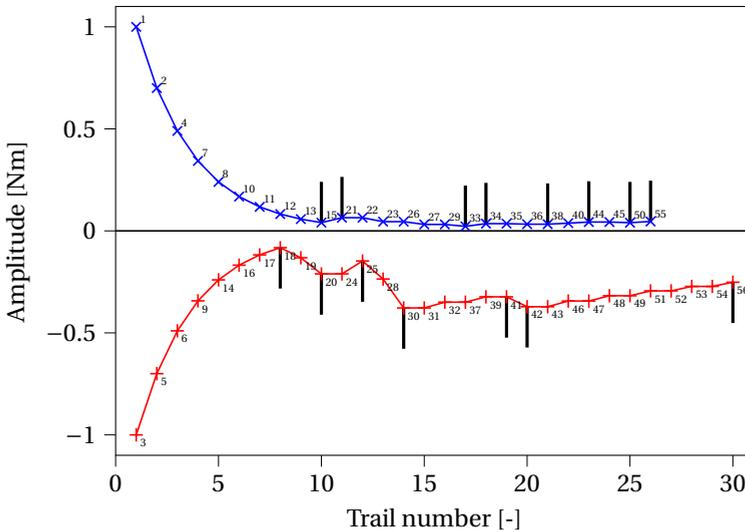
Figure 5.7: Example staircase-procedure (Participant 3), when applying a backward force on the stick and using a triangular pulse; numbers next to the points indicate the trials' sequence, vertical lines indicate reversals
