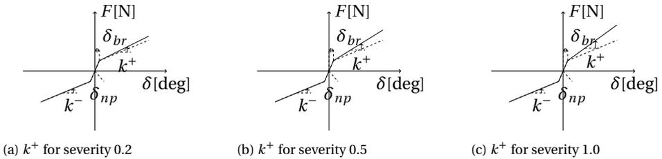
Figure 2.14: Haptic profiles showing progressively increasing positive spring stiffness ( $k$ )
