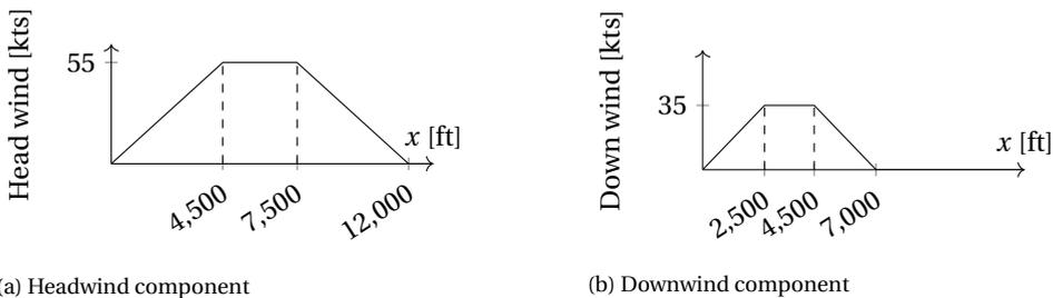
Figure 3.6: Windshear component distribution
