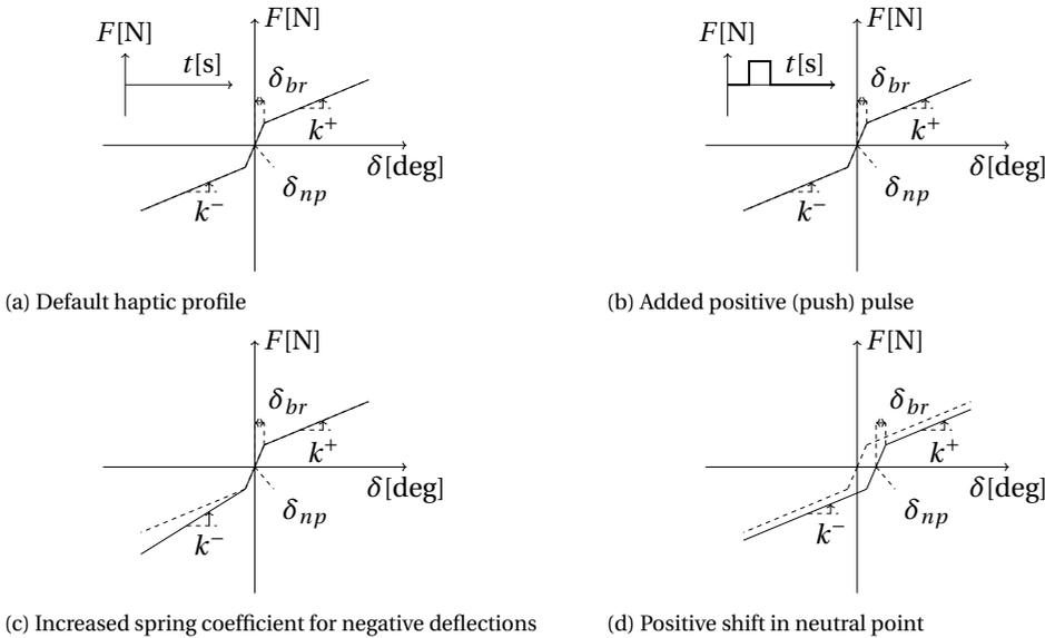
Figure 4.2: Control device profiles
