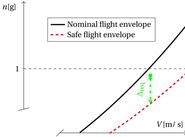
Figure 2.11: The amount of load factor change required when flying at low velocities, inset from Fig. 2.9
