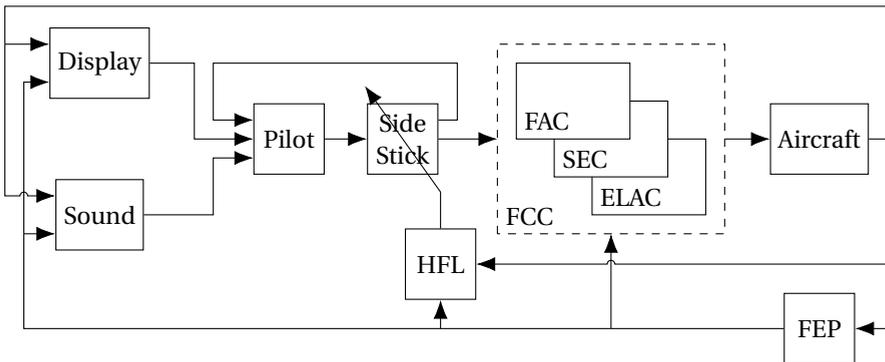
Figure 2.8: Block diagram representing the Airbus control loop combined with the Haptic Feedback Law (HFL)
