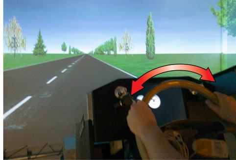
Figure 1.3: Example of haptic feedback applied to the steering wheel of a car in the HMI simulator at TU Delft
