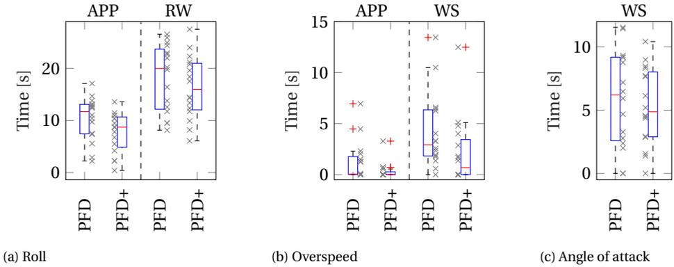
Figure 4.20: Mean times in protection per pilot; flight phases in which one or zero excursions into the protection limits were registered are not shown
