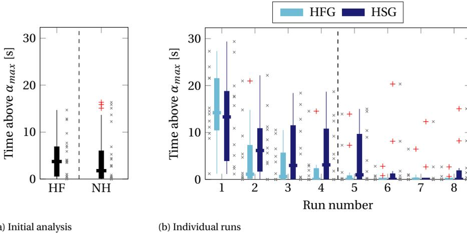
Figure 6.14: Time with angle of attack above maximum value during windshear recovery
