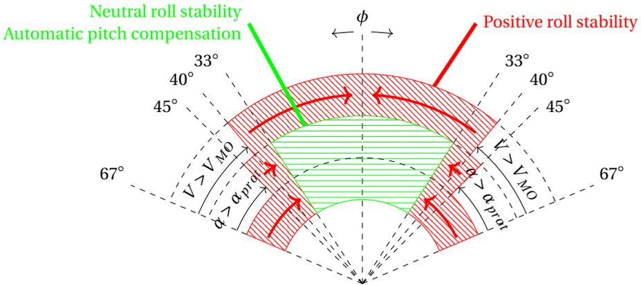
Figure 2.5: Lateral control in normal law, based on the A320 FCOM [13]
