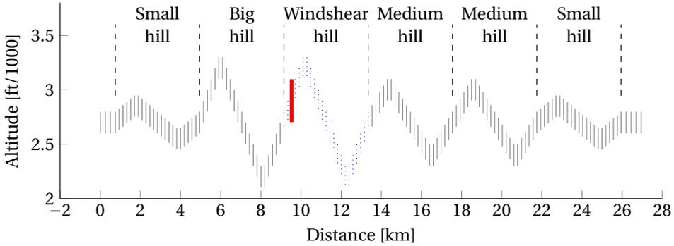
Figure 6.6: Flight path side-view, solid black vertical lines indicate “fly-through gates” shown on the outside visual; the thick red line indicates the trigger point of the windshear (not shown on the outside visual); the dotted blue lines indicate the windshear section used in our evaluation
