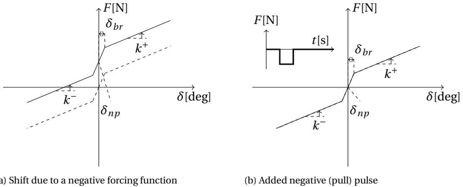
Figure 2.12: Haptic profiles showing the addition of a forcing function
