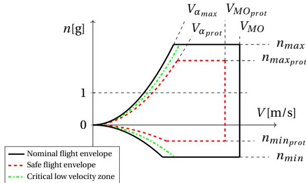
Figure 6.1: Flight envelope, velocity ( $V$ ) versus load factor ( $n$ )
