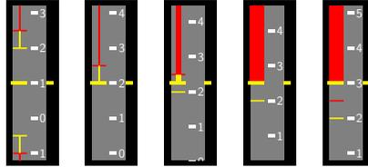
Figure 4.5: Load factor indicator progressively reaching and eventually exceeding the upper limit
