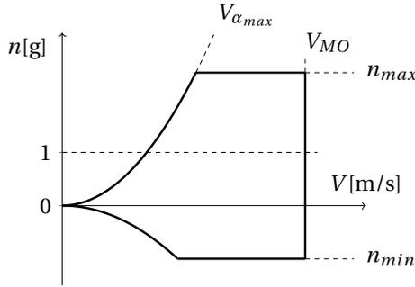
Figure 2.3: Flight envelope, allowable load factor ( $n$ ) versus allowable velocity ( $V$ )
