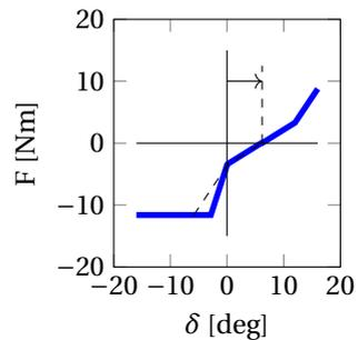
(e) Guidance design with increased stiffness (severity 0.5), Fig. 7.3c and shifted neutral point
