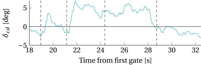
(c) Control device deflection, i.e., input from the side stick to the FCC
