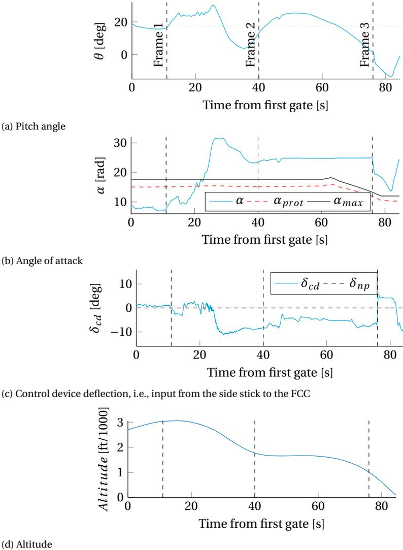
Figure 7.15: Time traces of the crash which occurred during Run 1 of Manual Participant 7
