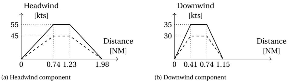
Figure 4.14: Windshear model, based on Ref. [76]; the dashed profile was used in the training runs
