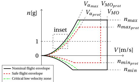
Figure 2.9: Flight envelope, load factor ( $n$ ) versus velocity ( $V$ ), inset for Fig. 2.11
