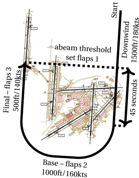
Figure 7.10: Traffic pattern flow to runway 36L at Schiphol (Schiphol layout from AIP [84])
