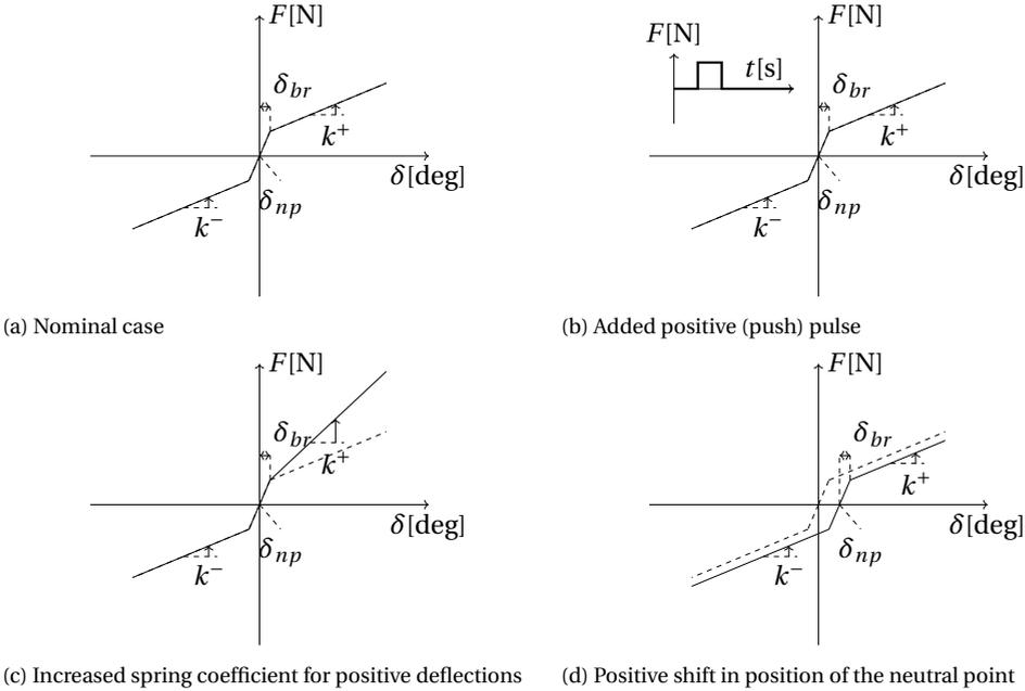
Figure 3.3: Control device profiles
