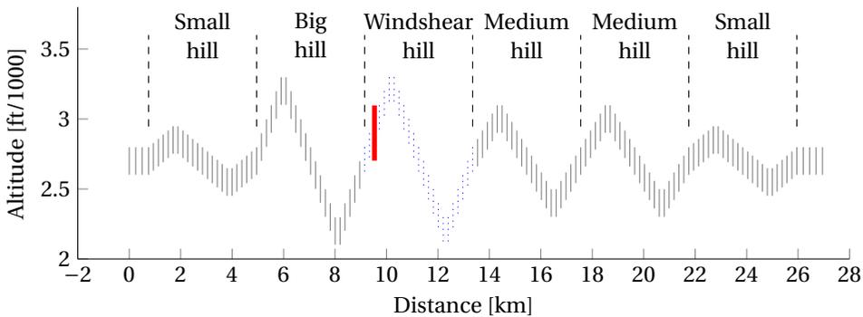
Figure 7.7: Flight path side-view, solid black vertical lines indicate “fly-through gates” shown on the outside visual; the thick red line indicates the trigger point of the windshear (not shown on the outside visual); the dotted blue lines indicate the windshear section used in our evaluation
