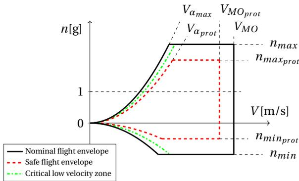
Figure 7.1: Flight envelope, velocity ( $V$ ) versus load factor ( $n$ )
