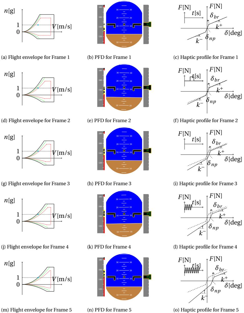
Figure 2.18: Flight envelopes, PFDs, and haptic profiles for an icing event illustrating shrinking of the flight envelope
