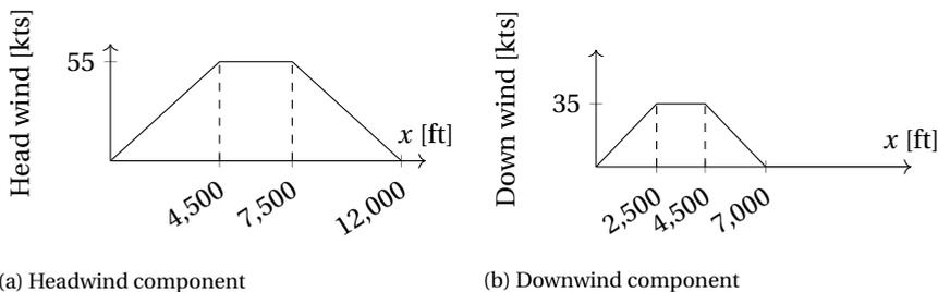
Figure 7.9: Windshear component distribution
