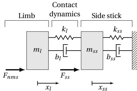
Figure 5.2: Schematic representation of the lumped limb and stick dynamics
