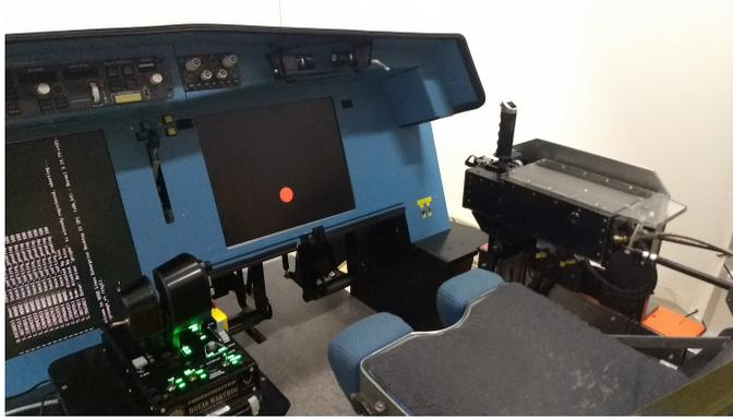
Figure 5.4: Simulator inside view showing the throttle quadrant (left), screen (front), and side stick (right)
