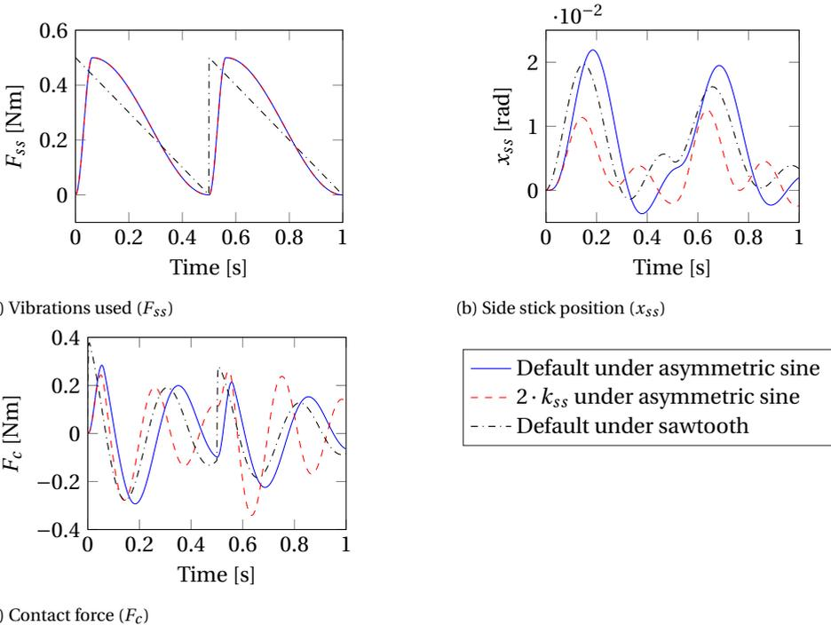
Figure 5.3: System responses to an asymmetric input
