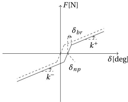
Figure 2.10: Haptic profile with a positive shift in the neutral point position
