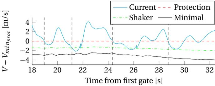
(a) Velocity relative to the minimal protection velocity
