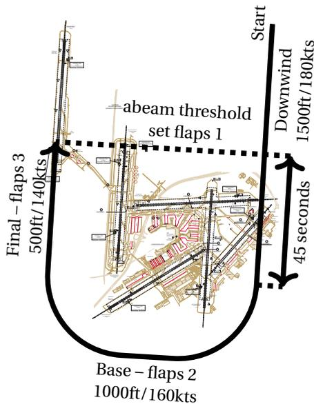
Figure 3.7: Traffic pattern flown to runway 36L at Schiphol (Schiphol layout from AIP [84])
