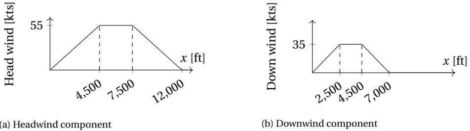
Figure 6.8: Windshear component distribution
