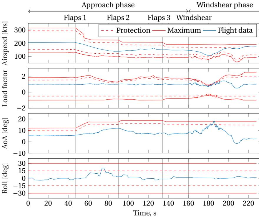
Figure 4.19: Typical flight data: Pilot A2 flying a windshear scenario at EGLL with the PFD+
