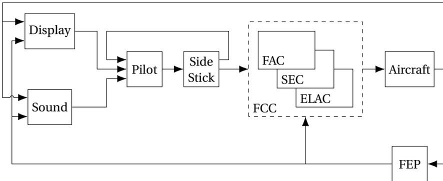
Figure 2.4: Block diagram representing the Airbus control loop
