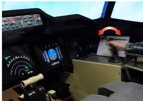
Figure 1.4: Example of haptic feedback applied to the side stick on the SIMONA flight deck at TU Delft
