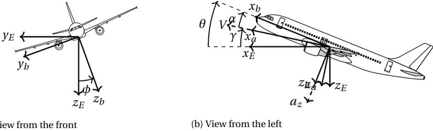
Figure 2.2: The aircraft with most important angles indicated (all positive)
