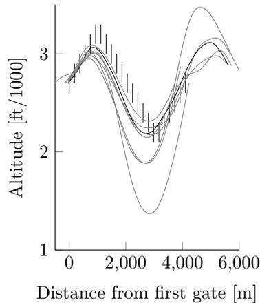
Figure 6.11: Windshear recoveries flown by Participant 23, Run 3 indicated in black, vertical lines represent gates on the outside visual
