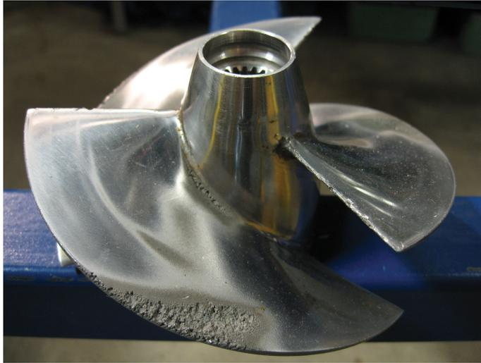
Figure 1.2: Example of blade damage caused by cavitation erosion on a boat propeller (this photograph has been obtained from the Britannica website, where it was made available by Erik Ax Dahl).
