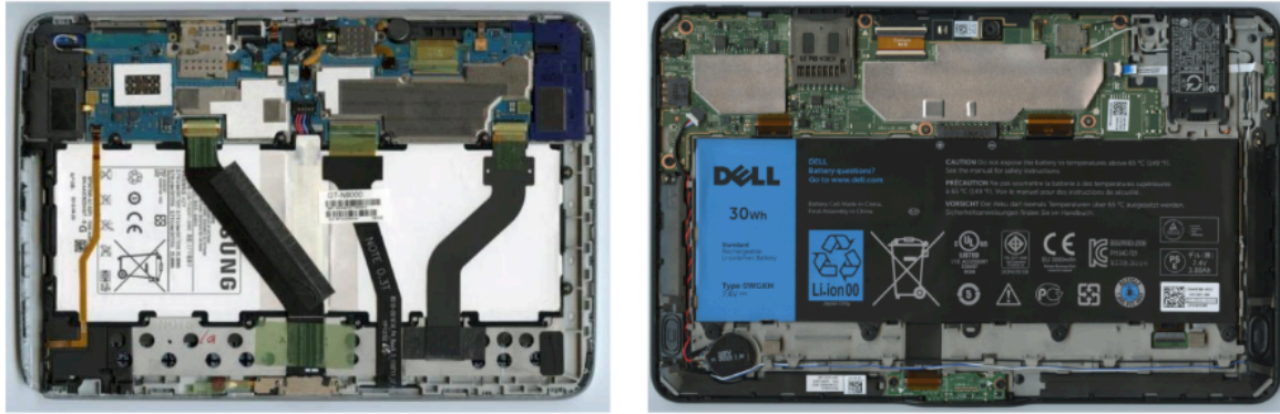
Figure 23 - Tablet distinct of connection of main components (left dry and right soldered connections) (Schischke, 2015)
