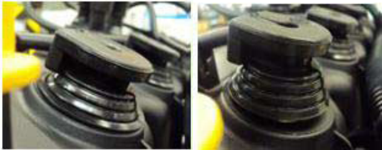
Figure 4. Spark plug fitted (left) and not fitted (right) according to method.
