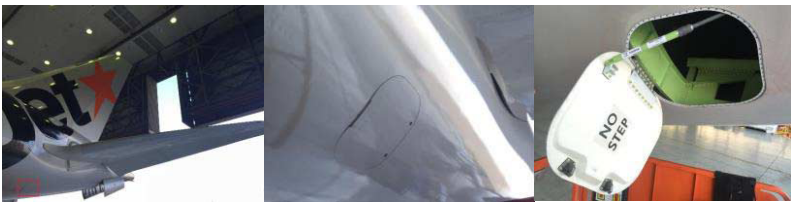
Figure 3. Location of access hatch on 787-8 aft of the rear pressure bulkhead.
