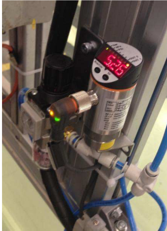
Figure 6. Pressure switch system.
