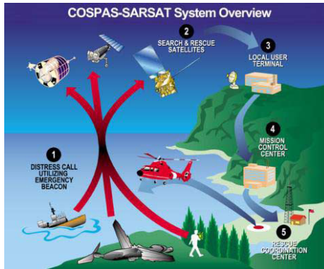
Figure 2. Overview of the operational procedure when an activated beacon uses COSPAS SARSAT [2].
