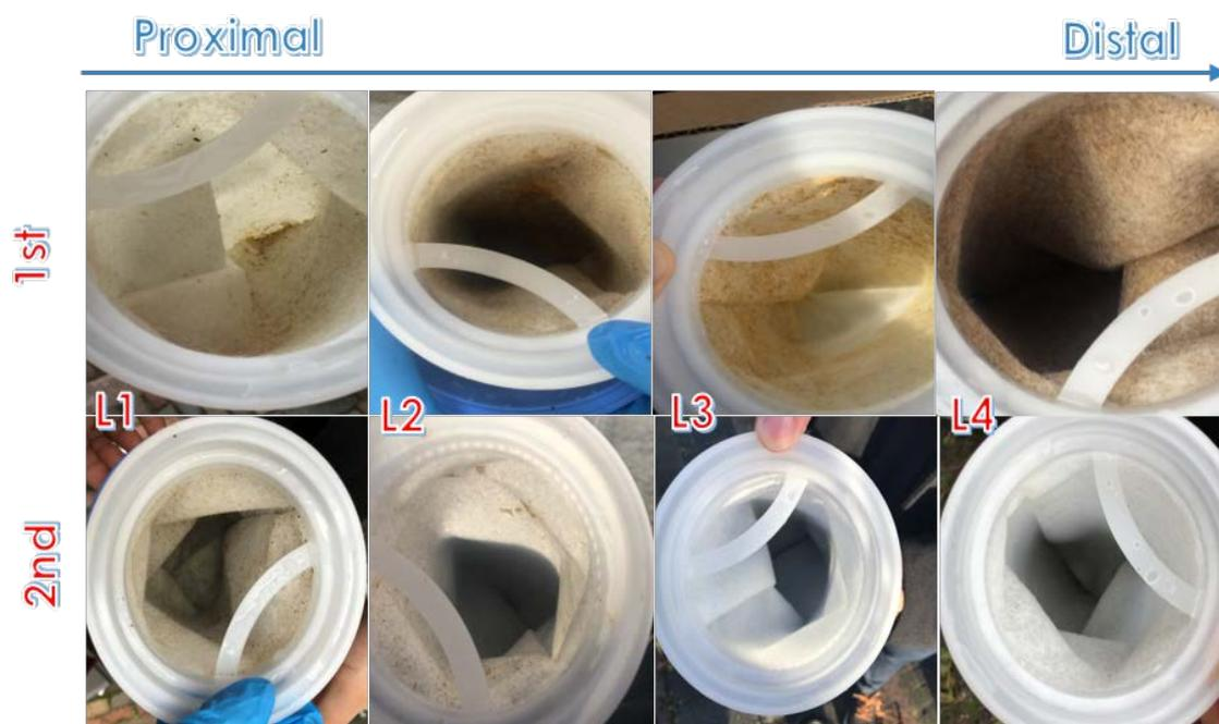
Figure 3.16 Visual observation of 1st and 2nd batch filter bags sorting in distance order from L1 to L4.
