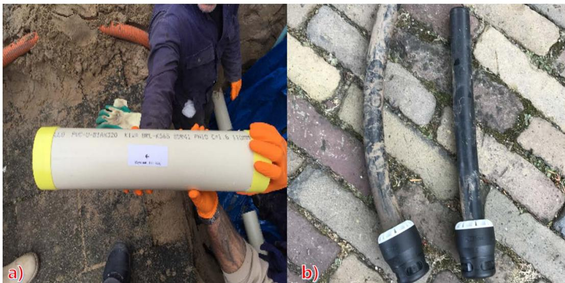
*Figure 2.5 a) Main pipe(PVC-U) sample with diameter of 110mm; b)Household connection pipes(HGPE) with a diameter of 25mm*
