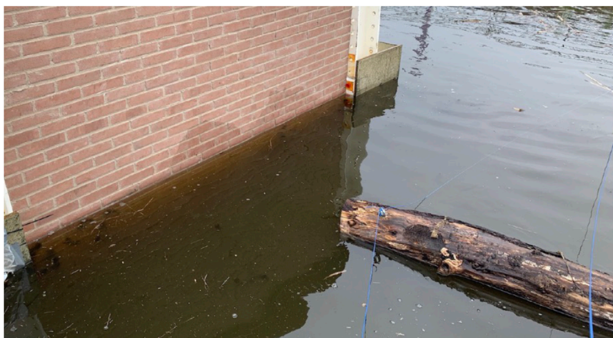
FIGURE 5 Floating tree log setup for soft debris impacts.
