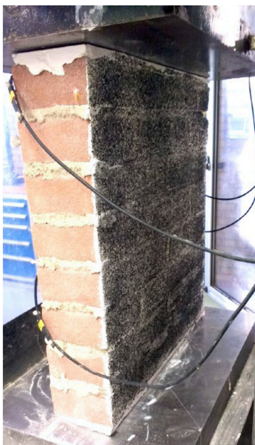
FIGURE 8 Compression wallet test in testing rig with Digital Image Correlation (DIC) black-and-white pattern.
