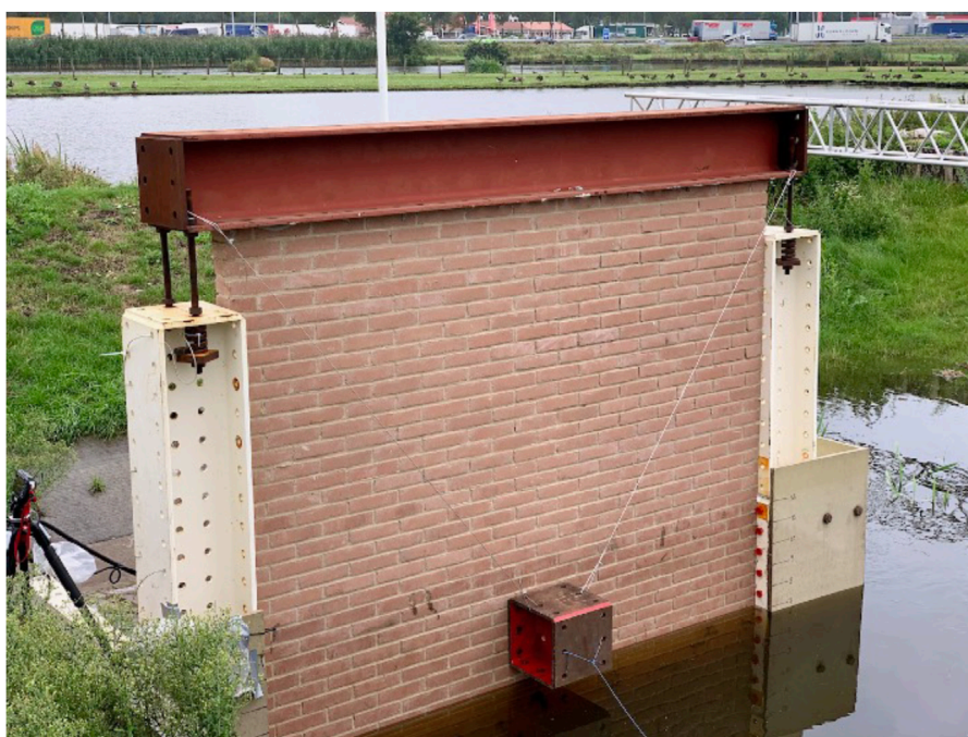
FIGURE 6 Steel cube setup for hard debris impacts.
